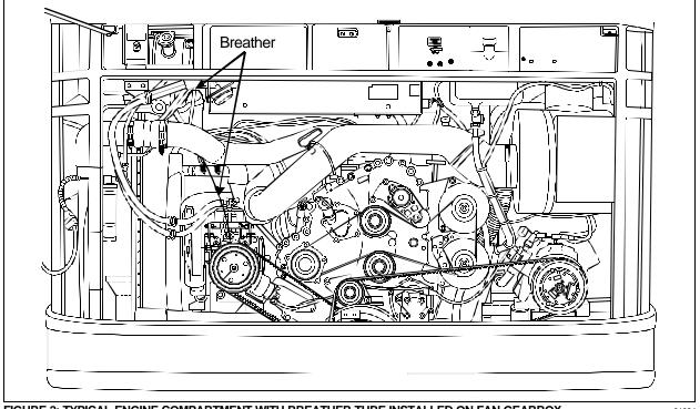
FIGURE 2: TYPICAL ENGINE COMPARTMENT WITH BREATHER TUBE INSTALLED ON FAN GEARBOX
