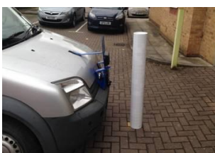
1m long pole in front of a camera mounted at 0.6m
