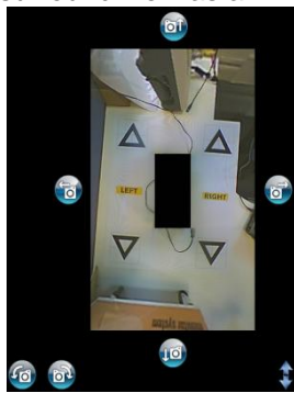
Whole surround view is out of line
