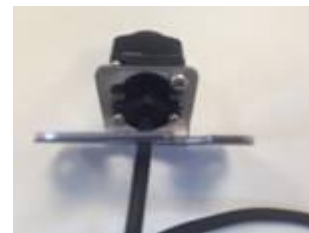
Camera rotated through 180° on its bracket (remove two larger screws rotate the camera and refit)
