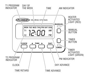
The 7 Day Digital Timer can be preset for a single start time, one day at a time or two programmed start times per day constantly activated for multiple days of the week. The clock can be preset for 12 or 24 hour time display. The heater run time duration can be preset for 1 or 3 hours. The manual button can be used to override the program and run the heater indefinitely until it is switched off.
