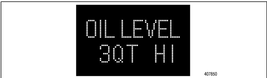
**Figure 5-4. High Fluid Level Display**
