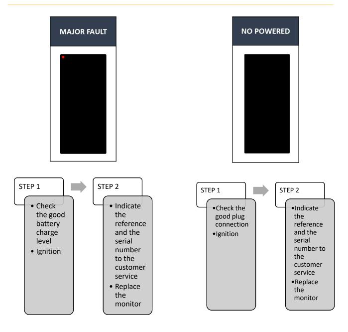
How performed an Ignition ? 1 - Shut down your vehicle 2 - Wait for 2s
