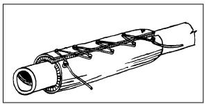
FIGURE 5: LACING WIRE INSTALLATION
