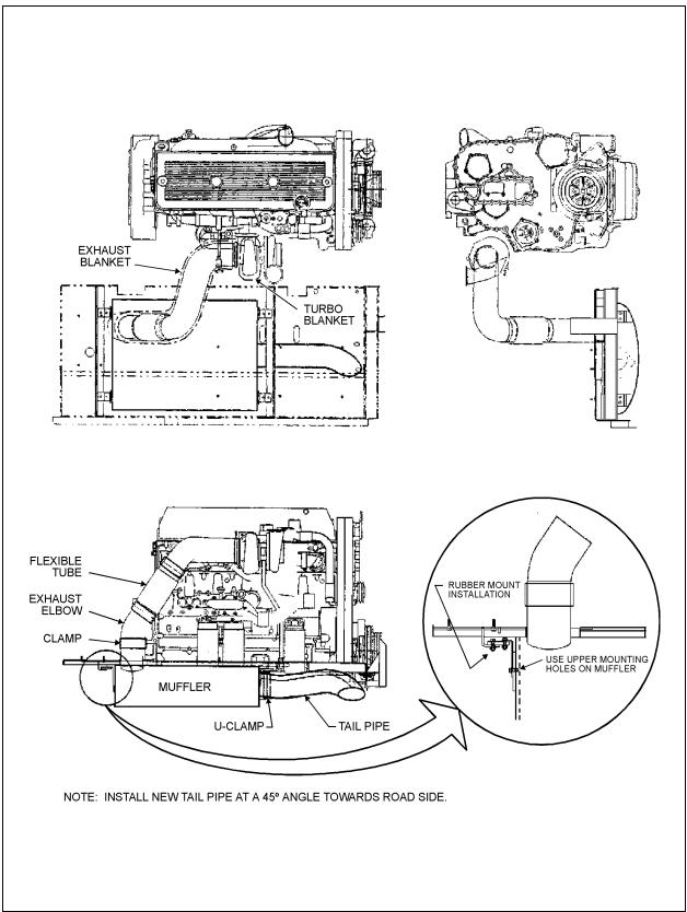
FIGURE 2: EXHAUST SYSTEM - XL-45 (COACH & SHELL) INSTALLATION
