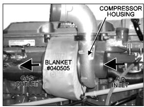
FIGURE 6: INSTALLATION OF TURBO BLANKET
