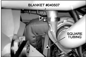
FIGURE 4: EXHAUST BLANKET INSTALLATION
