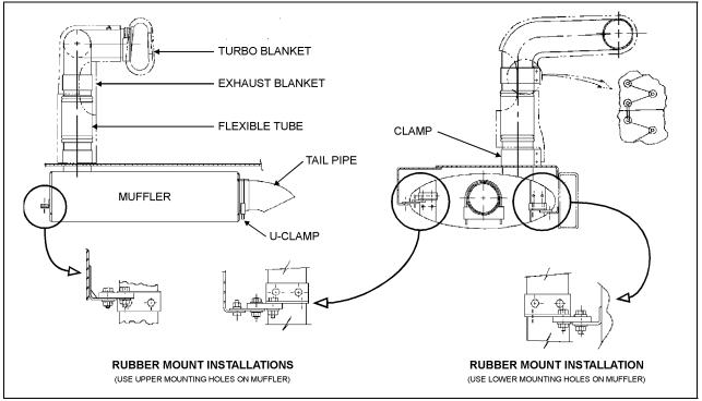
FIGURE 1: EXHAUST SYSTEM - XL-40 & 45E (COACH & SHELL) INSTALLATION
