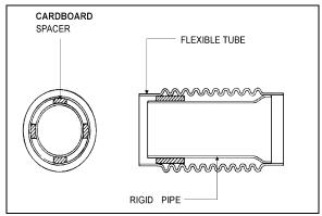
FIGURE 3: FLEXIBLE TUBE INSTALLATION
