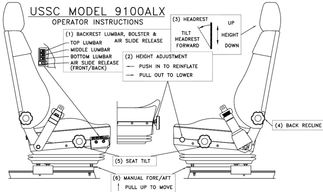
**SEAT HEIGHT:** The 91X ALX Air Suspension Seat has five (5) inches of vertical height adjustment. Seat height adjustment knob is located on the front left edge of the seat cushion. Pulling the knob out releases air pressure, this decreases height. Pushing the knob in increases the seat height.
