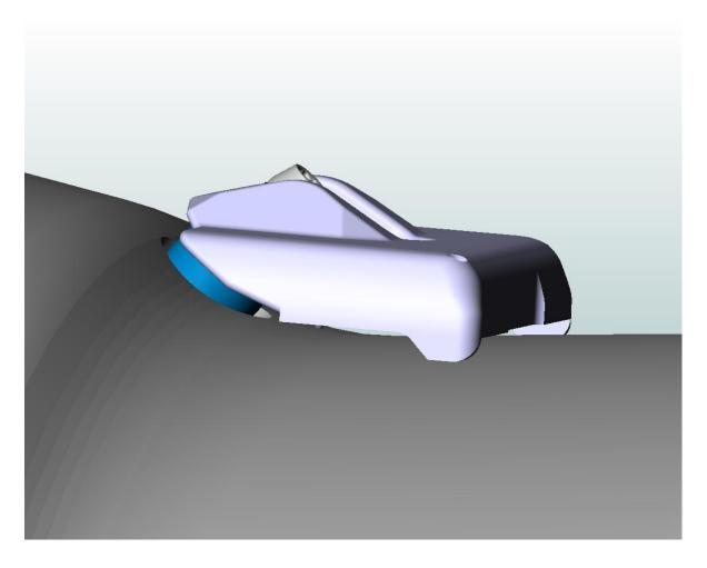
Each commercial vehicle wheel sensor is mounted to the wheel rim using a particular valve, suited to that rim. The feet of the sensors make contact with the rim creating a three point fixing.
