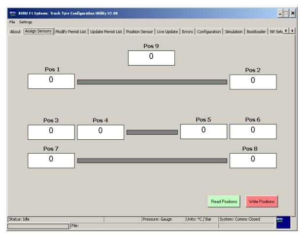
The assign sensors page is used to assign sensors to positions on the vehicle. Every sensor used on a vehicle must have its serial number programmed into the assign sensors page. This is the mechanism used to determine which sensor on the vehicle has an issue. The received sensor serial number is compared with the information entered into this page and the data allocated to a particular position.
