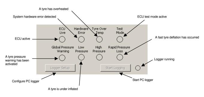
By clicking on the 'Logger Setup' the logging configuration page can be accessed.
