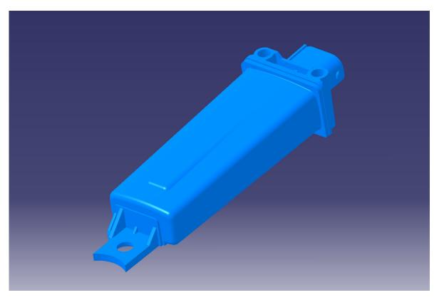
The DGA+ Antenna is used to receive the RF datagrams from the TPMS sensors and transmit the information to the TPMS ECU using a LIN bus connection.
