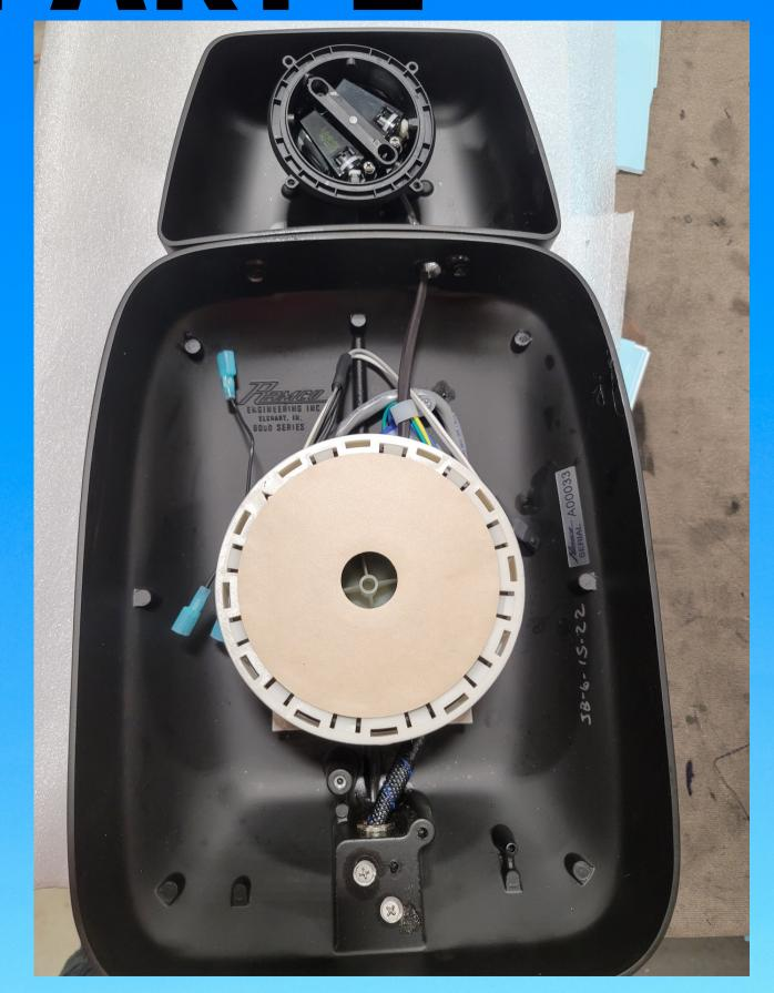
The circle by the arrow on the snap ring should line up with the hole that has the flat part on the inside. The three circles on the inside of the snap ring only work in one configuration as well, so you will not be able to improperly install it easily.
