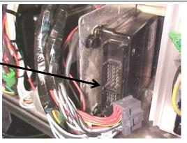
Disconnect connectors from CPC Disconnect connector from master ID Disconnect 3 connectors from CECM Disconnect connector C92
