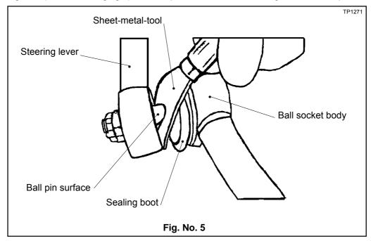
If there is corrosion of the ball pin or the sealing boot has deteriorated through ageing or is damaged, replace the ball joint in question, or the complete tie rod or drag link as appropriate.
