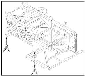
FIGURE 48: FRONT END JACKING POINTS
