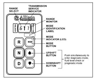
9.4 DIAGNOSTIC CODE DISPLAY AND CLEARING PROCEDURE – ALLISON 4<sup>TH</sup> GENERATION CONTROLS
