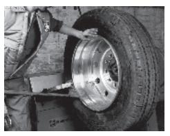
Remove the valve core from the valve stem to ensure complete deflation. Place wheel on machine and position tool so flat end can be driven between tire bead and rim flange. Straighten tool to a vertical position until bead is separated from wheel.
