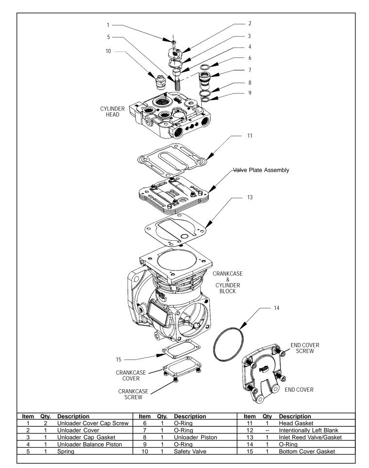
FIGURE 9- BA-921 EXPLODED VIEW OF SERVICEABLE PARTS
