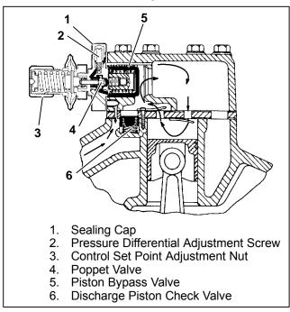
Figure 1-9. Pressure-Operated Unloader -**Unloaded Operation**
