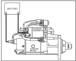
Figure 4 - TESTING PINION MOVEMENT AND PULL-IN WINDINGS (GROUND-FLOAT TYPE)
