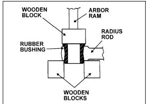
FIGURE 44: RADIUS ROD BUSHING INSTALLATION 16012
