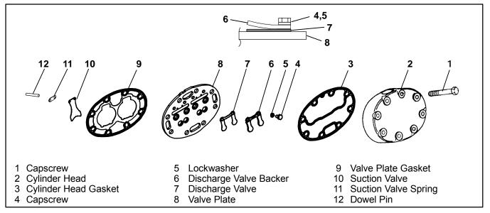
Figure 3-2. Cylinder Head & Valve Plate
