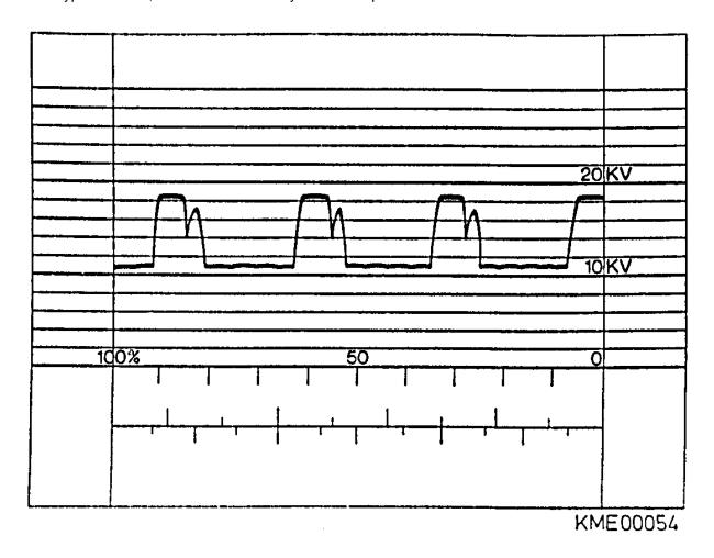
Figure 42 Open Positive Rectifier Diode
