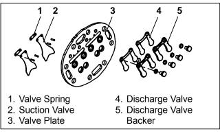
Figure 1-2. Suction & Discharge Valve
