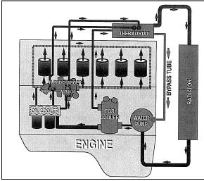
FIGURE 1: COOLANT FLOW SCHEMATIC (IMAGE DE
