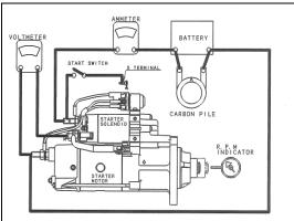
Figure 7 - NO-LOAD TEST CIRCUIT (BODY-GROUND TYPE)
