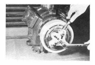
Once the rotor has been pulled from the clutch bearing mounting hub, carefully lift the rotor assembly away from the compressor, as shown.
