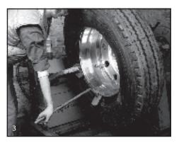
Lubricate the second tire bead. Start second bead into the well, holding it in position with the clamp to the rim flange. Lubricate bead half way around. With curved end of tool between tire bead and flange, and the stop towards the wheel, push tool outward to work tire over flange. Continue to pry bead over flange using the tool until remaining bead is over flange. Seat the tire bead using an air ring or other mechanical bead seating aid.
