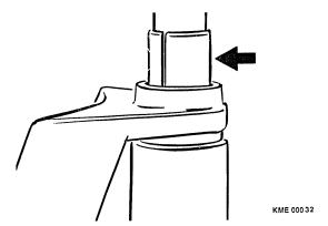
Figure 30 Sliding Bushing Installation
