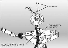
FIGURE 13: CLOCKSPRING INSTALLATION
