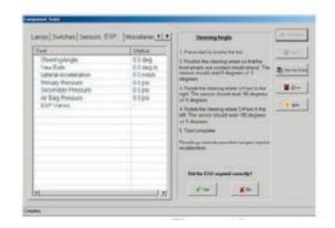
**7.** Follow the prompts to perform a test of the Steering Angle Sensor.
