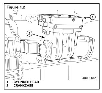
The **cylinder head** contains the inlet, discharge and unloader valving, as well as an integral relief valve. There are two water ports, marked Port 9, an air discharge port, marked Port 2, and an inlet port, marked Port 0, cast into the cylinder head to accommodate a hose connection. The cylinder head is mounted on the crankcase.
