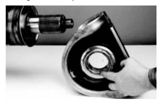
When replacing a center bearing assembly, be sure to fill the entire cavity around the bearing with a waterproof lubricant. Enough lubricant must be applied to fill the cavity to the extreme edge of the slinger surrounding the bearing. Refer to the below table.
