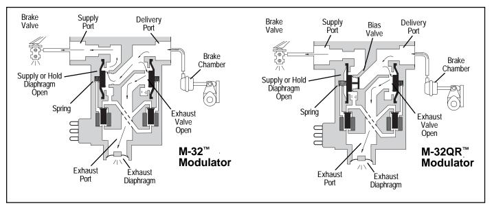
FIGURE 7: M-32™ AND M-32QR™ MODULATORS RAPID NON-ANTILOCK EXHAUST OF SERVICE BRAKES
