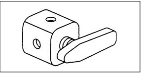
FIGURE 24: THREE-WAY VALVE
