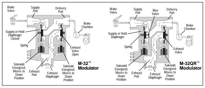
FIGURE 8: M-32™ MODULATOR ANTILOCK EXHAUST OF BRAKES
