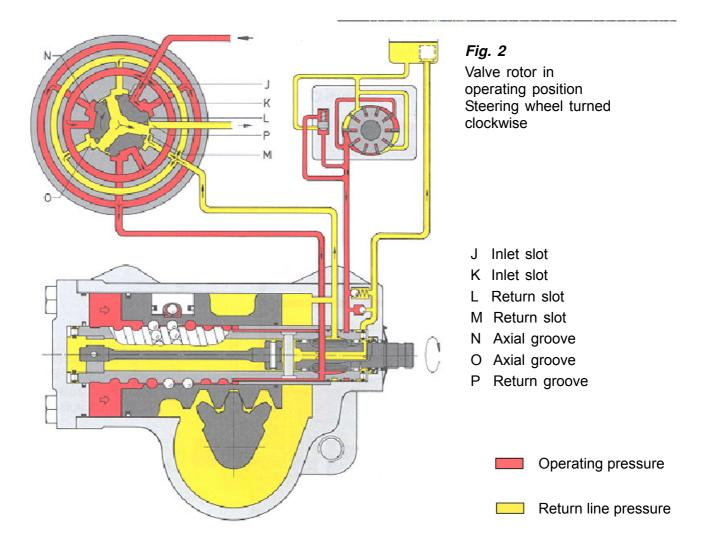
When the steering wheel is turned to the right, the piston will shift to the right (*Fig. 2*). A pressure will now build up in the left-hand cylinder chamber which is a function of the steering effort required.
