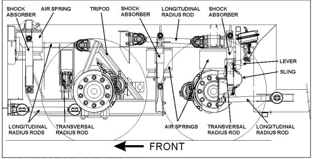
FIGURE 36: REAR SUSPENSION COMPONENTS
