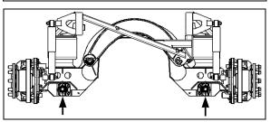
FIGURE 53: JACKING POINTS ON TAG AXLE
