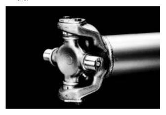
8. Move the cross laterally to the opposite side and through the cross hole, beyond the machined surface of the yoke lug. Place a bearing assembly over the cross trunnion and slide it into the cross hole, seating the plate to the face of the lug. Thread the bolts by hand or with a wrench into tapped holes in the yoke.
