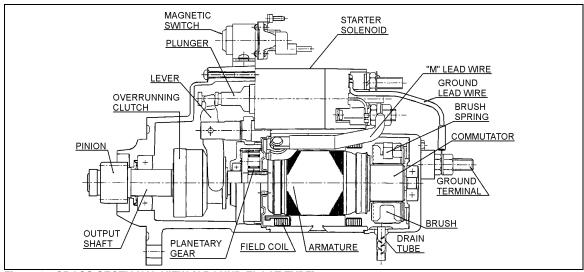
Figure 3 - CROSS-SECTIONAL VIEW (GROUND-FLOAT TYPE)
