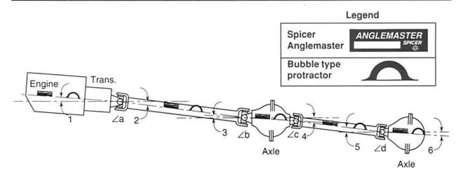
The most convenient way to determine U-joint angles in the side view is through use of a Spicer Anglemaster™ or a bubble type protractor. Procedure is as follows:
