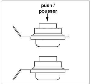
FIGURE 35: ENGINE COMPARTMENT LIGHT
