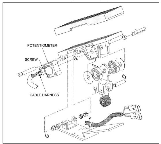
FIGURE 26: ELECTRONIC FOOT PEDAL ASSEMBLY 03035
