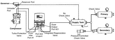
FIG. 2.C External Purge Tank Regeneration with Integrated Governor
