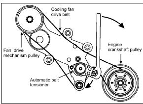
FIGURE 28: DRIVE BELT ROUTING (DDC S60 ENGINE)
