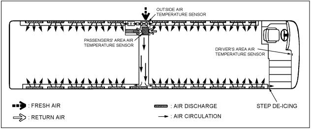
FIGURE 3: CENTRAL HVAC SYSTEM AIR CIRCULATION
