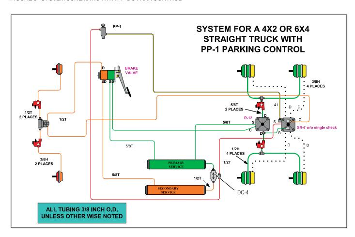
FIGURE 4 - SYSTEM SCHEMATIC WITH PP-1 PARK CONTROL AND DC-4 DOUBLE CHECK VALVE
