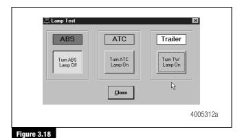
This is helpful in verifying correct operation, installation and wiring of the lamps to the ECU.
