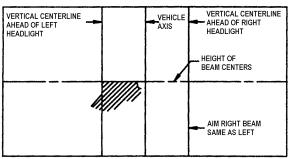
FIGURE 28: HIGH-INTENSITY ZONE (SHADED AREA) OF A PROPERLY AIMED LOWER BEAM ON THE AIMING SCREEN 7.6 M (25FT) IN FRONT OF VEHICLE 06504
