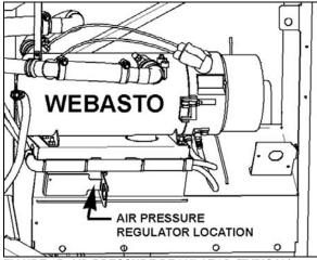
FIGURE 15: AIR PRESSURE REGULATOR (TYPICAL)07130
