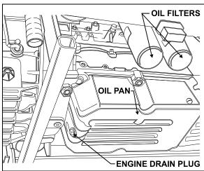
FIGURE 22: ENGINE DRAIN PLUG AND OIL FILTERS
