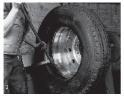
Repeat procedure at intervals until bead is totally separated from wheel. Repeat procedure on other side of tire. Tire is now ready for demounting. Lubricate the tire bead.
