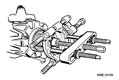
Figure 20 Inner Bearing Race Removal
