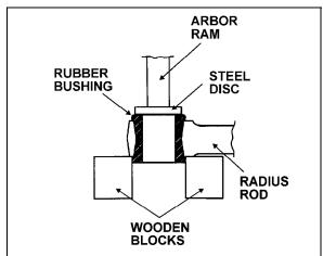
FIGURE 43: RADIUS ROD BUSHING REMOVAL
