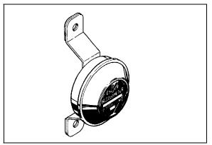
FIGURE 18: HUBODOMETER
