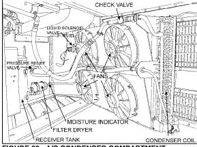
FIGURE 29: A/C CONDENSER COMPARTMENT 2
