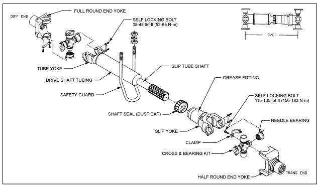
FIGURE 1: PROPELLER SHAFT ASSEMBLY
