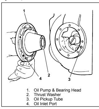
Figure 3-5. Oil Pump and Bearing Head Assembly 3.5.2 Disassembly, & Inspection
