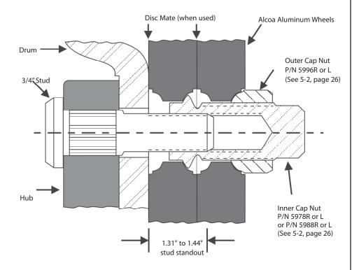
Correct mounting for dual aluminum, stud located / ball seat mount wheels.
