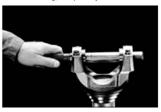
5. If, after proper cleaning, the alignment bar still does not pass through both bushings, the yoke lugs are distorted, and the yoke should be replaced.
