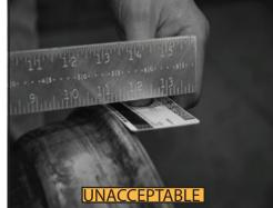
Photo above shows and undersized wheel that you can clearly place a credit card (approximately .030 in. or .76mm) between the square and the wheel.
