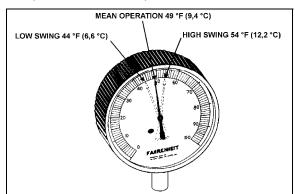
FIGURE 34: HIGH & LOW SWING TEMPERATURE AT REMOTE BULB 22047
