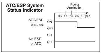
FIGURE 9 - ATC INDICATOR LIGHT START UP SEQUENCE
