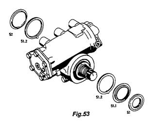
Slide the assembled dust seal (51) over the serration of sector shaft (80) by hand (the sector shaft must be kept as free of grease as possible) and press it into housing (1) until stop-ring (51.1) is flush with housing (1).
