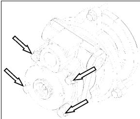
FIGURE 7: POWER STEERING PUMP REMOVAL
