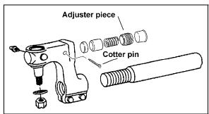
FIGURE 3: TIE ROD END PLAY ADJUSTMENT
