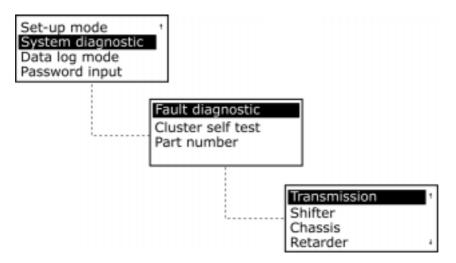
The line "Fault diagnostic" should now be highlighted, if it's not you can simply use the up/down button on the windscreen wiper handle to move to that line. Press the "Return" button again and the fault code set in the transmission ECU will now be displayed on the screen.
