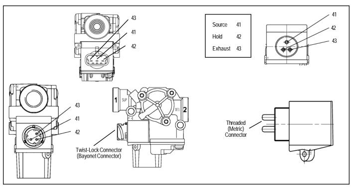
FIGURE 10: M-32™ AND M-32QR™ MODULATORS CONNECTOR VIEWS
