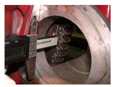
Dimension between the mounting surface and the end surface of ring gear
