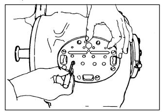
Figure 3-4. Checking Suction Valve
