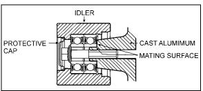
FIGURE 23: IDLER MOUNTED ON THE CAST ALUMINUM SUPPORT
