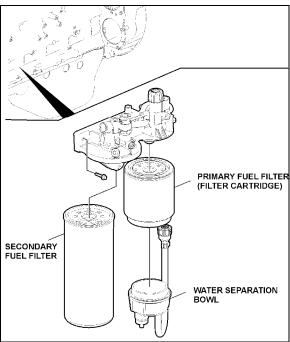
FIGURE 11: FUEL FILTERS WITH VOLVO D13 ENGINE
