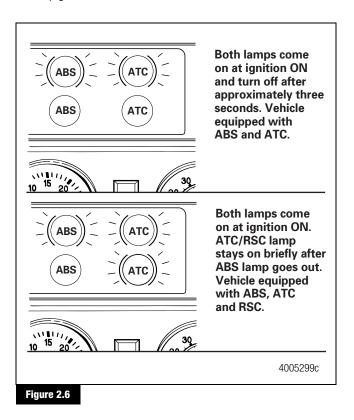
**NOTE:** Active mode means RSC is installed and will become active if it is needed.
