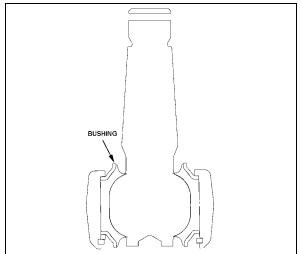
FIGURE 27: LOWER A-ARM CENTRAL BALL JOINT 16113
