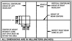
FIGURE 29: AIM INSPECTION LIMITS FOR UPPER-BEAM HEADLIGHTS 06505
