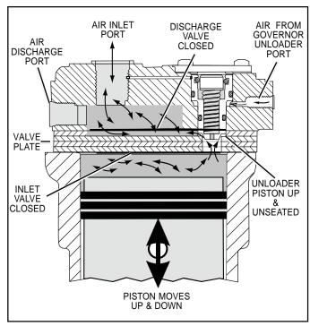
FIGURE 6 - OPERATIONAL-UNLOADED
