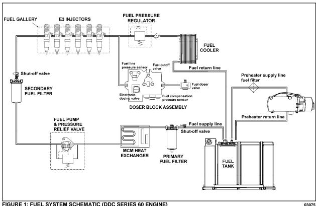
FIGURE 1: FUEL SYSTEM SCHEMATIC (DDC SERIES 60 ENGINE)
