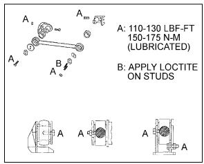
FIGURE 9: RADIUS ROD INSTALLATION
