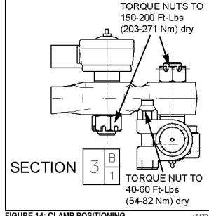
**FIGURE 14: CLAMP POSITIONING**
