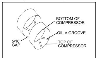
Figure 3-14. Seal End Main Bearings
