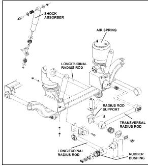
FIGURE 2: DETAILS OF FRONT SUSPENSION 16110
