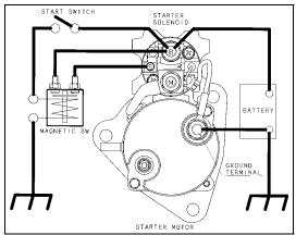
Figure 2 - BASIC STARTING CIRCUIT (GROUND-FLOAT TYPE)
