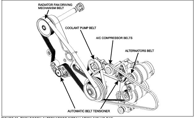
FIGURE 22: TWIN BOSCH ALTERNATORS INSTALLATION (VOLVO D13)
