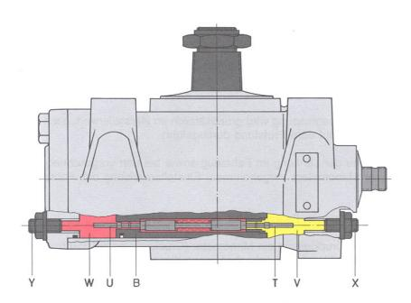
Fig. 4 Steering limiting valve closed
