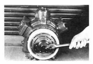
Install a flange-type gear puller into the three 5/16-18 tapped holes in the clutch rotor assembly, as shown.
