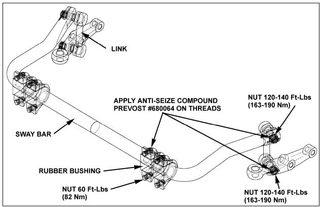
FIGURE 34: SWAY BAR (FRONT SUSPENSION)
