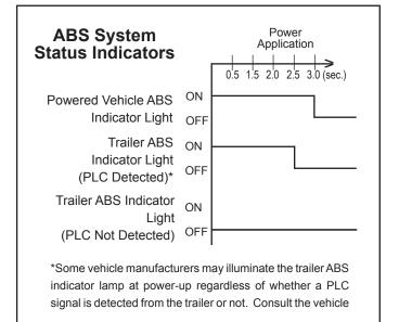
FIGURE 8 - ABS DASH LIGHTS START UP SEQUENCE
