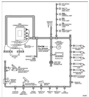
FIGURE 14: VEHICLE INTERFACE HARNESS (GENERAL APPLICATION SHOWN)
