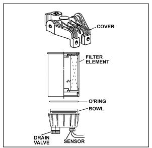
FIGURE 5: RACOR FUEL /WATER SEPARATOR
