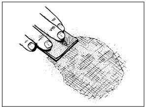
FIGURE 5: FIBERGLASS REPAIR
