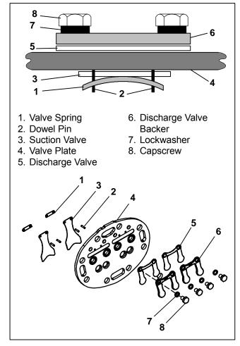
Figure 3-3. Installing Suction Valves
