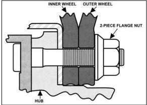
FIGURE 5: HUB-MOUNTED WHEELS
