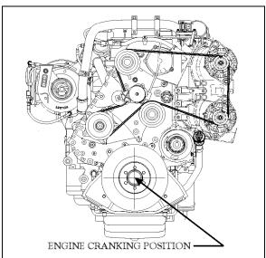
FIGURE 10: ENGINE CRANKING POSITION
