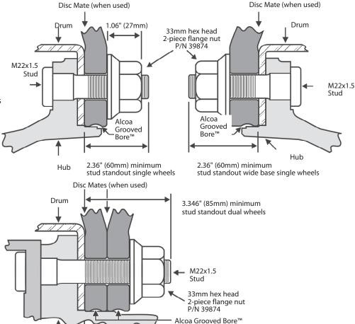
Typical assembly of single and dual wheels of hub piloted type with 33mm hex head two-piece flange nut, Part No. 39874. If hex nuts with greater overall height are used, more stud length is required.
