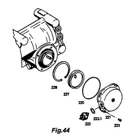
Place O-ring (220) in annular groove of housing cover (221).
