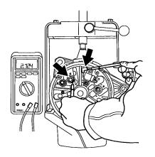
Figure 8 Testing of Suppression Capacitor
