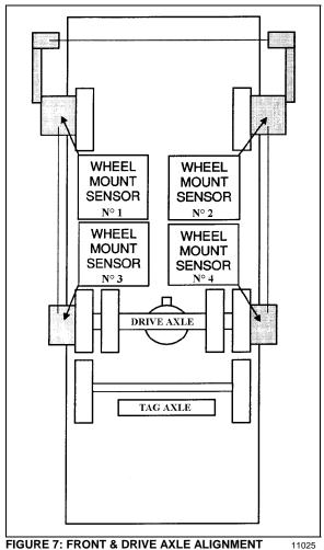
FIGURE 7: FRONT & DRIVE AXLE ALIGNMENT
