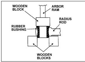
FIGURE 8: RADIUS ROD BUSHING INSTALLATION 16012
