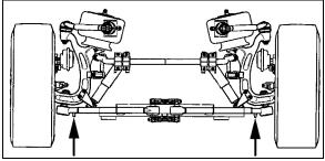
FIGURE 50: JACKING POINTS ON IND. SUSPENSION 16139
