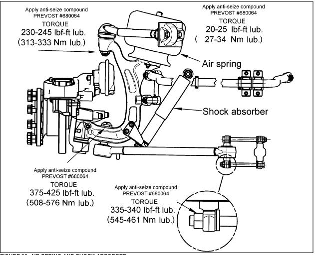
FIGURE 32: AIR SPRING AND SHOCK ABSORBER
