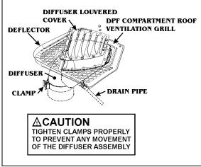
FIGURE 9: DIFFUSER ASSEMBLY
