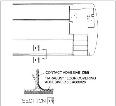
FIGURE 45: TARABUS FLOOR COVERING ADHESIVE APPLICATION
