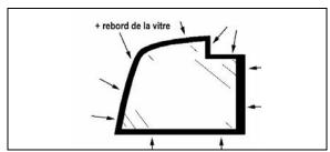
Apply masking tape onto front face before applying Sika glue to protect paint and adjacent surfaces.
