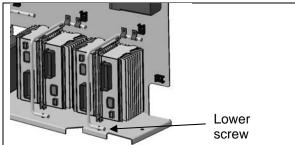
FIGURE 17: IO-B MODULE REMOVAL
