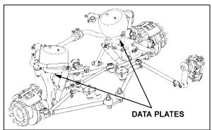
FIGURE 6: ISS TYPICAL SERIAL & MODEL NUMBERS 16136
