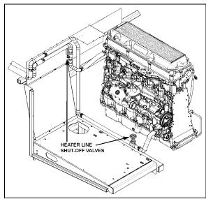
FIGURE 39: HEATER LINE SHUT-OFF VALVES
