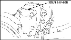
FIGURE 8 : POWER STEERING PUMP NAMEPLATE 00035
