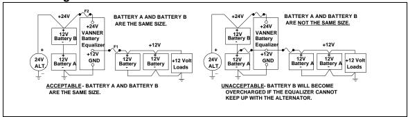
In certain applications, such as private coach or alternate energy applications, it may be desirable to have additional 12 volt "House Batteries" to operate heavy 12 volt (inverter) loads. Use the Equalizer to charge the additional batteries.
