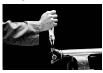
Set the yoke in the arbor press with a piece of tube stock beneath it. Position the yoke with the universal joint grease zerk (nipple) fitting pointing up to prevent interference during disassembly. Place an appropriate push rod on the upper bearing assembly, and press it through to release the lower bearing assembly.
