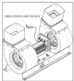
FIGURE 27: EVAPORATOR MOTOR ASSEMBLY
