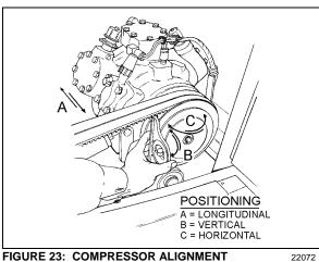
FIGURE 23: COMPRESSOR ALIGNMENT
