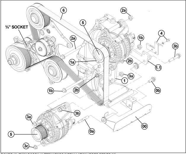
FIGURE 19: TWIN BOSCH ALTERNATORS INSTALLATION (DDEC SERIES 60)
