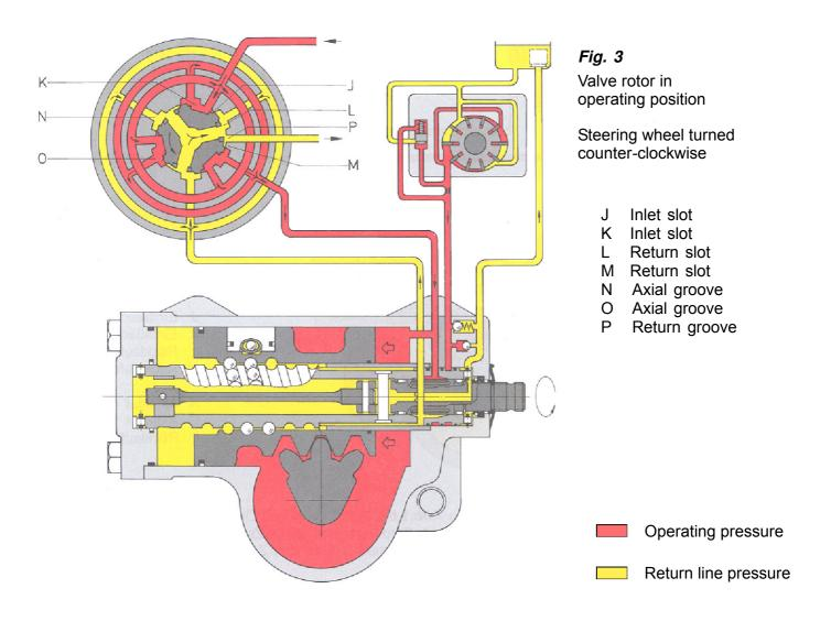
When the steering wheel is turned to the left, the piston will shift to the left (*Fig. 3*). Therefore, pressure build-up now takes place in the right-hand cylinder chamber.
