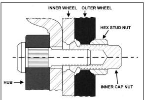
FIGURE 4: STUD-MOUNTED WHEELS
