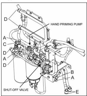
FIGURE 8: MANUAL SHUT-OFF VALVE (VOLVO D13 ENGINE) 03088
