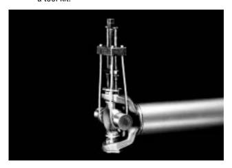
Clean the cross holes on the yoke, and inspect the cross hole surfaces for damage or raised metal. Raised metal or fretting can be removed from yoke cross holes with a fine-toothed file and/or emery cloth.
