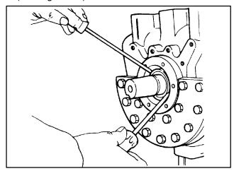
Figure 3-8. Shaft Seal Removal
