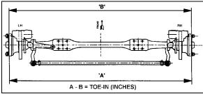
FIGURE 6: TOE-IN MEASUREMENTS
