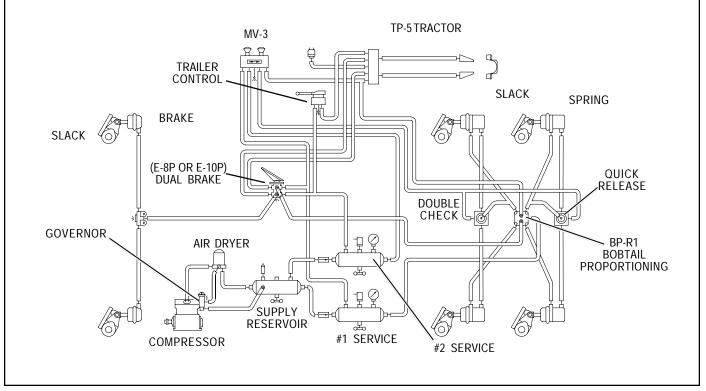
FIGURE 3 - TYPICAL PIPING SCHEMATIC
