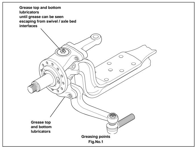
NOTE :- ALL OTHER COMPONENTS IN THE NDS RANGE OF AXLES ARE GREASED FOR LIFE AND REQUIRE NO FURTHER LUBRICATION DURING THE LIFE OF THE COMPONENT.
