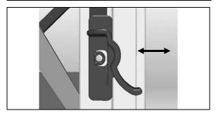
• Check handle adjustment. Handle must remain tight against its plastic housing.
