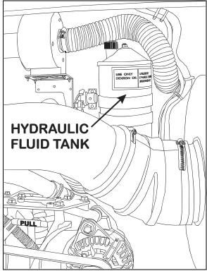
FIGURE 18: HYDRAULIC FLUID RESERVOIR LOCATION 14059
