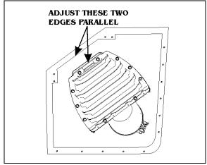
FIGURE 10: DIFFUSER POSITION ADJUSTMENT 04015\_1
