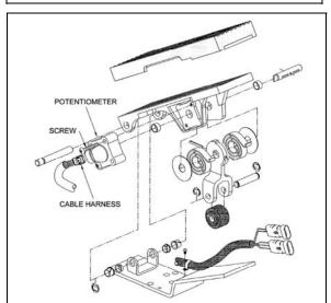
FIGURE 22: ELECTRONIC FOOT PEDAL ASSEMBLY 03035
