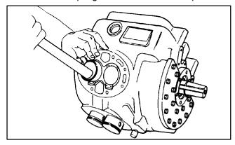
Figure 3-19. Installing Pistons
