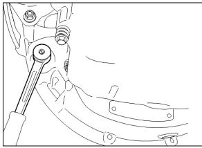
FIGURE 11: VOLVO ENGINE CRANKING POSITION
