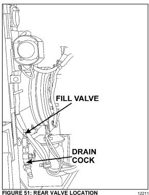
FIGURE 51: REAR VALVE LOCATION
