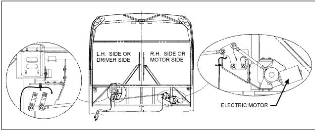
FIGURE 34: WINDSHIELD WIPER INSTALLATION
