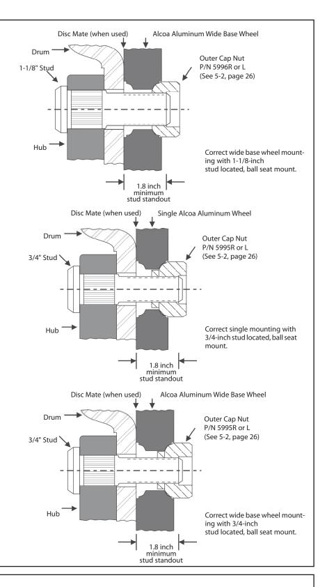
Dualed wheels, stud located, ball seat mounting
