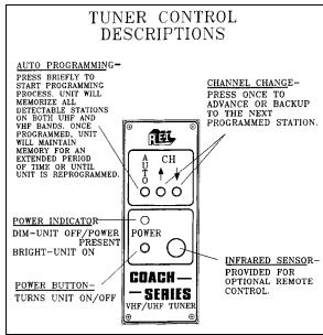
FIGURE 14: TUNER CONTROLS DESCRIPTION
