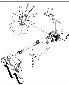
FIGURE 19: COOLING FAN DRIVE MECHANISM
