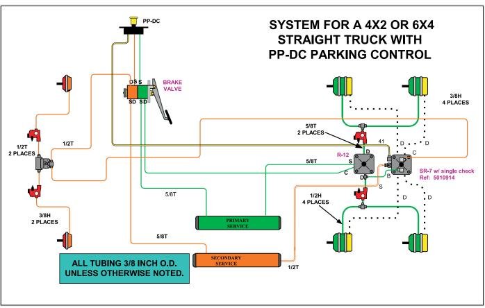
FIGURE 3 - SYSTEM SCHEMATIC WITH PP-DC PARK CONTROL
