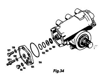
Place O-ring (122) in the inner radial groove in cylinder cover (125) and lay sealing ring (123) on top of it.
