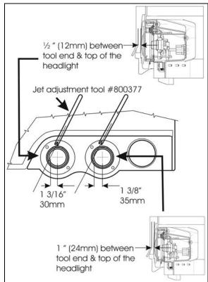
FIGURE 31: WASHER NOZZLES ADJUSTMENT
