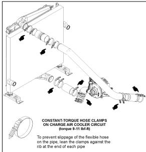
FIGURE 9: CHARGE AIR COOLER HOSE CLAMPS (DDC S60) 05134
