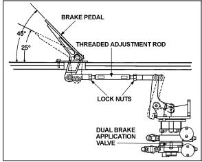
FIGURE 14: BRAKE PEDAL ADJUSTMENT
