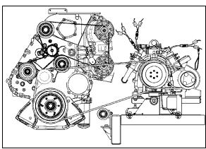
FIGURE 19: BELTS ARRANGEMENT (DDC S60 ENGINE)
