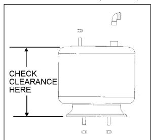
FIGURE 46: TYPICAL AIR SPRING CLEARANCE
