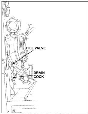
FIGURE 3: REAR VALVE LOCATION (TYPICAL)
