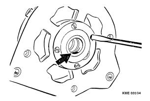
Figure 19 Drive End Bearing Removal
