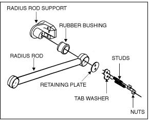
FIGURE 6: TYPICAL RADIUS ROD SETUP
