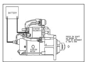
Figure 8 - CHECKING OUTPUT SHAFT CLEARANCE (GROUND-FLOAT TYPE)
