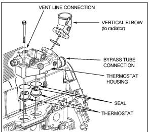
FIGURE 11: THERMOSTAT HOUSING (DDC S60 ENGINE)
