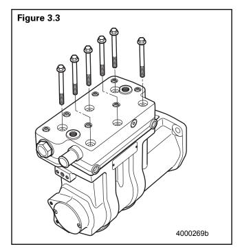
Use a mild cleaning solvent to clean the top of the crankcase.
