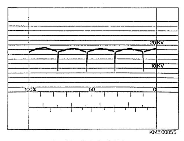
Figure 43 Open Negative Rectifier Diode
