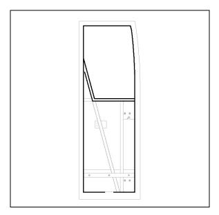
Apply Sika 255 onto door frame structure.
