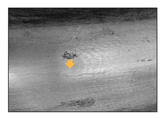
Bead seat cracks are normally caused by overloading of the wheels. If you have this type of wheel breakage it would be recommended to use SEVERE SERVICE WHEELS.
