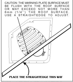
FIGURE 11: DIFFUSER POSITION ADJUSTMENT 04015\_2
