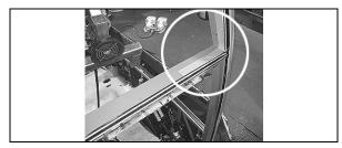
• Apply masking tape onto window.
