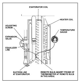
FIGURE 33: SUPERHEAT ADJUSTMENT INSTALLATION22046
