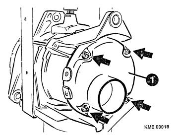
Figure 5 Air Intake Cover Removal (1)
