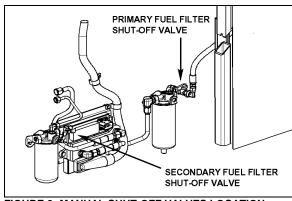
FIGURE 2: MANUAL SHUT-OFF VALVES LOCATION (DDC S60 ENGINE)
