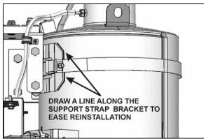
FIGURE 5: MARKING THE SUPPORT STRAP BRACKET
