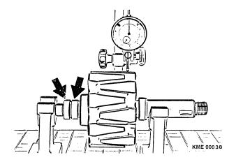
**Figure 23 Rotor Concentricity Measurement**
