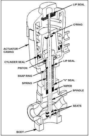
FIGURE 44: PNEUMATIC WATER VALVE
