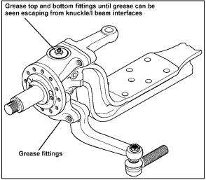
FIGURE 2: FRONT AXLE GREASING POINTS
