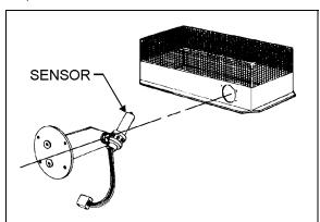
FIGURE 6: THERMISTOR SENSOR
