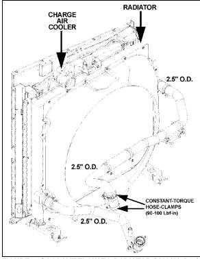
FIGURE 7: COOLANT FLOW TO RADIATOR (VOLVO D13)
