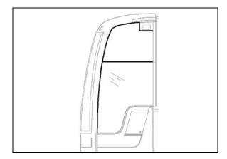
From vehicle's interior, apply some Sika 255 and make 2 finishing joints. Smooth down the joints and remove masking tape.
