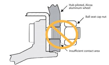
Incorrect use of ball seat cap nut on hub piloted system. Do not use ball seat cap nuts with hub piloted wheels.
