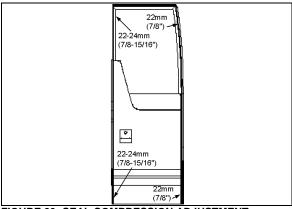
FIGURE 23: SEAL COMPRESSION ADJUSTMENT
