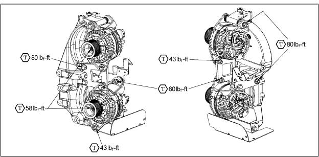
FIGURE 20: ALTERNATORS AND ACCESSORIES MOUNTING TORQUES (DDEC SERIES 60)
