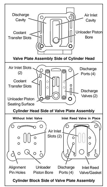
FIGURE 7 - CYLINDER HEAD AND VALVE PLATE ASSY.
