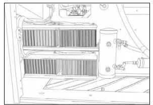
FIGURE 8: LOCATION OF BATTERIES IN CONDENSER **COMPARTMENT**
