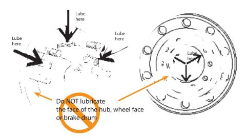
Before installing two-piece flange nuts, lightly lubricate the stud threads and the contact surfaces between the cap nut and the washer as illustrated below with an SAE 30W oil. This will minimize corrosion between the mating surfaces. Lubrication is not necessary with new hardware.
