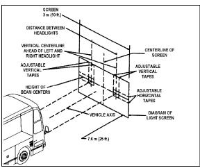
FIGURE 26: ALIGNMENT OF HEADLIGHT AIMING SCREEN 06502
