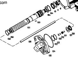
Pull reaction piston (131) out of pipe (130).
