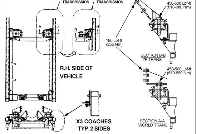
FIGURE 9: ZF OR ALLISON TRANSMISSION BRACKETS
