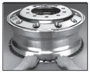
Measure the circumference of the bead seat on the open side (see illustration to left) with a ball tape.
