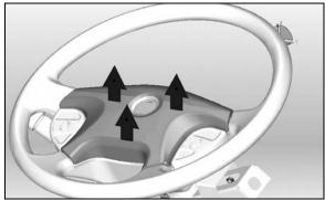
FIGURE 10: REMOVING THE HORN PAD
