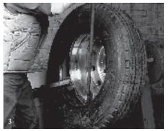
Insert curved end of tire tools between tire and wheel, approximately 10 inches apart. Pull one tool toward center of wheel, then pull second tool in the same manner. To free bead, leave one tool in position, take out and reinsert the other tool, curved end between bead and flange, a short distance from the spanned area. Pry bead free of rim, repeating process until entire bead is free from wheel.
