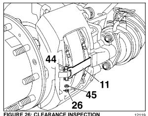
FIGURE 26: CLEARANCE INSPECTION
