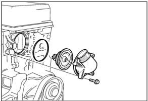
FIGURE 12: THERMOSTAT HOUSING (VOLVO D13 ENGINE)
