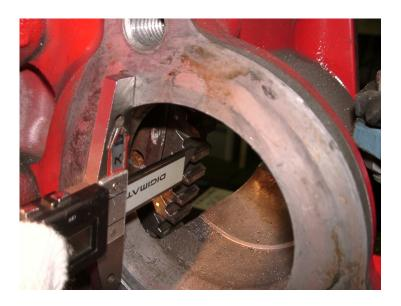
Dimension between the mounting surface and the damage depth portion of ring gear
