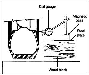
FIGURE 3: DIAL GAUGE INSTALLATION
