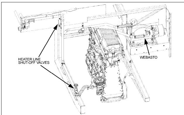
FIGURE 14: LOCATION OF HEATER LINE SHUT-OFF VALVES IN ENGINE COMPARTMENT
