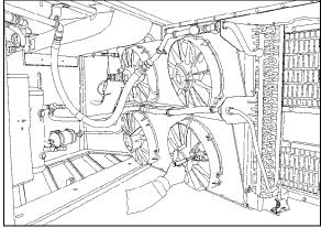
FIGURE 11: CONDENSER COIL CLEANING
