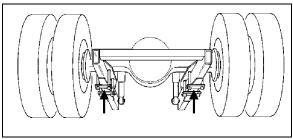
FIGURE 6: JACKING POINTS ON DRIVE AXLE
