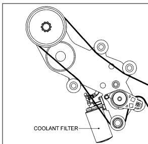
FIGURE 16: COOLANT FILTER (DDC S60 ENGINE) 05138
