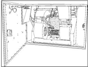
FIGURE 7: EVAPORATOR COMPARTMENT
