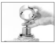
Remove cam ring, locate dots
