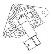
**Figure 7 Brush Length Measurement**
