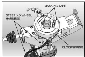
FIGURE 12: LOCKING THE CLOCKSPRING IN PLACE
