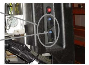
Push the blue button in to open the circuit
