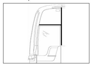
Apply anti-silicone onto molding.
