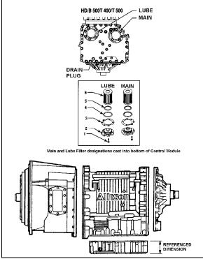
FIGURE 7: DRAIN PLUG AND FILTERS
