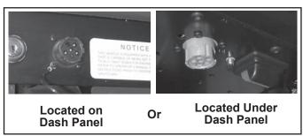
FIGURE 13 - TYPICAL VEHICLE DIAGNOSTIC CONNECTOR LOCATIONS (J1708/J1587, J1939)
