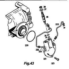
Install pipes (225 and 226) with new O-rings (224).
