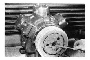
12. Secure armature assembly to crankshaft with the 3/8 special flat washer, lock washer, and 3/8-24 x 1-1/4" lg. capscrew removed in Step 1 of Clutch Removal. Torque capscrew to 16-20 ft-lb using CTD tool P/N 07-00240-01 to prevent crank shaft rotation.
