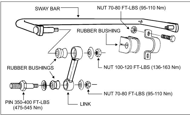
FIGURE 35: SWAY BAR (REAR SUSPENSION)
