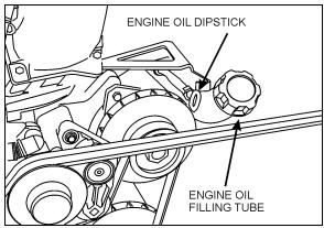
FIGURE 7: ENGINE OIL FILLING TUBE
