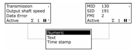
As in the example above, you can see that the fault code is set in MID 130, the SID number is 191 and the FMI number is 2. By looking at the fault code table for MID 130 (which represents the TECU) you can see that SID number 191 means "Output speed level error" as well as the displaytext shown if your dipsplay would have been set to show faults in text mode.
