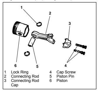
Figure 3-13. Connecting Rod, Piston, and Pin
