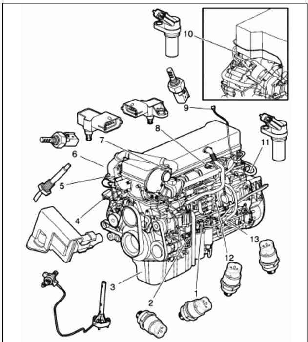
FIGURE 1: ENGINE SENSORS LOCATION
