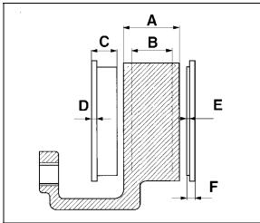
FIGURE 34: ROTOR AND PAD WEAR LIMITS
