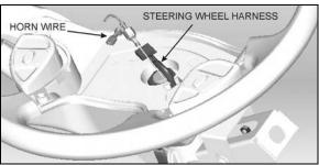
FIGURE 11: STEERING HARNESS & HORN WIRE
