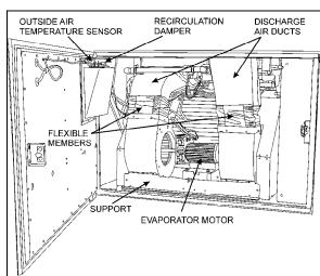
FIGURE 25: EVAPORATOR COMPARTMENT
