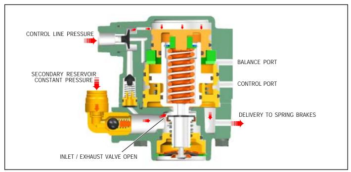
FIGURE 5 - CHARGING LESS THAN 107 PSI
