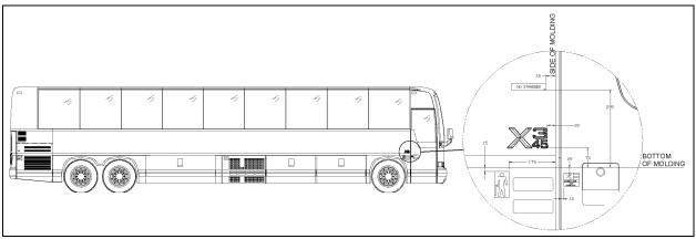
FIGURE 41: SIDE CREST POSITIONING
