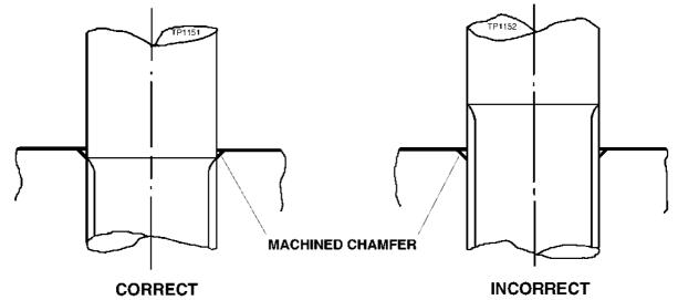
IMPORTANT:- THIS STUD FITTING PROCEDURE IS TO BE USED IN LIEU OF STATED TORQUE VALUES ON EXISTING ARRANGEMENTS.
