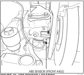
FIGURE 46: ABS SENSOR LOCATION
