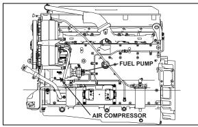
FIGURE 9: AIR COMPRESSOR LOCATION
