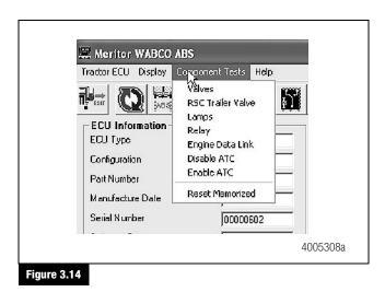
**NOTE:** Components for test may also be selected from the icons on the Tractor ABS Main Screen.
