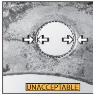
For hub piloted - normally if you see a wallowed out bolt hole, this would indicate the wheel ran loose.
