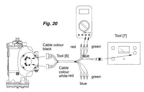
Rotate the potentiometer (232) together with the cover (221) until the Multimeter measuring instrument reads half the voltage applied, namely 2.5 V + 0.03 V.
