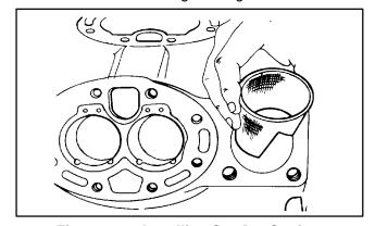
Figure 3-20. Installing Suction Strainer
