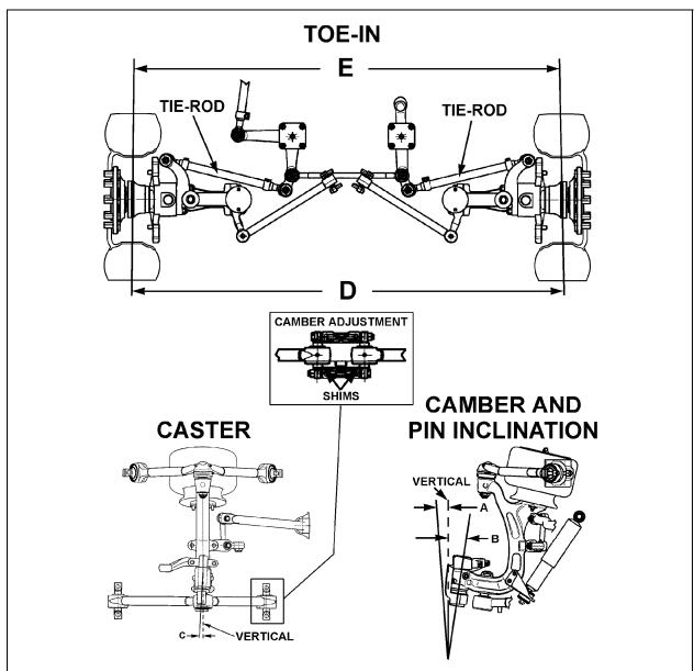
FIGURE 30: FRONT END ALIGNMENT DIAGRAM
