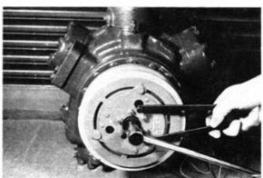
Remove the clutch armature assembly from the compressor crankshaft as a complete assembly, as shown.
