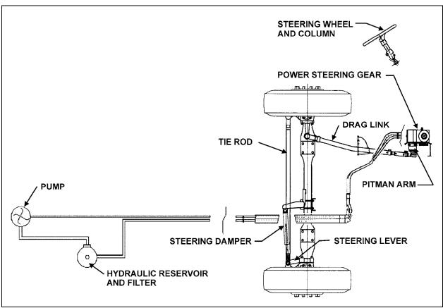
FIGURE 1: I-BEAM AXLE STEERING SYSTEM SETUP
