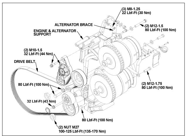
FIGURE 21: BOSCH ALTERNATORS MOUNTING TORQUES (VOLVO D13)
