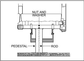
FIGURE 44: SEAT PEDESTAL ASSEMBLY
