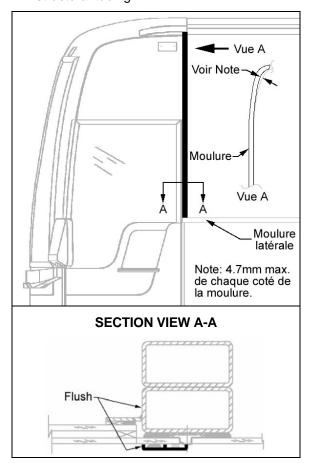
Position and fix horizontal molding (gutter).
