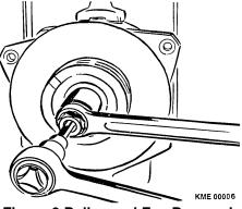
Figure 9 Pulley and Fan Removal
