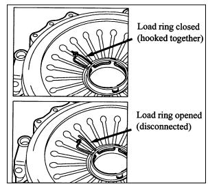
FIGURE 8: RELEASE BEARING RETAINING CLIP 0711
