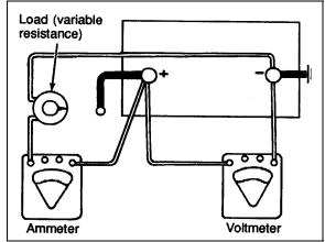
FIGURE 13: LOAD TEST
