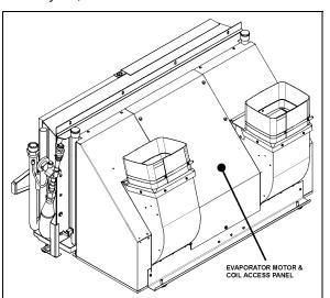
FIGURE 9: EVAPORATOR MOTOR & COIL ACCESS
