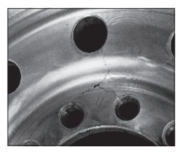
Shown below are stud hole cracks emanating from bolt hole to bolt hole. Causes are: undersized diameter of wheel support surface (see specifications on next page), support surface not flat, incorrect attachment parts (see Section 5-2) and insufficient torque (see Sections 5-8, 5-11, 6-2). Remove wheel from service.
