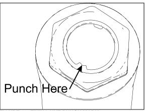
FIGURE 16: FIXING NUT PUNCH MARK
