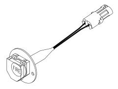
FIGURE 6 – MANUAL ACTIVATION SWITCH (DEPICTED WITHOUT TAMPER SEAL)
