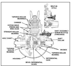
FIGURE 3: DRIVER-CONTROLLED DIFFERENTIAL LOCK
