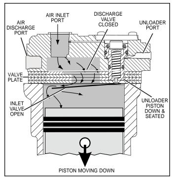
FIGURE 4 - OPERATIONAL-LOADED (INTAKE)
