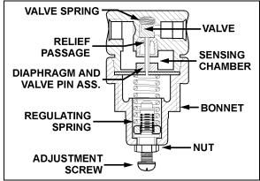
FIGURE 7: AIR PRESSURE REGULATING VALVE 12141B
