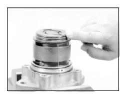
Grease o-ring and back-up ring
