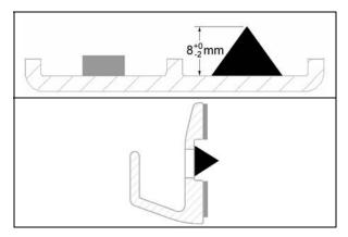
Position and fix vertical molding. Lean vertical molding against lateral molding. Make sure vertical molding lines up with structural tubing.
