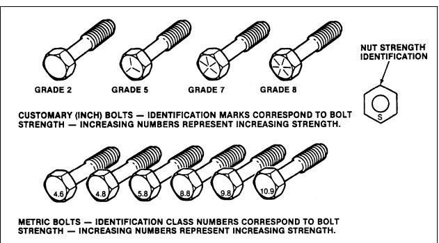
FIGURE 14: BOLT STRENGTH MARKINGS
