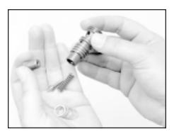
Remove spool assembly components
