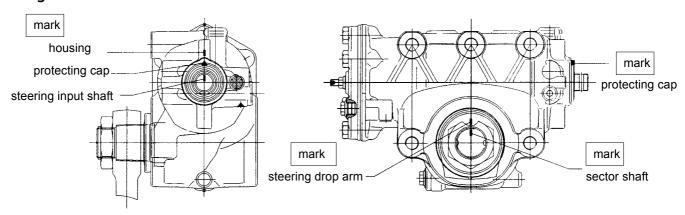
2.4 Place the steering gear into the mounting bracket and fasten it with screws.
