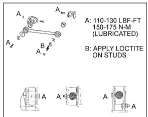
FIGURE 45: RADIUS ROD INSTALLATION
