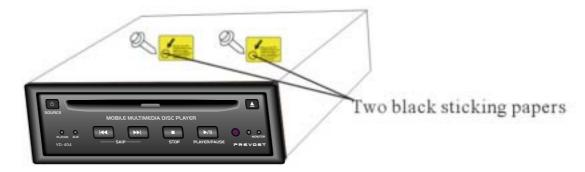
There are 2 mounting screws on the case of the DVD player( as above figure shows) to protect the unit during shipping.
