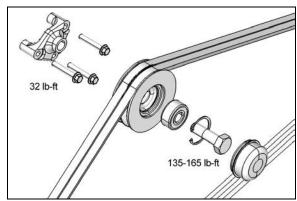
FIGURE 21: IDLER PULLEY INSTALLATION ON VOLVO **D13 ENGINE**
