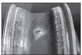
Bead seat and valve stem corrosion often are caused by entrapped moisture. Mild corrosion should be removed thoroughly by wire brush and the rim protected with non-water-based tire lubricant (see Section 4-1). Remove any severely corroded wheel from service.
