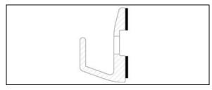
Apply Sika 252 inside the moldings onto the whole length.
