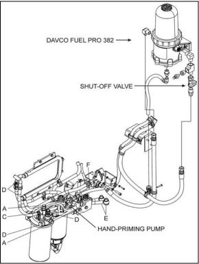
FIGURE 9: MANUAL SHUT-OFF VALVE LOCATION WITH DAVCO FUEL PRO 382 (VOLVO D13 ENGINE) 03087
