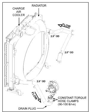
FIGURE 6: COOLANT FLOW TO RADIATOR (DDC S60)
