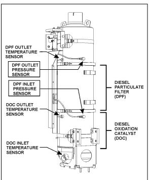
FIGURE 3: AFTERTREATMENT DEVICE (ATD USED WITH DDC S60 ENGINE SHOWN, ATD USED WITH VOLVO D13 ENGINE IS SLIGHTLY DIFFERENT) 04016
