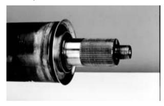
12. If no damage is apparent, remove the slinger, and proceed to the installation of the center bearing, described in the "Reassembly - Inboard Slip Style" section.
