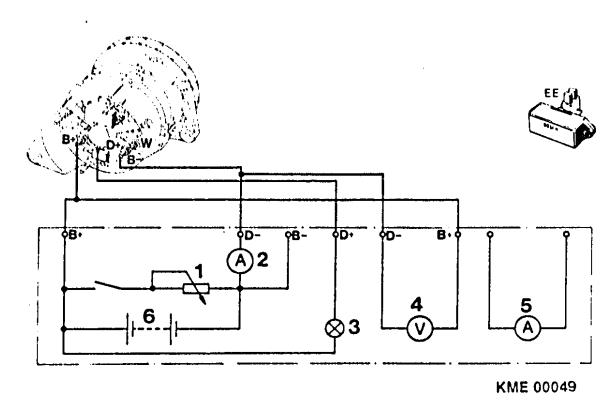
Figure 39 Alternator Test Bench Hook-up Schematic
