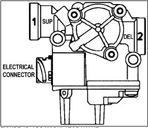
FIGURE 45: ABS MODULATOR VALVE
