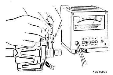
Figure 21 Rotor Resistance Testing
