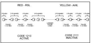
FIGURE 19: FLASHING FAULTS CODES
