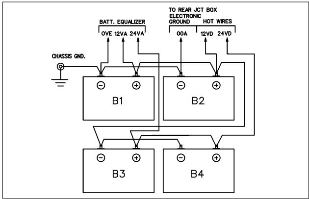
FIGURE 11: BATTERY CONNECTIONS
