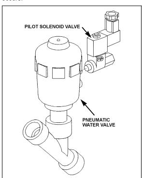
FIGURE 41: DRIVER'S HOT WATER PNEUMATIC VALVE ASSEMBLY 22240
