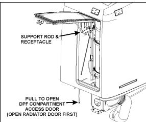
FIGURE 4: OPENING DPF COMPARTMENT ACCESS
