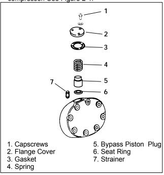
Figure 2-1. Removal of Piston Plug
