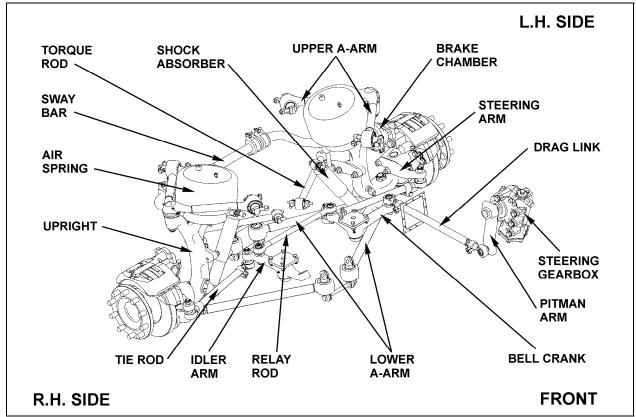
FIGURE 11: SUSPENSION AND STEERING LINKAGE
