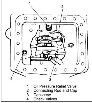
Figure 3-11. Bottom Plate and Oil Strainer Removed
