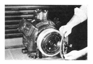
4. Remove the rotor retaining nut with special CTD tool P/N 07-00242-01.
