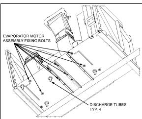
FIGURE 26: EVAPORATOR MOTOR ASSY FIXING BOLTS
