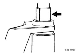
Figure 17 Sliding Bushing Removal
