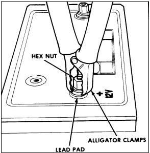
FIGURE 14: ALLIGATOR CLAMPS AND BATTERY 06065
