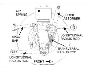
FIGURE 1: FRONT SUSPENSION COMPONENTS 10
