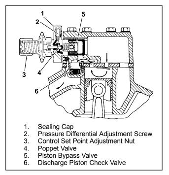
Figure 1-8. Pressure-Operated Unloader **Loaded Operation**
