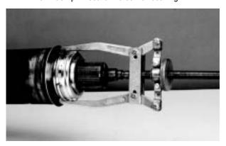
Inspect the midship for wear on the bearing diameter. If the midship is damaged from a seized bearing, replacement of the entire coupling shaft is necessary.
