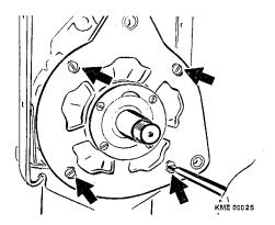
Figure 10 Drive End Shield Removal
