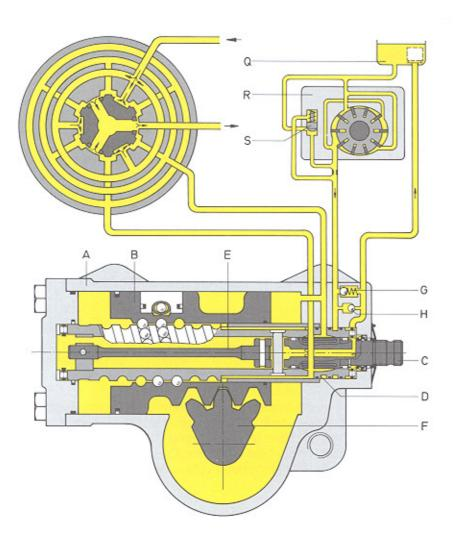
Fig. 1 Valve rotor in mid-position
