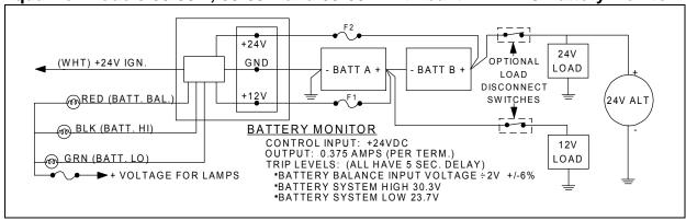
The EM-70 Battery Monitor provides the following ground signals: Battery HI when  $\pm$ 24 rises above 30.3V, Battery LO when  $\pm$ 24 falls below 23.7V, Battery BALANCE when  $\pm$ 12 is not within 6% of ( $\pm$ 24  $\pm$ 2). Each ground signal is rated 0.375 amps and should be protected by a 1 amp fuse.
