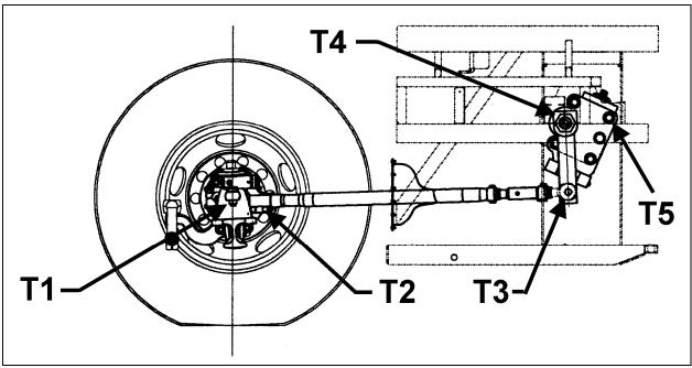
FIGURE 21: DRAG LINK COMPONENTS
