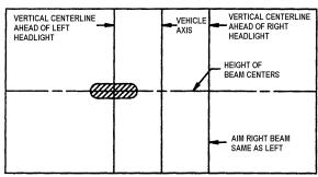
FIGURE 27: HIGH-INTENSITY ZONE (SHADED AREA) OF A PROPERLY AIMED UPPER BEAM ON THE AIMING SCREEN 7.6 M (25FT) IN FRONT OF VEHICLE 06503
