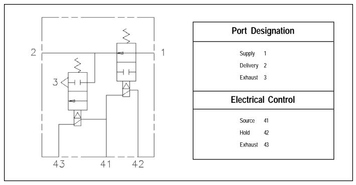
FIGURE 11: M-32™ AND M-32QR™ MODULATORS DIN SYMBOL
