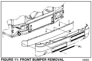
FIGURE 11: FRONT BUMPER REMOVAL
