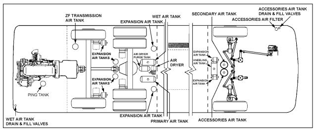
FIGURE 49: IFS AIR TANKS LOCATION
