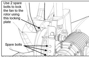
FIGURE 24: MECHANICAL LOCKING
