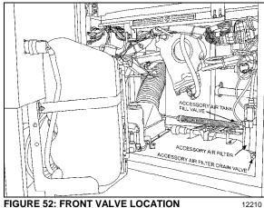
**FIGURE 52: FRONT VALVE LOCATION**
