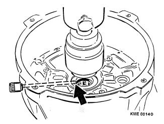
Figure 29 Installation of Bearing and Seal
