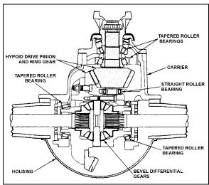
FIGURE 2: DIFFERENTIAL ASSEMBLY
