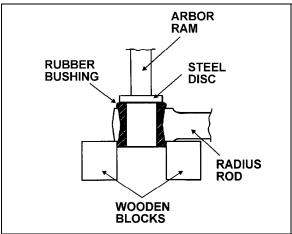
FIGURE 7: RADIUS ROD BUSHING REMOVAL
