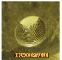
For hub piloted - normally if you see thread marks on the inside diameter of the bolt holes, this would indicate the wheel ran loose.
