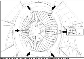
FIGURE 25: RADIATOR FAN MOUNTING BOLTS
