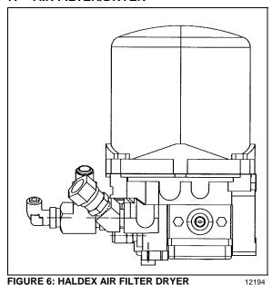
The air filter/dryer is located in front of rear wheelhousing above drive axle (Fig. 1, 2 & 6).
