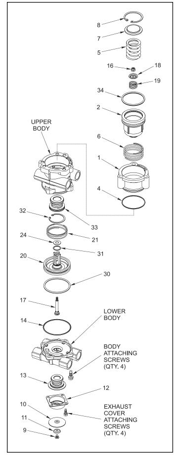
FIGURE 5 - ESPBRAKEVALVE - EXPLOSED VIEW
