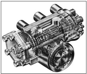
FIGURE 3: POWER STEERING GEAR
