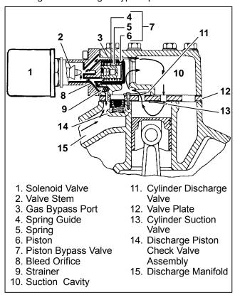
Figure 1-6. Electric-Operated Unloader-Unloaded Operation
