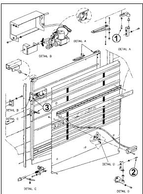
FIGURE 33: ENGINE COMPARTMENT R.H. SIDE DOOR 18635
