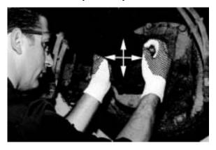
3. Grasp the end fitting with both hands and rotate left to right, feeling for play and backlash. There should not be any movement in the end fittings relative to the output or input shafts to which they are connected. If looseness is evident, consult transmission, axle, or transfer case original-equipment manufacturer's service and maintenance manuals for proper end fitting to shaft specifications.
