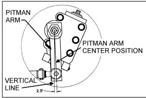
FIGURE 15: PITMAN ARM ADJUSTMENT
