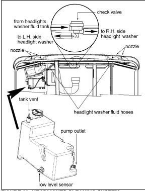
FIGURE 29: HEADLIGHTS CLEANING SYSTEM
