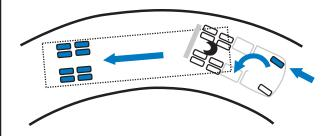
The Bendix® Yaw Control system reduces engine throttle and selectively applies brakes to reduce the tendency to jackknife.
