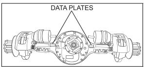
FIGURE 5: TYPICAL SERIAL & MODEL NUMBERS 00007
