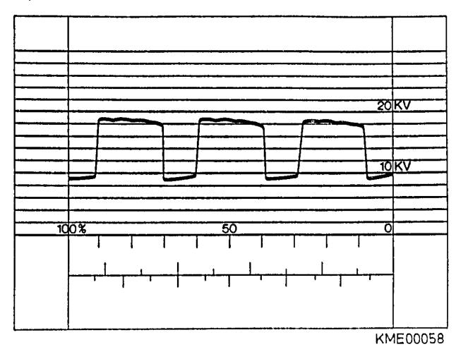
Figure 46 Shorted Negative Rectifier Diode
