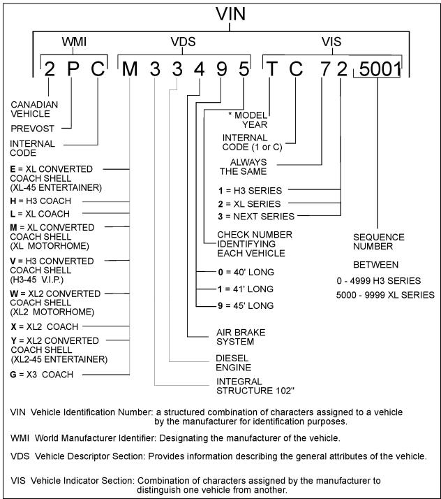
FIGURE 12: VEHICLE IDENTIFICATION NUMBER
