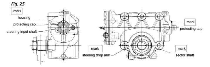
Now turn the steered wheels to the straight ahead driving position.
