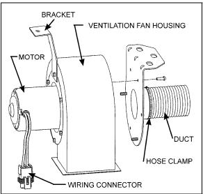
FIGURE 23: VENTILATION FAN INSTALLATION
