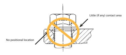
Incorrect use of flange nut positioned on Alcoa ball seat wheel. Do not use any flange nut on Alcoa aluminum ball seat wheels.
