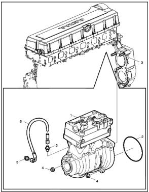
FIGURE 10: AIR COMPRESSOR LOCATION
