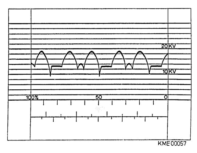
Figure 45 Shorted Positive Rectifier Diode
