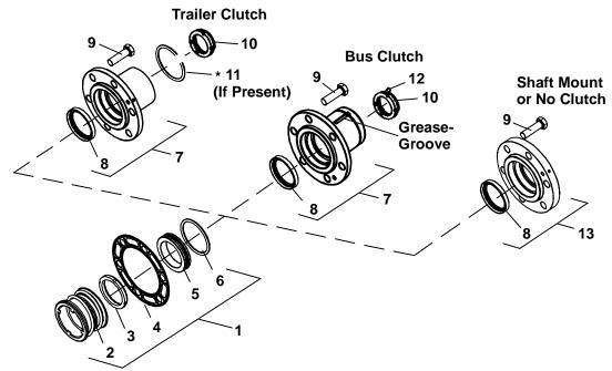
\*NOTE: Early production trailer compressors may have had the snap ring style clutch hub. Should the hub require replacement, it must be converted to the threaded clutch hub (Item 7).
