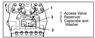
Figure 3-1. Shaft Seal Reservoir
