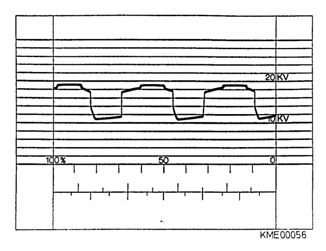
Figure 44 Shorted Exciter Diode
