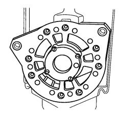
Figure 27 Drive End Bearing Retaining Screws
