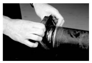
7. Using a puller, follow the tool manufacturer's instructions to remove the bearing assembly from the midship. Discard the center bearing.
