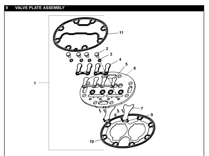
CAUTION: The above valve plate can only be used on the Twin Port 05G compressor.
