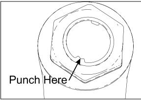
FIGURE 18: FIXING NUT PUNCH MARK
