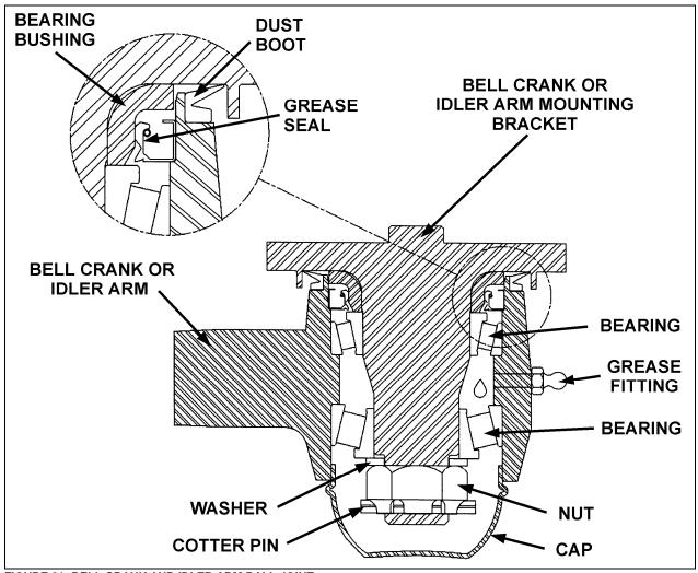
FIGURE 21: BELL CRANK AND IDLER ARM BALL JOINT
