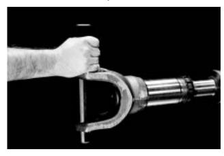
The alignment bar will identify yoke lugs that have taken a set because of excessive torque. The raised metal or distorted lugs can be a cause of premature cross and bearing problems.
