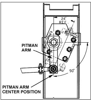
FIGURE 17: PITMAN ARM ALIGNMENT
