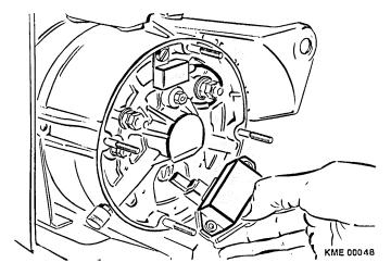
Figure 37 Regulator Installation All rights rest with Robert Bosch Corp, including patent rights. All rights of use of reproduction and publication rest with R. B. Corp.
