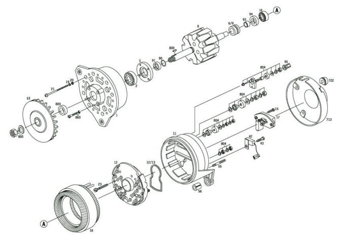
**Figure 4 Alternator Exploded View**
