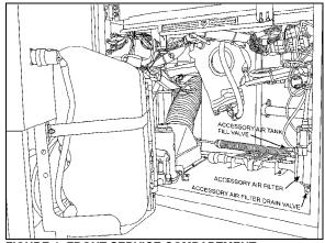
FIGURE 4: FRONT SERVICE COMPARTMENT
