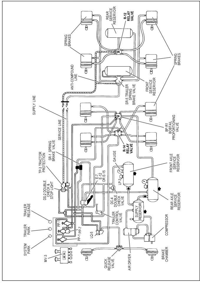
FIGURE 3 - TYPICAL PIPING SCHEMATIC
