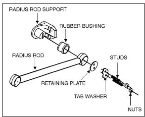
FIGURE 42: TYPICAL RADIUS ROD SETUP
