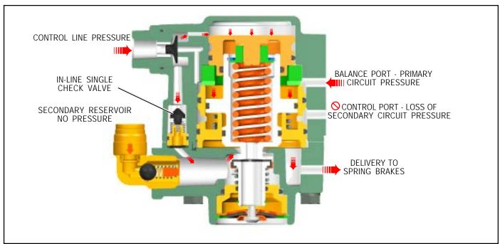
FIGURE 10 - SERVICE APPLICATION LOSS OF SECONDARY CIRCUIT
