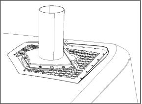
FIGURE 13: EXHAUST GAS COLLECTION ADAPTER04020
