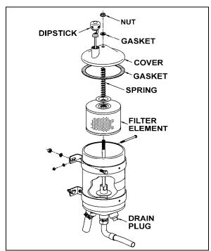
FIGURE 19: POWER STEERING FLUID RESERVOIR
