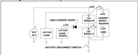
The system must be wired as shown to prevent Reverse Polarity Damage to polarity sensitive 12 volt loads and Family 1 and Family 2 Equalizers while the ground-side disconnect switch is open. The equalizer's GND terminamust be wired to the battery side of the ground-side disconnect switch circuit for the equalizer to work properly.
