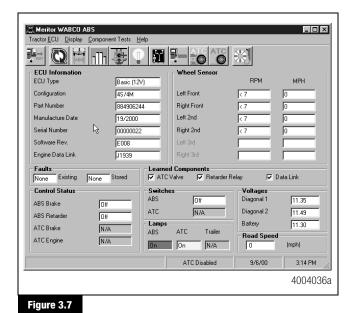
This screen provides information about the current state of Meritor WABCO ABS. ECU information is read once from the ECU and does not change. All other information (e.g., wheel sensors, control status, voltages, faults and road speed) is read and updated continuously.
