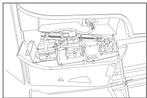
FIGURE 25: OPENING HEADLIGHT ASSEMBLY
