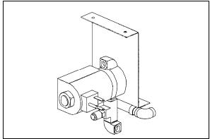
FIGURE 28: AIR HORN VALVE
