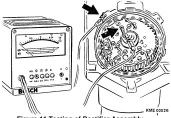
Figure 11 Testing of Rectifier Assembly
