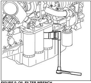
FIGURE 5: OIL FILTER WRENCH
