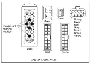
FIGURE 3: MULTIPLEX MODULE CONNECTORS PIN-OUT 06624
