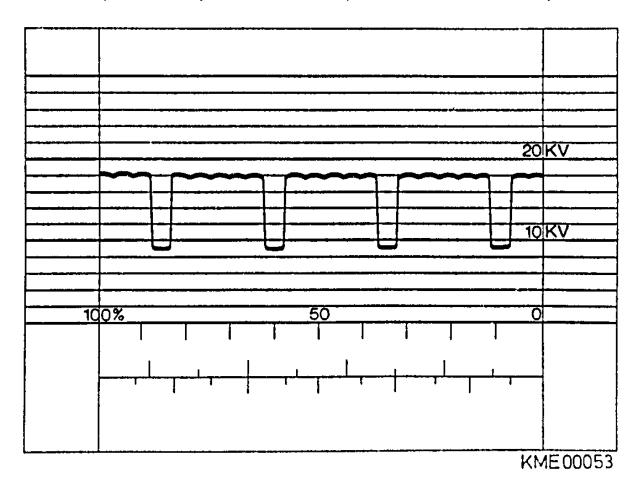
Figure 41 Open Exciter Diode
