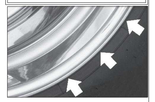
Heavy duty truck tires have a "guide rib" molded into the sidewall next to the tire bead. When the tire is inflated this ring should be evenly spaced from the wheel rim all the way around the wheel. Check the position of the ring before removing the assembly from the inflation cage. If the ring and wheel are not concentric, deflate the assembly in the cage and remount the tire.
