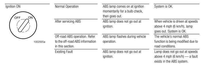
NOTE: If the ECU senses a tractor ABS fault during normal vehicle operation, the ABS indicator lamp will come on and stay on.
