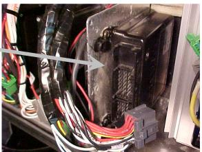
Unplug 1 connector from the master ID Disconnect CPC connectors Unplug 3 connectors from the CECM Unplug connector C92
