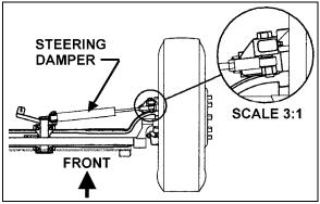
FIGURE 20: STEERING STABILIZER (DAMPER)
