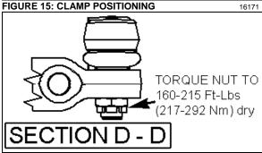
FIGURE 16: CLAMP POSITIONING
