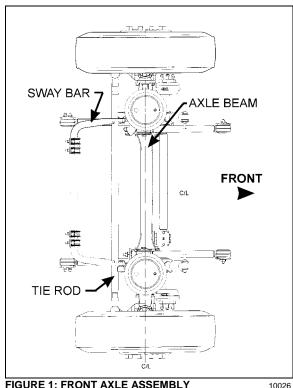
FIGURE 1: FRONT AXLE ASSEMBLY
