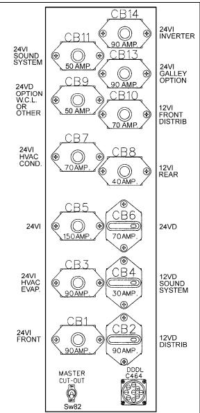
FIGURE 2: REAR ELECTRICAL JUNCTION PANEL
