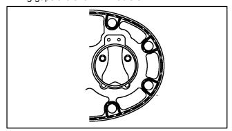
Figure 3-16. Correct Piston in Cylinder Orientation
