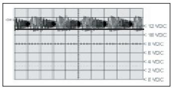
FIGURE 7 - POWER LINE WITH PLC SIGNAL
