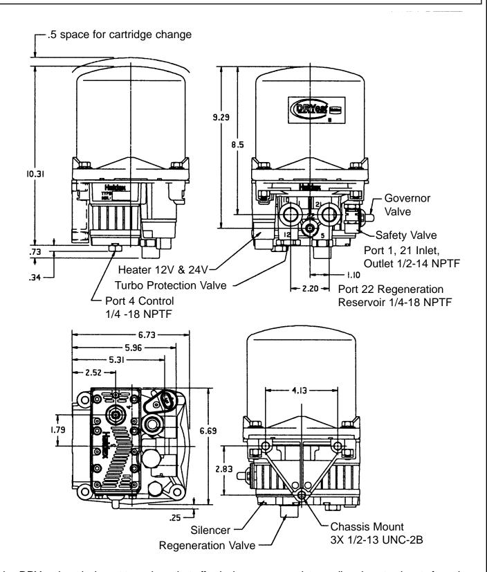
The Haldex DRYest is a desiccant type dryer that effectively removes moisture, oil and contaminants from the compressed air system. This reduces the risk of freezing or corrosion of the components in the air system. When compressor cut-out is reached, dry air is allowed to flow back to regenerate the desiccant bed. The SIX (6) different applications available for the DRYest are illustrated on the next page.
