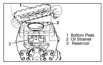
Figure 3-10. Bottom Plate Removal
