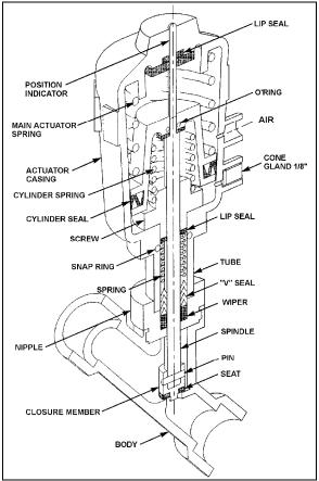
FIGURE 42: PNEUMATIC WATER VALVE
