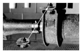
Visually inspect the center bearing rubber cushion for damage. Make sure the slingers are not rubbing against the rubber cushion. Verify that the rubber cushion is properly seated in the metal bracket. If any of these conditions are evident, replacement of the center bearing assembly is necessary. Refer to recommendations in the Disassembly and Reassembly on page 16 for proper center bearing replacement procedures.
