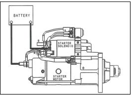
Figure 6 - TESTING HOLD-IN WINDINGS (GROUND-FLOAT TYPE)
