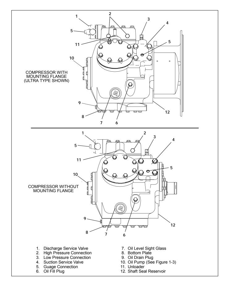
Figure 1-1. Model 05G Compressor
