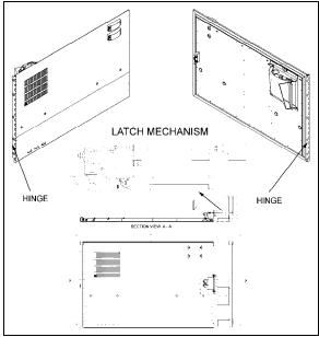
**FIGURE 36: EVAPORATOR DOOR**
