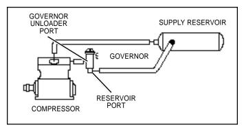
FIGURE 3 - BA-921 COMPRESSOR UNLOADER SYSTEM
