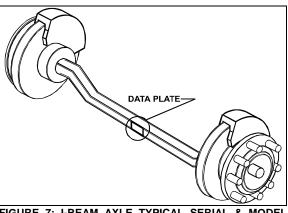
FIGURE 7: I-BEAM AXLE TYPICAL SERIAL & MODEL **NUMBERS**
