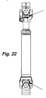
Using a suitable tool, for example a ratchet belt, constrict the ball-track relay shaft until there is sufficient space for the steering gear to be built in without constricting the ball-track relay shaft any further. (*Fig. 22*).
