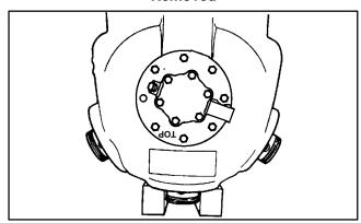
Figure 3-12. Piston Rings Removed
