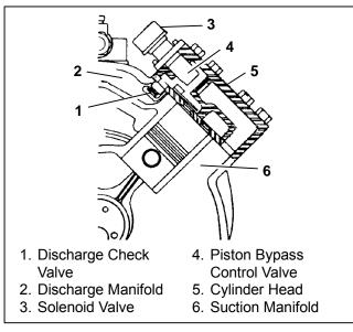
Figure 1-5. Compressor Unloader
