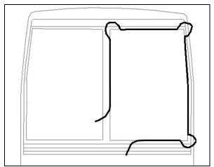
FIGURE 13: WINDSHIELD INSTALLATION USING ROPE
