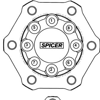
HUB FLANGE BOLT TIGHTENING TORQUE SEQUENCE FOR 10 BOLT FIXING
