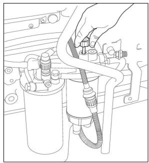
FIGURE 12: HAND PRIMING PUMP
