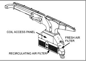
FIGURE 13: DRIVER'S SECTION AIR FILTERS
