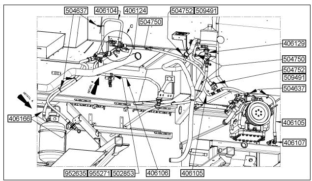
FIGURE 40: FIRE EXTINGUISHER INSTALLATION
