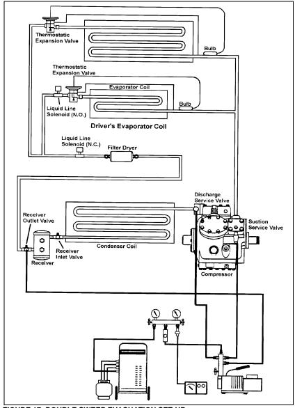
FIGURE 17: DOUBLE SWEEP EVACUATION SET-UP
