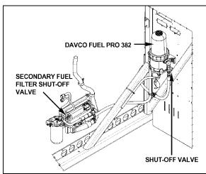
FIGURE 3: MANUAL SHUT-OFF VALVE WITH DAVCO FUEL PRO 382 (DDC S60 ENGINE) 0307:
