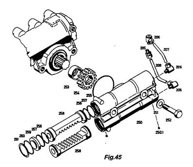
Slip two O-rings (256) and two gaskets (257) onto each pistor (258).
