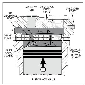
FIGURE 5 - OPERATIONAL-LOADED (COMPRESSION)
