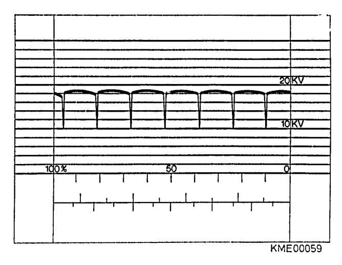
Figure 47 Open Stator Phase
