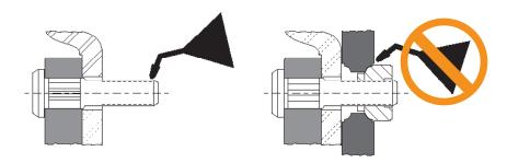
On vehicles equipped to accept wheels manufactured for use with the stud located ball seat mounting system, wheel studs on the right side of the vehicle have right-hand threads and those on the left have left-hand threads. The "R" and "L" on the studs and nuts indicate right and left-hand threads respectively (see Section 5-2).
