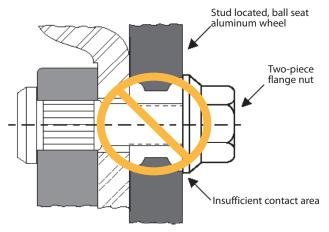
Do not use two-piece flange nuts with stud located ball seat wheels.
