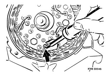
Figure 35 Soldering of Stator Leads
