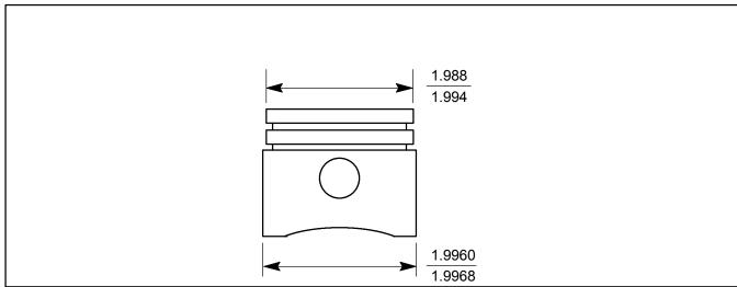
Figure 3-21. Piston Dimension (Wear Limits)
