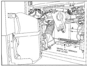
FIGURE 9: FRONT SERVICE COMPARTMENT
