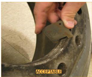
Hub bore gauge does not fit.
