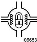
Illuminates when the differential action is locked
