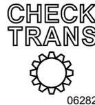
When the "CHECK TRANS" indicator is illuminated and the shift selector emits short beeps for 8 seconds, the transmission control module (TCM) is restricting transmission shifting because special or abnormal conditions are detected. The control pad display will be blank.
