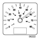
Indicates the vehicle speed in miles per hour (mph) and kilometers per hour (km/h). The digital odometer records the distance traveled in miles or in kilometers (units are driver selectable).
