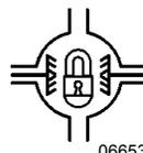
Illuminates when the differential action is locked
