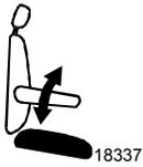
To lower or raise the seat's rear section, pull handle #4 up and push or pull the seat cushion.
