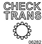
When the "CHECK TRANS" indicator is illuminated and the shift selector emits short beeps for 8 seconds, the transmission control module (TCM) is restricting transmission shifting because special or abnormal conditions are detected. The control pad display will be blank.
