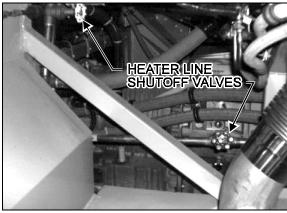
FIGURE 7: HEATER LINE SHUTOFF VALVES
