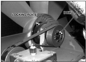
FIGURE 12: FAN-MECHANICAL LOCKING DEVICE 05033
