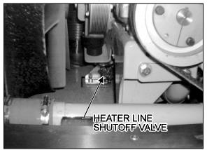
FIGURE 6: HEATER LINE SHUTOFF VALVE
