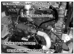
FIGURE 8: ENGINE COOLANT DRAIN COCKS
