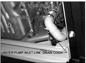
FIGURE 9: WATER PUMP DRAIN COCK (VIEWED FROM UNDERNEATH VEHICLE)
