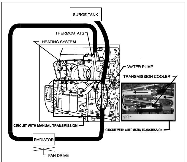
FIGURE 1: COOLING SYSTEM DESCRIPTION
