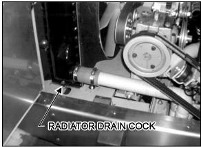
FIGURE 10: RADIATOR DRAIN COCK
