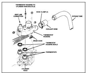
FIGURE 13: THERMOSTAT AND RELATED PARTS 05034
