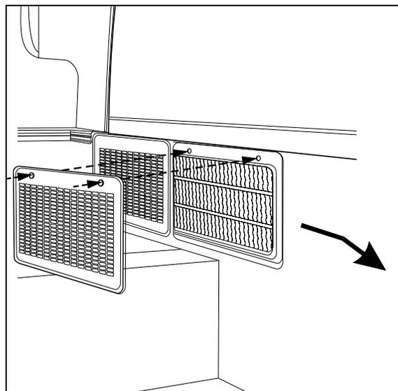
ACCESS TO DRIVER'S HVAC UNIT AIR FILTERS
