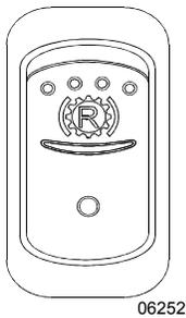
Press down this rocker switch to activate the transmission retarder.
