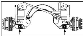
JACKING POINTS ON AUXILIARY AXLE
