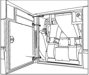
EVAPORATOR COMPARTMENT (WITH CENTRAL A/C SYSTEM ONLY) 22365
