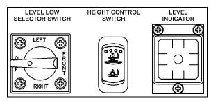
When driving, the conventional air leveling system of the vehicle controls the height at three points: the front, the left rear and the right rear. Your vehicle is equipped with a suspension system that consists of air springs (pressurized air bellows) located near each wheel. The amount of air in each air spring (and thus the vehicle height) is controlled by automatic leveling valves that operate between the chassis and the axles of the vehicle.
