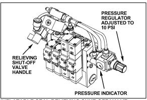
INFLATABLE SEAL RELIEVING SHUT-OFF VALVE 26098
