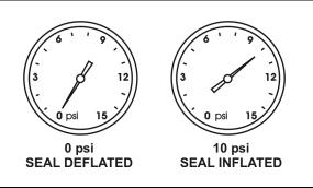
**INFLATABLE SEAL PRESSURE GAGE**
