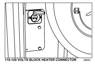
The vehicle is equipped with an engine immersion-type electric block heater to assist cold weather starting. A connector is located inside the engine R.H. side compartment. Using an extension cord, connect to a 120 VAC outlet. Use the engine block heater when the vehicle is parked in cold weather for a long period and the proper power source is available.
