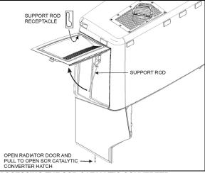
ACCESSING THE SCR CATALYTIC CONVERTER
