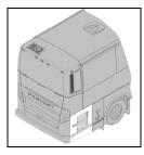
Lock this door using the exterior compartment key. Lift up protector cover to gain access to the lock. Pull up the door handle to release the latch and then pull the door open.
