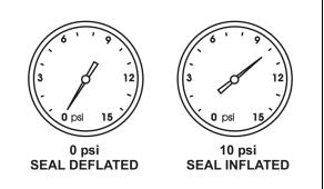
**INFLATABLE SEAL PRESSURE GAGE**
