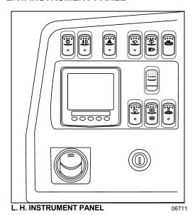
The L.H. instrument panel includes driver-exclusive controls, ignition switch and an adjustable air register for the driver.
