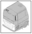
To open engine compartment door, first open engine compartment curbside door. Lift the latch release lever, place hand on the upper right of the rear door and pull rearward.
