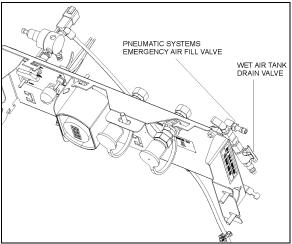
FILL VALVE IN ENGINE COMPARTMENT
