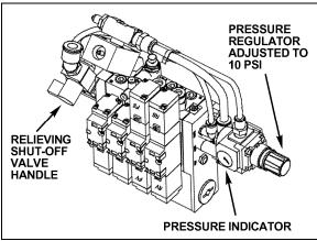
INFLATABLE SEAL RELIEVING SHUT-OFF VALVE 26098
