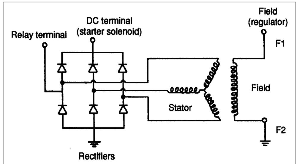
FIGURE 65: ALTERNATOR WIRING DIAGRAM
