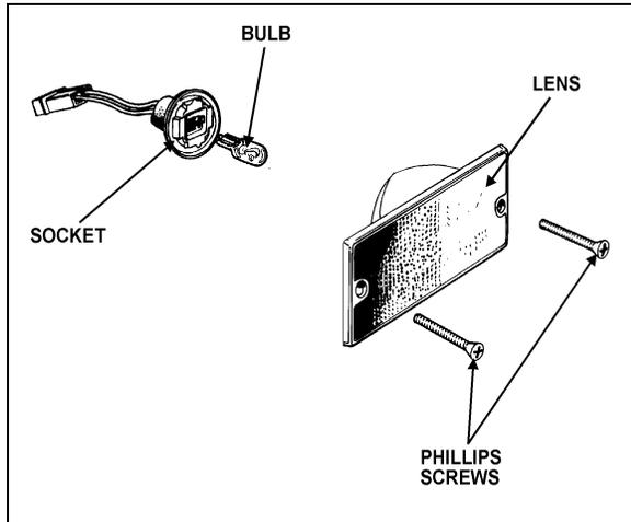
FIGURE 102: TYPE "B" LIGHT BULB 06155
