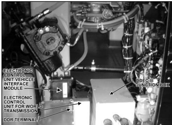
FIGURE 35: STEERING COMPARTMENT 06120
