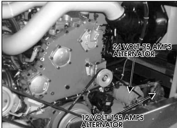
FIGURE 74: ENGINE REAR COMPARTMENT (ALTERNATOR)
