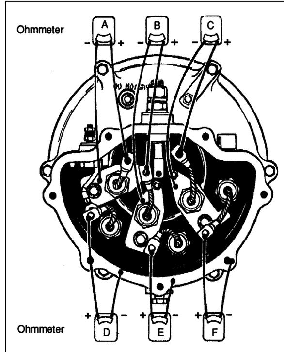
FIGURE 68: DIODES TEST
