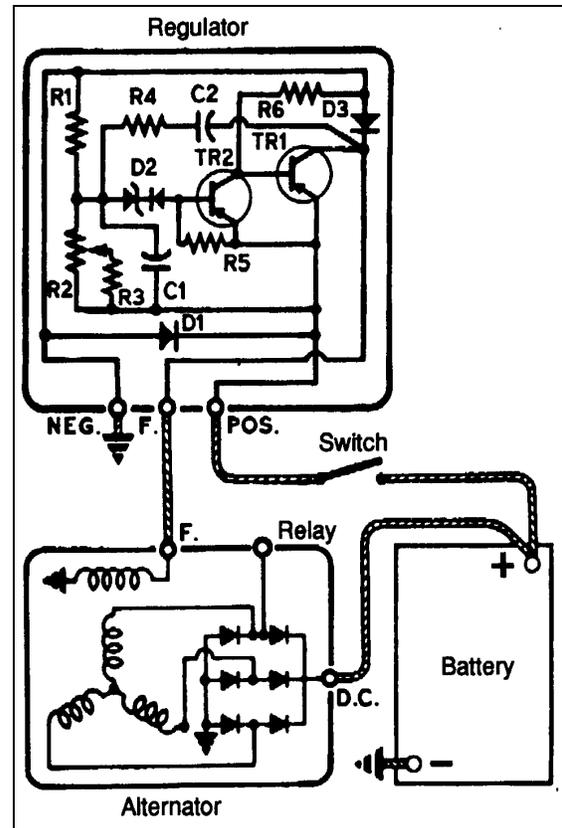
FIGURE 81: TYPICAL WIRING DIAGRAM OF NEGATIVE GROUND SYSTEM 0
