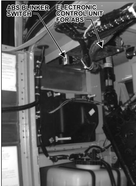
FIGURE 34: STEERING COMPARTMENT (LEFT WALL) 06119
