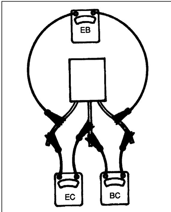
FIGURE 86: TRANSISTOR TEST
