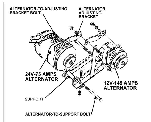
FIGURE 78: 12V-145 AMPS AND 24V-75 AMPS ALTERNATORS 06144
