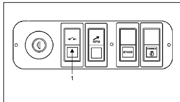
FIGURE 19: L.H. LOWER SWITCH PANEL (BATTERY MASTER SWITCH) 18116
