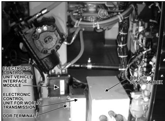
FIGURE 10: STEERING COMPARTMENT 06120
