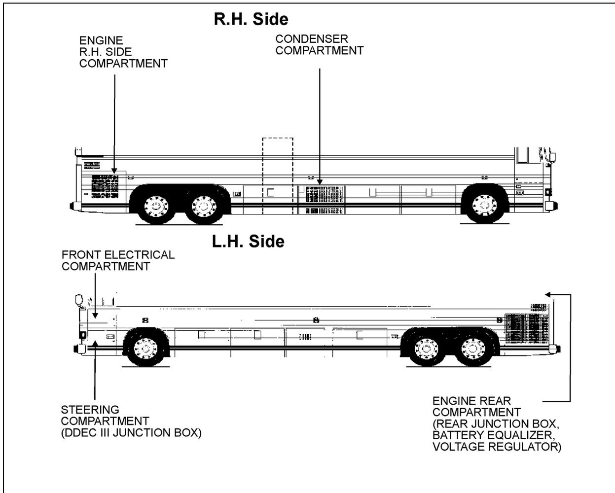
FIGURE 30: ELECTRICAL COMPARTMENT (XL-40 AND XL-45E CONVERTED VEHICLES)
