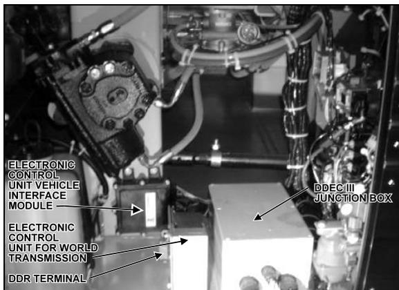
FIGURE 24: STEERING COMPARTMENT 06120
