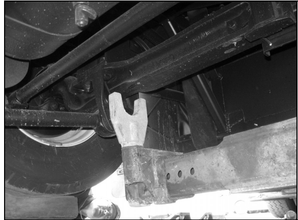
LIFTING FROM UNDER THE FRONT AXLE
