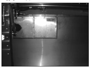
**Note:** Optional auxiliary fuel tank has a label affixed to the side of the tank and can be easily read through the second (third on XL-45E) baggage compartment door.
