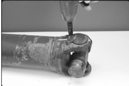
FIGURE 15: SPRING TAB BOLTS REMOVAL
