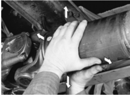
FIGURE 6: CHECK FOR LOOSENESS
