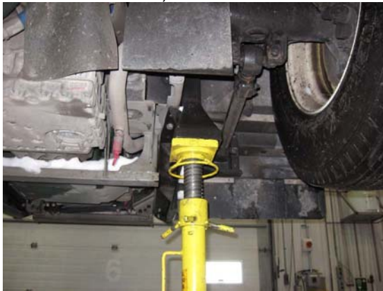
FIG.7 JACK STAND AT CHASSIS HOISTING RECEPTACLE - AFT OF TAG AXLE, ROAD SIDE
