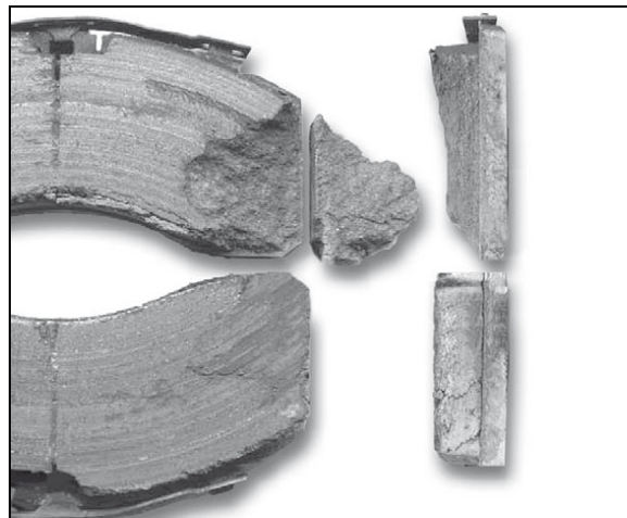
FIGURE 32: MAJOR BREAKOUTS ON THE SURFACE OF THE BRAKE PAD ARE NOT PERMITTED
