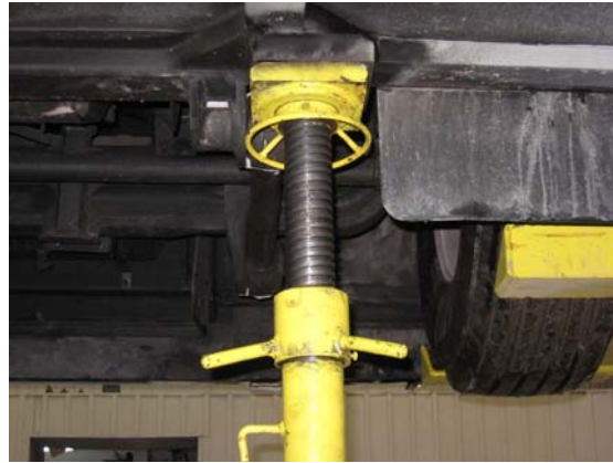
FIG.6 JACK STAND AT CHASSIS HOISTING RECEPTACLE - AFT OF FRONT AXLE, CURB SIDE
