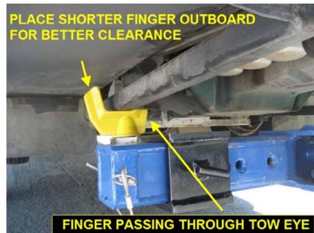
FIG.62 PROPER LOCATION WHEN LIFTING THE SIDE-MEMBERS – ON THIS PICTURE, THE BUS IS EQUIPPED WITH REAR TOW EYES
