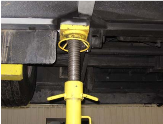
FIG.5 JACK STAND AT CHASSIS HOISTING RECEPTACLE - AFT OF FRONT AXLE, ROAD SIDE
