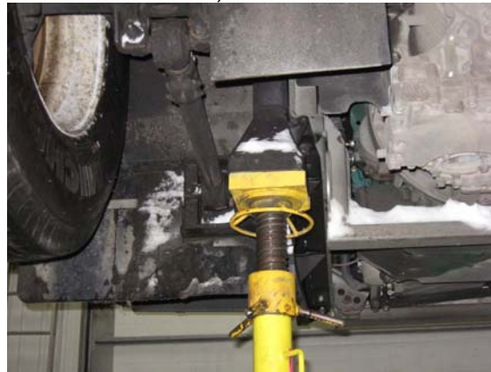
FIG.8 JACK STAND AT CHASSIS HOISTING RECEPTACLE - AFT OF TAG AXLE, CURB SIDE
