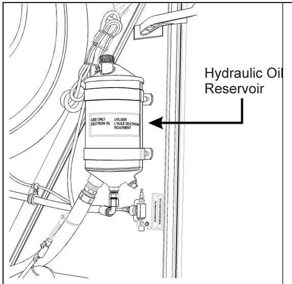
FIGURE 24: HYDRAULIC FLUID RESERVOIR LOCATION
