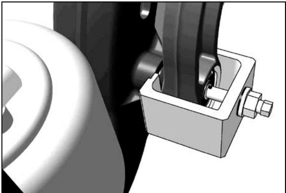
FIGURE 12: INSTALLING EXTRACTOR TOOL
