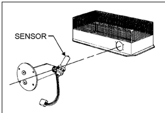
FIGURE 7: THERMISTOR SENSOR
