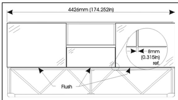
FIGURE 59: FACE FIXED WINDOW INSTALLATION
