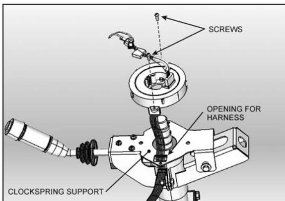
**FIGURE 13: CLOCKSPrING INSTALLATION**
