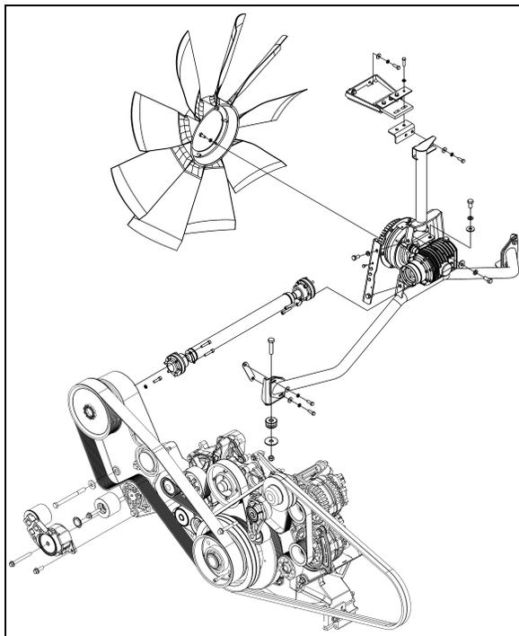
FIGURE 21: COOLING FAN DRIVE MECHANISM
