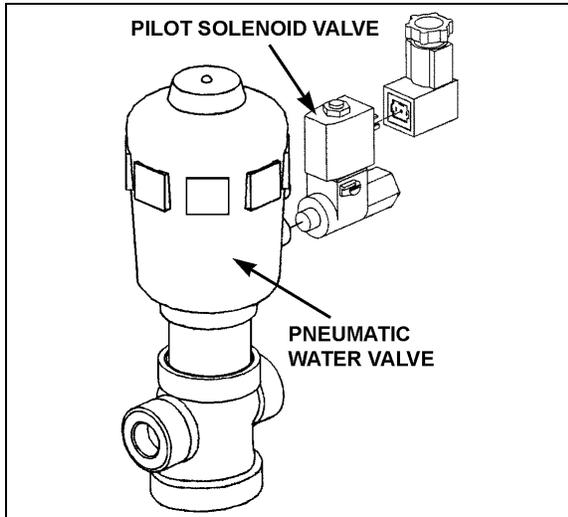
FIGURE 46: CENTRAL HOT WATER PNEUMATIC VALVE ASSEMBLY 22329
