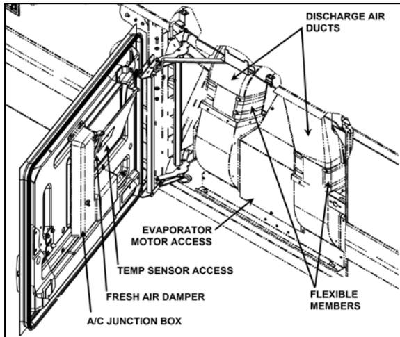
FIGURE 24: EVAPORATOR COMPARTMENT 22301\_B
