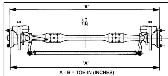
FIGURE 5: TOE-IN MEASUREMENT
