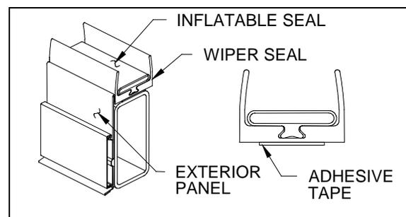
FIGURE 30: SEAL ASSEMBLY
