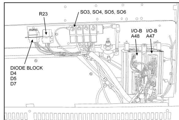
FIGURE 17: ENTRANCE DOOR &amp; WIPER CONTROL PANEL
