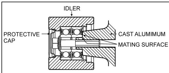
FIGURE 24: IDLER MOUNTED ON THE CAST ALUMINUM SUPPORT
