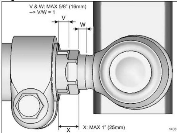
**FIGURE 23: DRAG LINK ADJUSTMENT SYSTEM**
