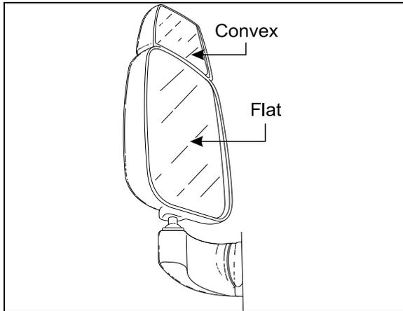
FIGURE 14: REAR VIEW MIRROR (RAMCO) 18398A
