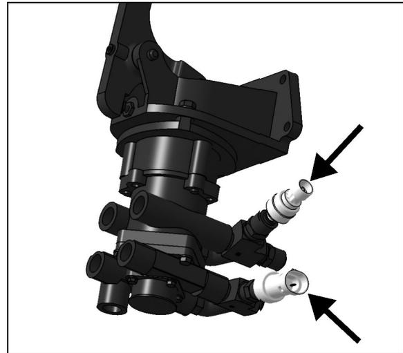
FIGURE 15: PRESSURE SWITCHES
