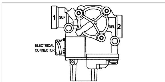
FIGURE 34: M-32QR PRESSURE MODULATOR VALVE
