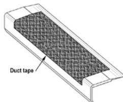
11. Apply some masking tape onto the step perimeter, clean using Sika 205 (refer to Section B) then apply a bead of Sika 252 black. Smooth out the joints then remove masking tape.
