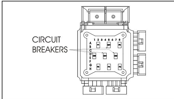
FIGURE 36: VEC CIRCUIT BREAKERS & FUSES
