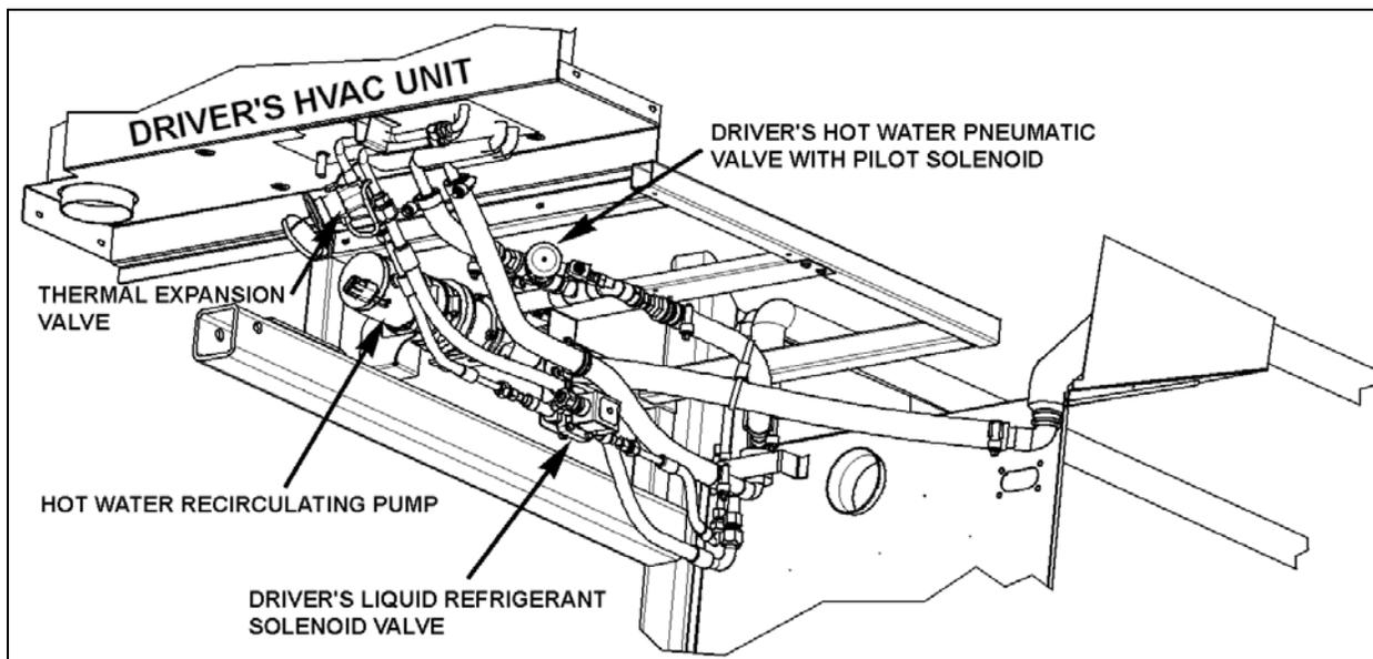
**FIGURE 53: CEILING OF THE SPARE WHEEL COMPARTMENT**
