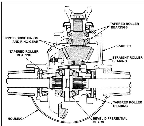
FIGURE 2: DIFFERENTIAL ASSEMBLY
