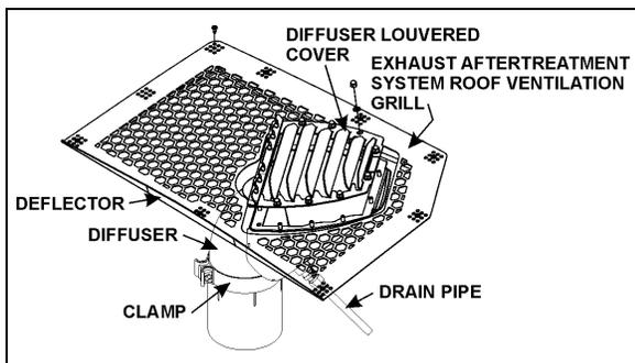
FIGURE 6: DIFFUSER ASSEMBLY 04014
