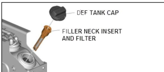
5. Flush the tank with hot water. Let all of the water drain from the tank.
