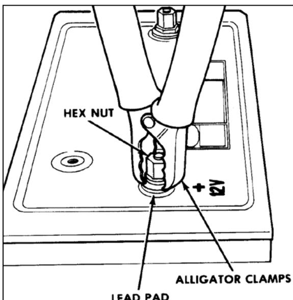
FIGURE 20: ALLIGATOR CLAMPS AND BATTERY 06065
