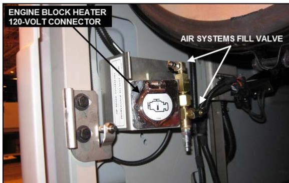
FIGURE 53: REAR VALVE LOCATION
