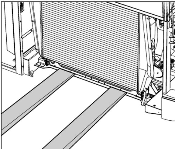
FIGURE 17: POSITIONING FORKLIFT
