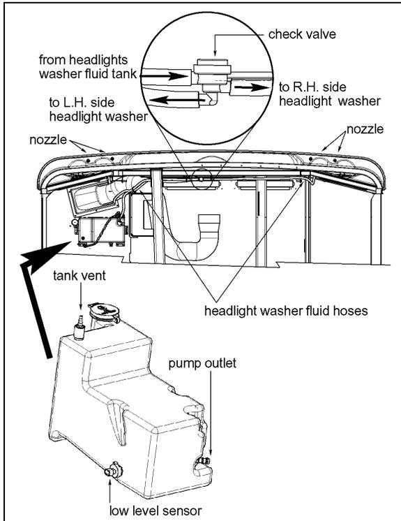
FIGURE 30: HEADLIGHTS CLEANING SYSTEM 23380
