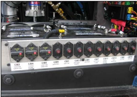
FIGURE 10: REAR ELECTRICAL JUNCTION PANEL
