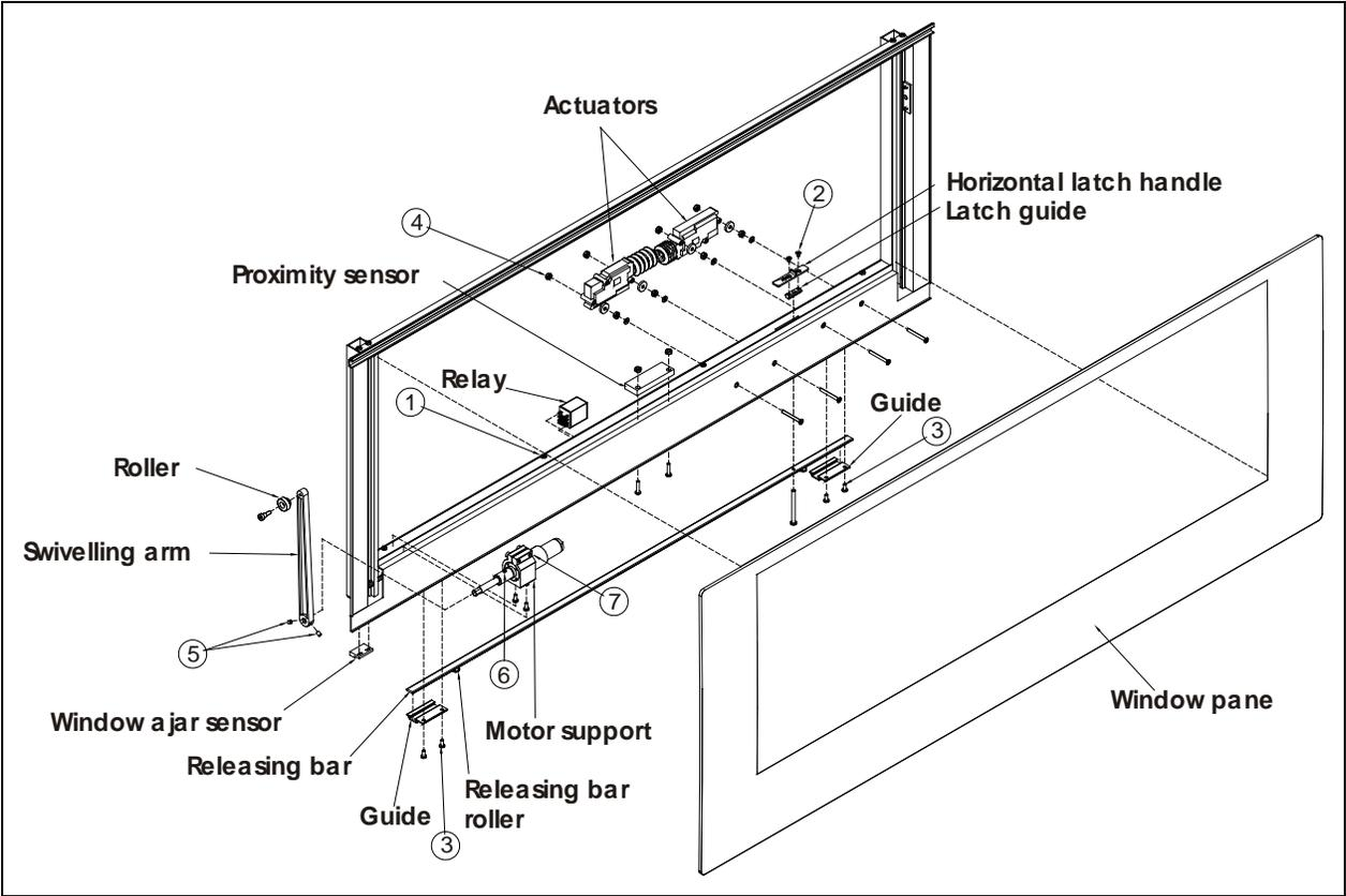
FIGURE 62: ELECTRIC AWNING WINDOW EXPLODED VIEW (SASH) 18583
