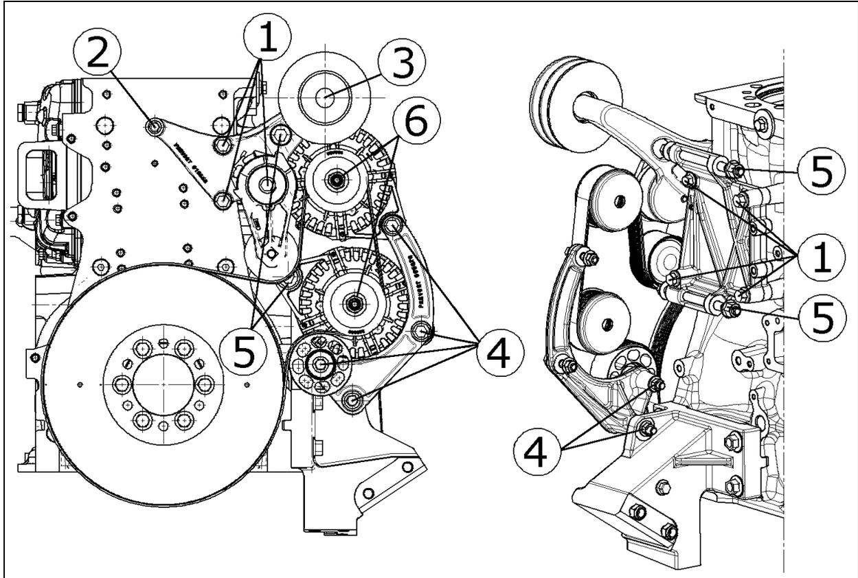
FIGURE 29: TWIN BOSCH ALTERNATORS INSTALLATION (X3-45 COACH)
