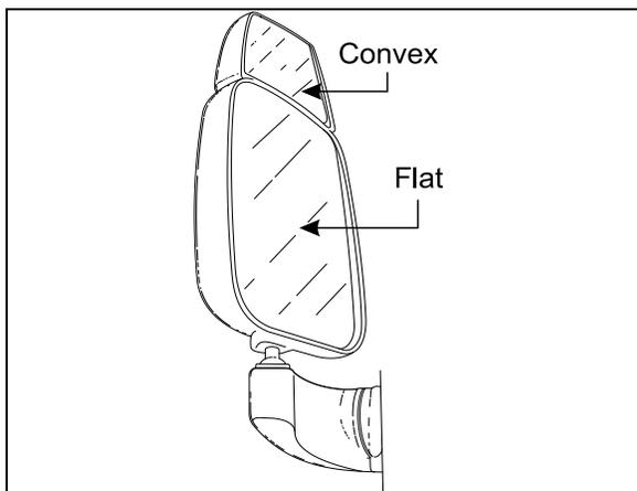
FIGURE 56: REAR VIEW MIRROR (RAMCO) 18398A
