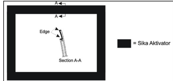
**FIGURE 54: FACE FIXED WINDOW AND HALF-WINDOW – SIKA AKTIVATOR**
