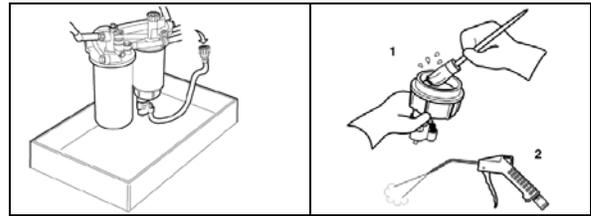
4. Unscrew and remove the primary fuel filter from the fuel filter housing. Drain filter.
