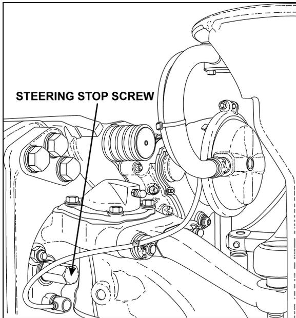
FIGURE 16: STEERING STOP SCREW ON I-BEAM AXLE
