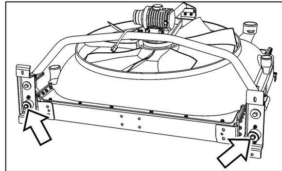
FIGURE 18: REMOVING FASTENERS
