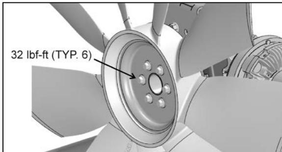
FIGURE 26: RADIATOR FAN MOUNTING BOLTS 05125
