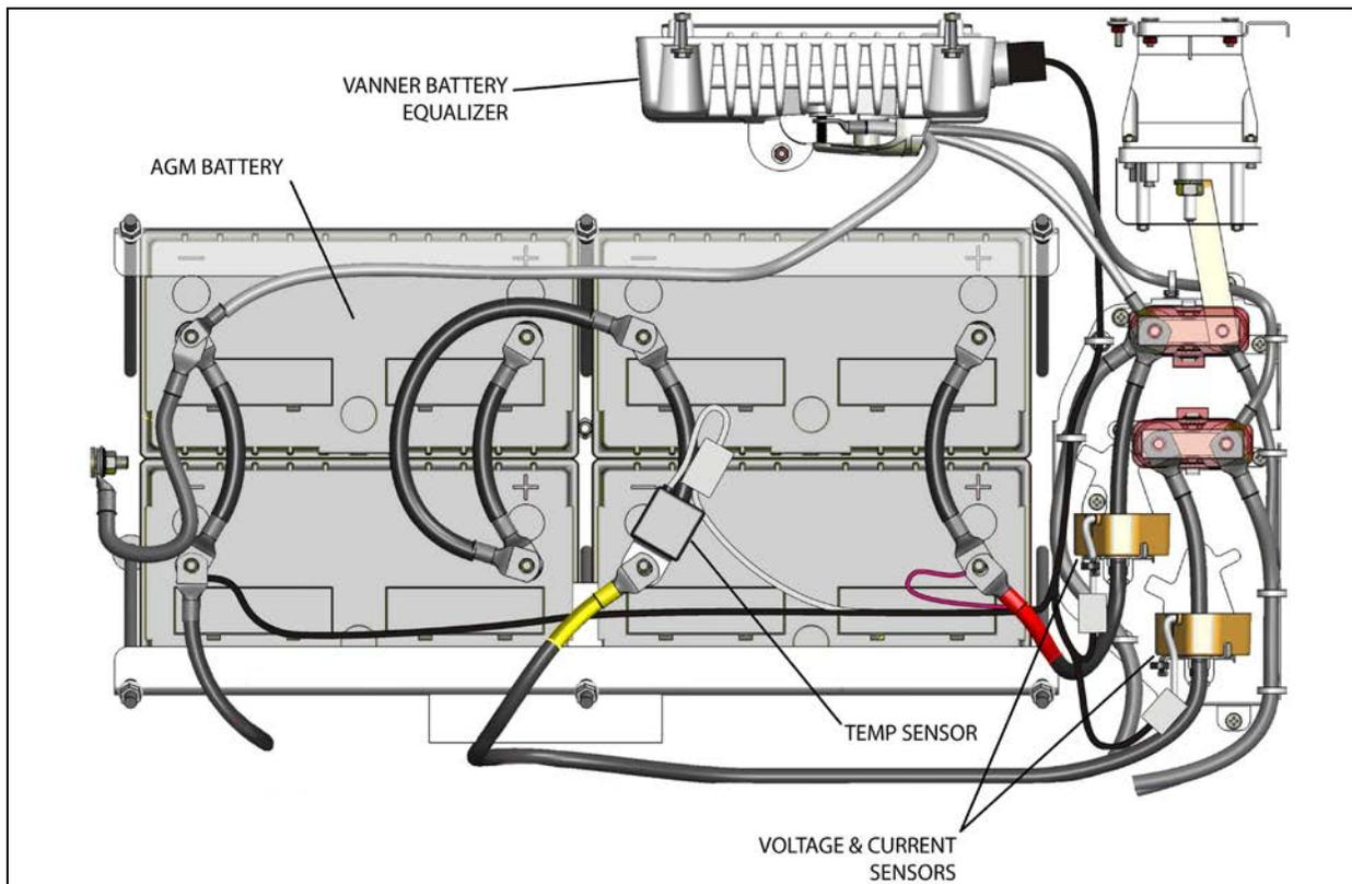
FIGURE 22: PRIME ELECTRICAL COMPONENTS
