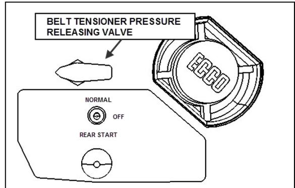
FIGURE 36: PRESSURE RELEASING VALVE
