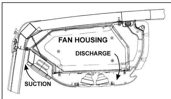
FIGURE 4: PASSENGERS OVERHEAD COMPARTMENT VENTILATION SYSTEM
