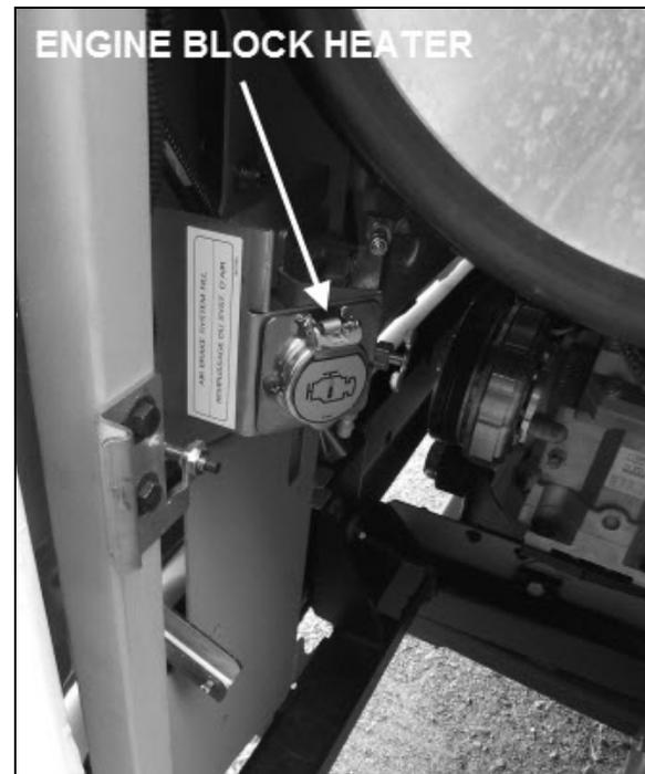
FIGURE 30: ELECTRIC HEATER CONNECTION
