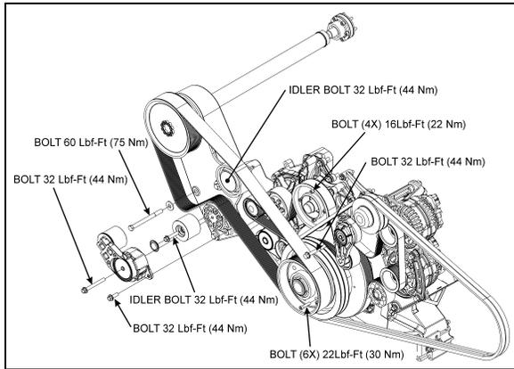
FIGURE 23: TIGHTENING SPECIFICATION (VOLVO D13 ENGINE)
