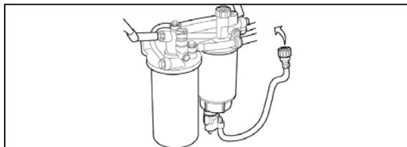
11. Connect the electrical connector for the water/fuel separation bowl indicator.
