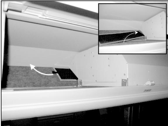
FIGURE 18: OVERHEAD COMPARTMENT FAN AIR FILTER
