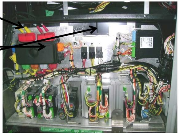
Disconnect 4 connectors from the ABS module
