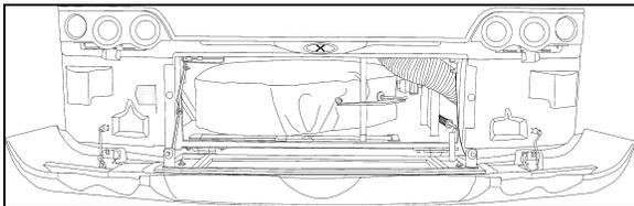
**FIGURE 11: X3 SERIES SPARE WHEEL COMPARTMENT**
