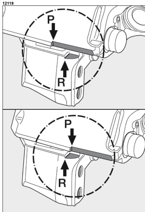
FIGURE 25: PAD WEAR CHECK FRONT AND TAG AXLE
