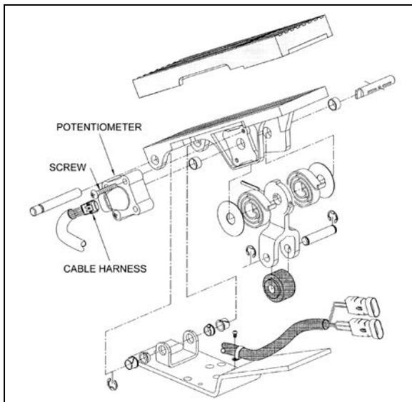
FIGURE 13: ELECTRONIC FOOT PEDAL ASSEMBLY 3035
