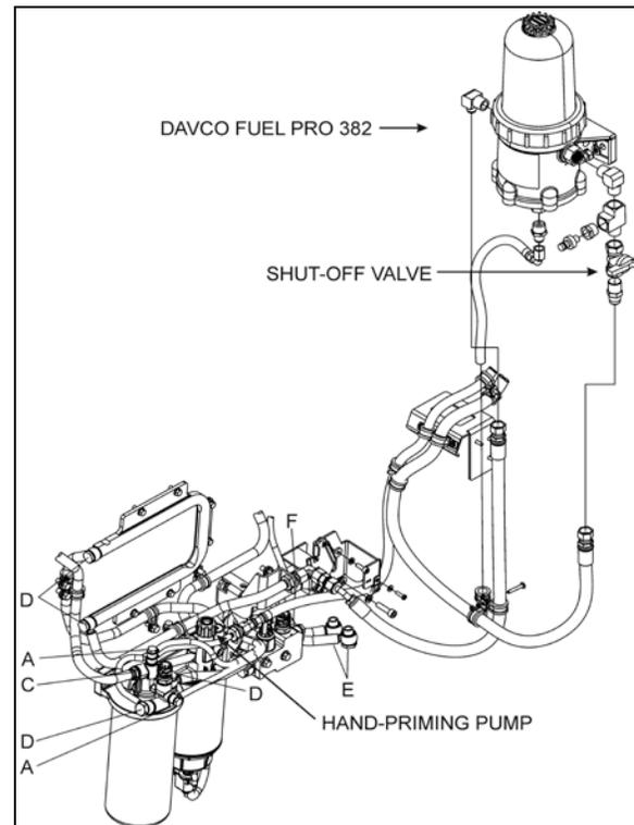
FIGURE 3: MANUAL SHUT-OFF VALVE LOCATION WITH DAVCO FUEL PRO 382 (VOLVO D13 ENGINE)
