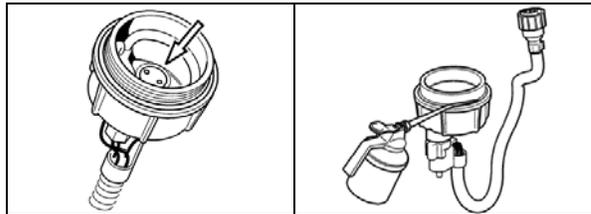
7. Check that the drainage hole in the water separator bowl is not blocked.
