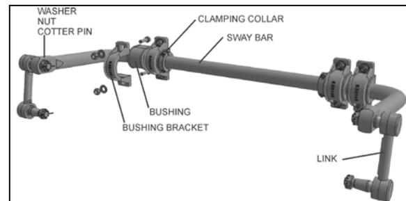
FIGURE 7: I-BEAM FRONT AXLE SWAY BAR 16028
