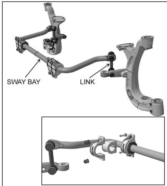
FIGURE 34: SWAY BAR (INDEPENDENT FRONT SUSPENSION)<sup>16138\_C</sup>
