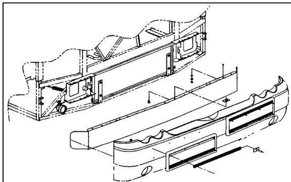
FIGURE 13: FRONT BUMPER REMOVAL 18665
