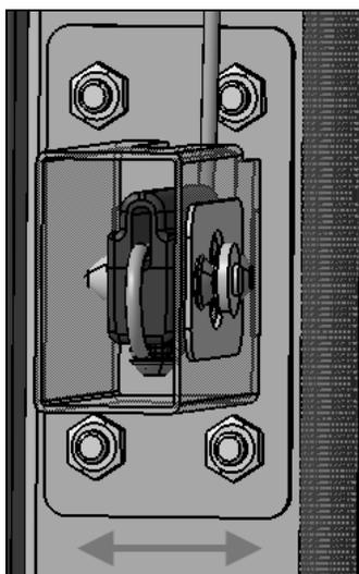
12. Make sure that backing plate is parallel to structure before tightening the retainer support hardware
