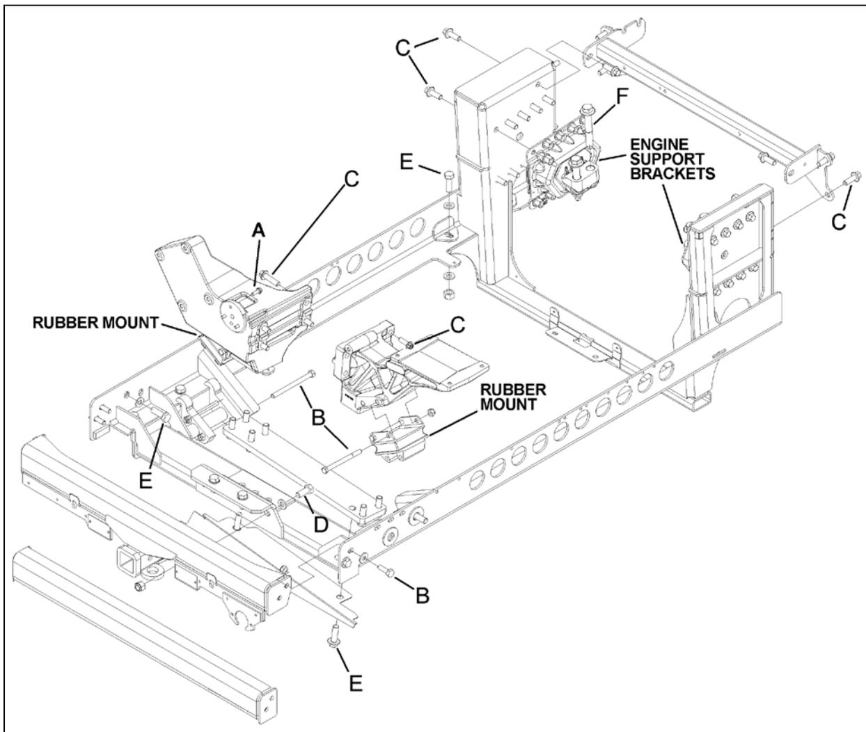
**FIGURE 12: VOLVO ENGINE POWER PLANT CRADLE INSTALLATION**
