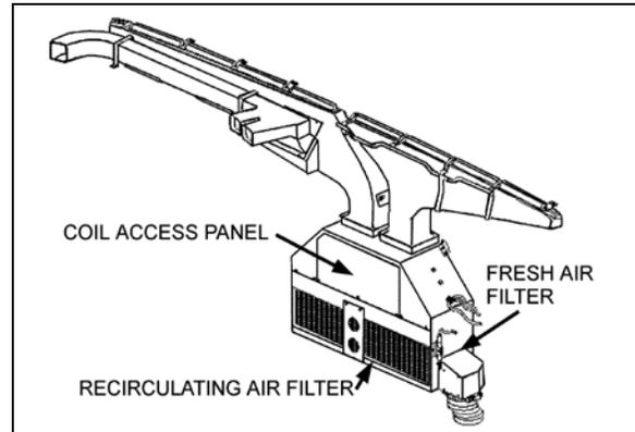
FIGURE 11: DRIVER'S HVAC UNIT COIL ACCESS PANEL
