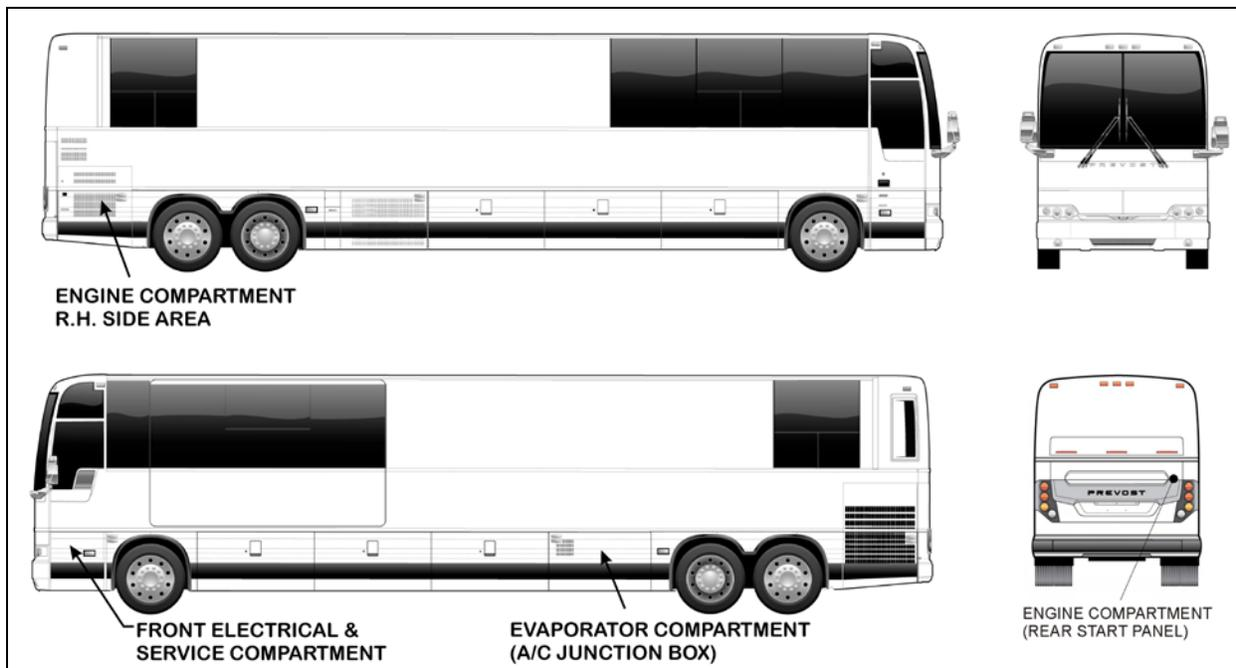
FIGURE 6: ELECTRICAL COMPARTMENTS (X3-45 VIP COMERCIAL BUS SHELL)
