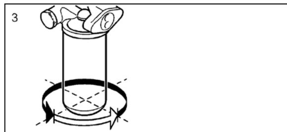
FIGURE 7: OIL FILTER REPLACEMENT
