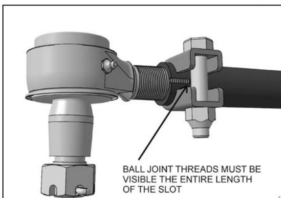
**FIGURE 20: ADEQUATE CLAMPING CONDITION**
