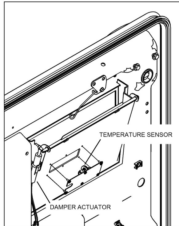
FIGURE 2: PASSENGERS' AREA FRESH AIR DAMPER 22302\_A
