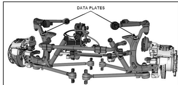
FIGURE 5: ISF TYPICAL SERIAL & MODEL NUMBERS 16136
