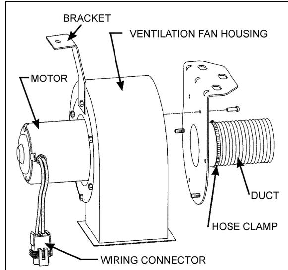
FIGURE 24: VENTILATION FAN INSTALLATION 23222
