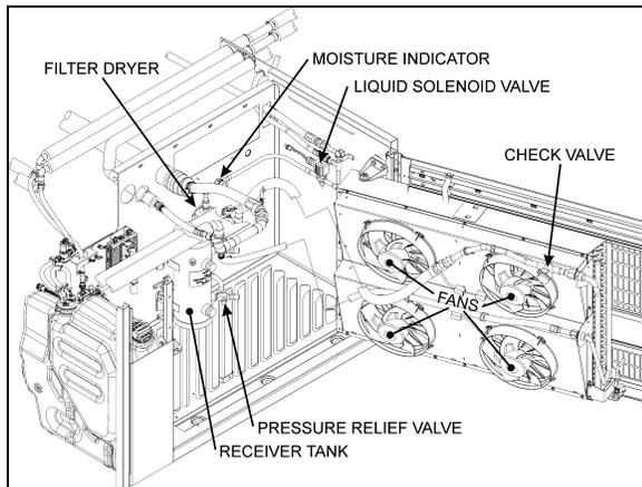
FIGURE 29: A/C CONDENSER COMPARTMENT 22323
