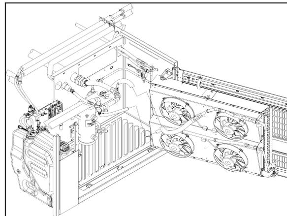
FIGURE 9: CONDENSER COMPARTMENT 22299
