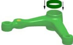
3. Insert the large bearing outer race into appropriate bore (done on a press).
