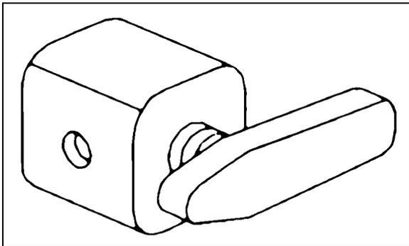
FIGURE 21: THREE-WAY VALVE
