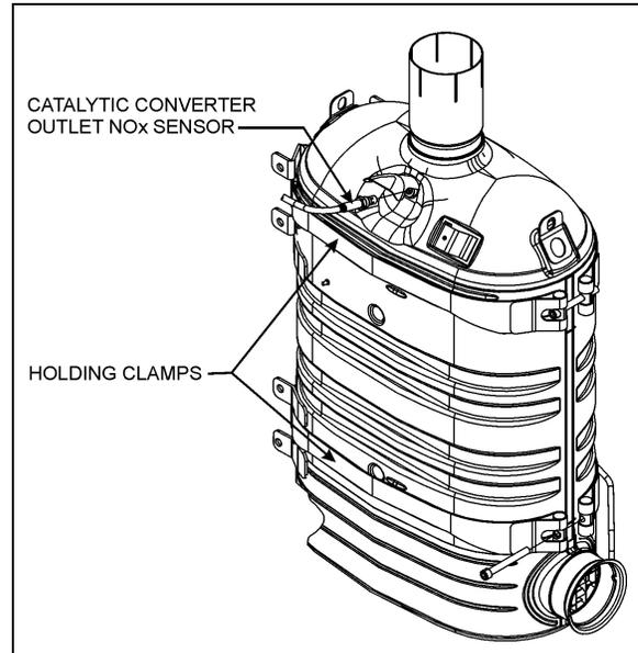
FIGURE 5: CATALYTIC CONVERTER
