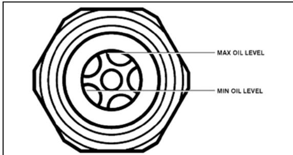
FIGURE 13: SIGHT GLASS FOR CHECKING OIL LEVEL
