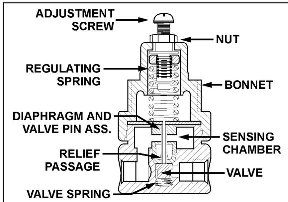
FIGURE 9: AIR PRESSURE REGULATING VALVE 12141A
