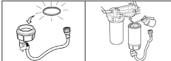
9. Install a new gasket to the water separation bowl and then reinstall the separation bowl to the new primary fuel filter cartridge.
