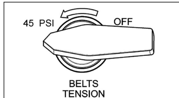
**FIGURE 10: BELT TENSIONER VALVE ON REAR CONTROL PANEL**
