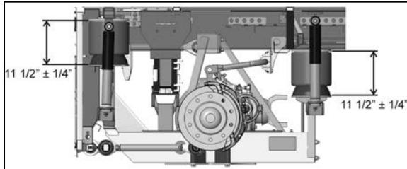
FIGURE 46: DRIVE AXLE AIR SPRING CLEARANCE 16195
