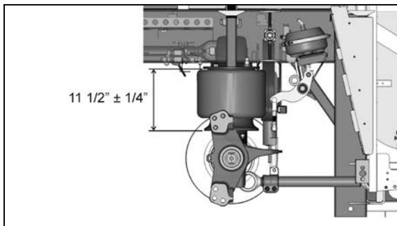
FIGURE 47: TAG AXLE AIR SPRING CLEARANCE 16195
