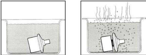
2. After at least 30 seconds, check that the thermostat is still closed.
