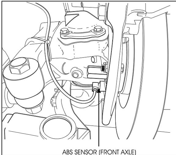
FIGURE 32: ABS SENSOR LOCATION
