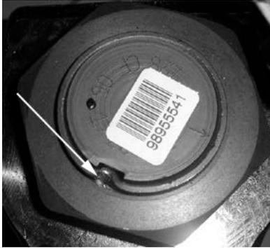
FIGURE 14: FIXING NUT PUNCH MARK
