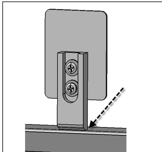
10. Make sure that skid bar only touches slightly bus structure at bottom. The door should not move up when closing.
