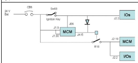
JB6 is a wake-up pin. JA15 output remains active for 5 minutes after JB6 is inactive.
