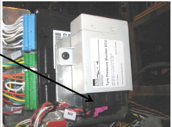
Disconnect connector A 83 under Volvo Link
