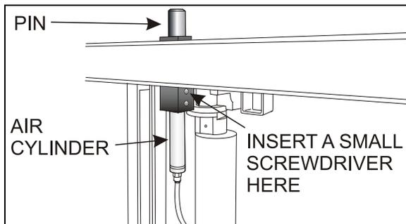
FIGURE 8: SECURITY PIN AIR CYLINDER REMOVAL
