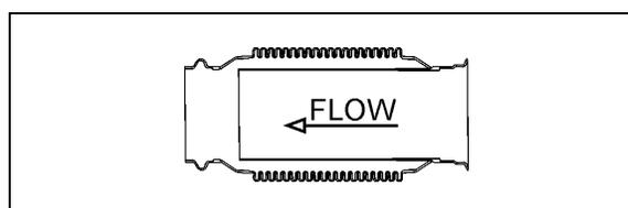
FIGURE 2: FLEXIBLE COUPLING
