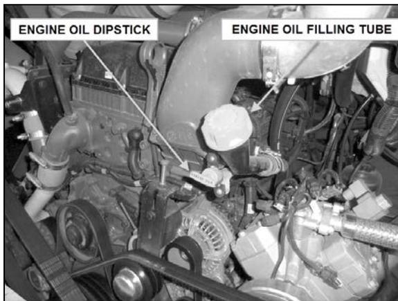
FIGURE 8: ENGINE OIL FILLING TUBE
