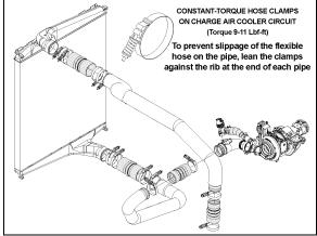
FIGURE 4: CHARGE AIR COOLER HOSE CLAMPS
