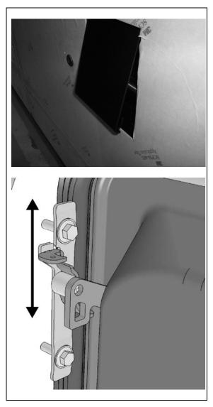
Make sure that skid bar only touches slightly bus structure at bottom. The door should not move up when closing.
