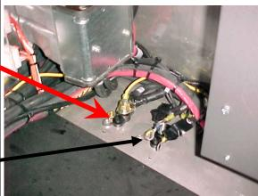
Using electric tape, insulate the 2 largest gage wires. Make sure the ring terminals do not touch each others and the vehicle body.
