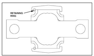
FIGURE 29: UPPER A-ARM BAR PIN BUSHING
