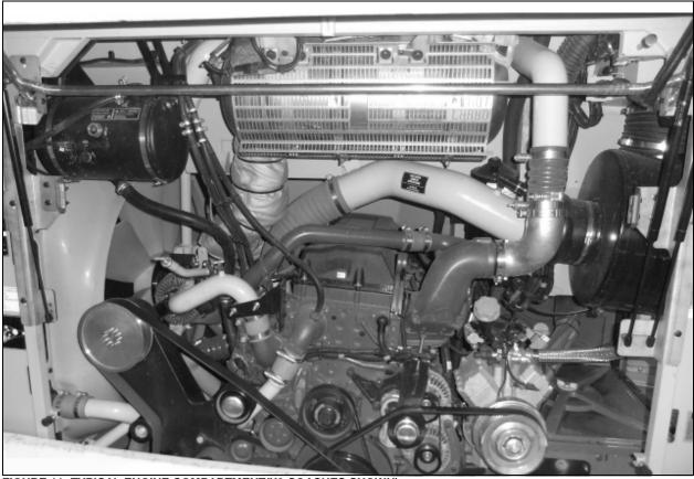
FIGURE 11: TYPICAL ENGINE COMPARTMENT(X3 COACHES SHOWN)
