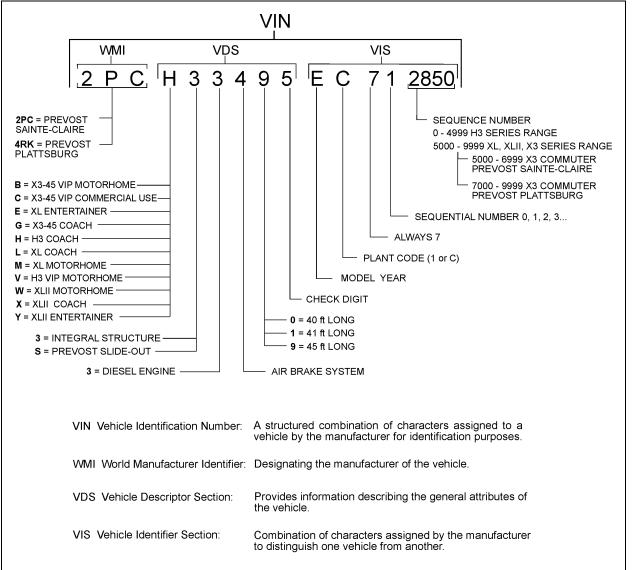
FIGURE 11: VEHICLE IDENTIFICATION NUMBER
