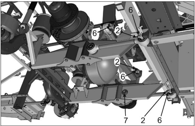
FIGURE 57: TORQUE SPECIFICATIONS - DRIVE AXLE
