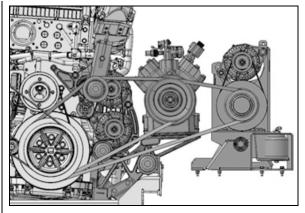
FIGURE 23: THREE ALTERNATOR BELT ARRANGEMENT
