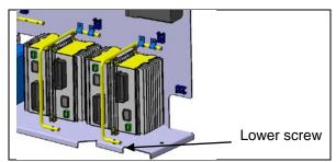
FIGURE 26: IO-B MODULE REMOVAL
