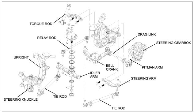
FIGURE 9: IFS STEERING LINKAGE OVERVIEW
