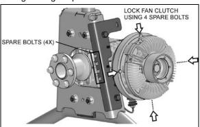
FIGURE 25: MECHANICAL LOCKING
