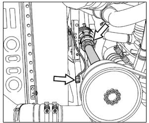
FIGURE 16: DISCONNECTING FAN DRIVE SHAFT
