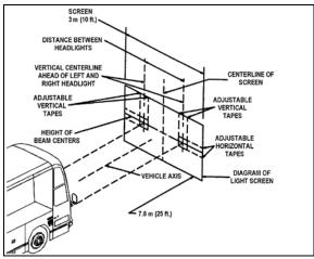
FIGURE 33: ALIGNMENT OF HEADLIGHT AIMING
