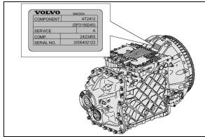
FIGURE 3: I-SHIFT TRANSMISSION
