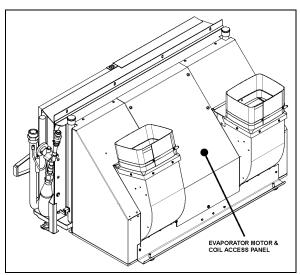
FIGURE 12: EVAPORATOR COIL ACCESS PANEL (TYPICAL) 22309
