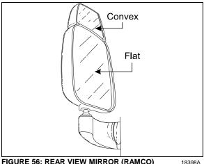
FIGURE 56: REAR VIEW MIRROR (RAMCO)
