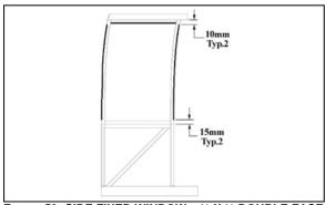
FIGURE 53: SIDE FIXED WINDOW – ¼ X ½ DOUBLE FACE ADHESIVE TAPE INSTALLATION
