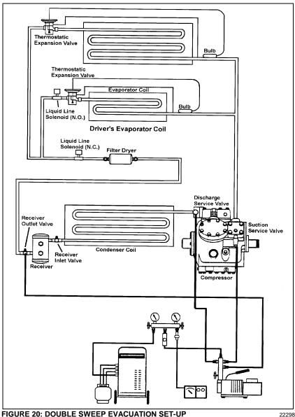
FIGURE 20: DOUBLE SWEEP EVACUATION SET-UP
