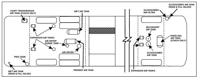
FIGURE 51: IFS AIR TANKS LOCATION
