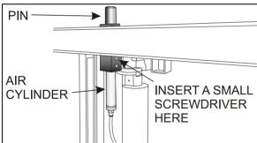
FIGURE 8: SECURITY PIN AIR CYLINDER REMOVAL
