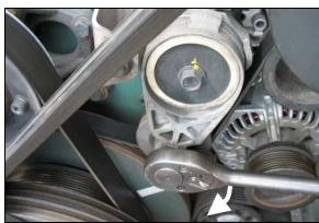
FIGURE 27: 1/2" SOCKET DRIVE WRENCH
