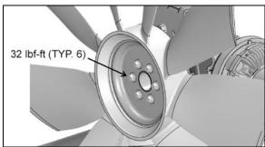
FIGURE 26: RADIATOR FAN MOUNTING BOLTS
