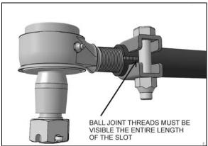
FIGURE 20: ADEQUATE CLAMPING CONDITION
