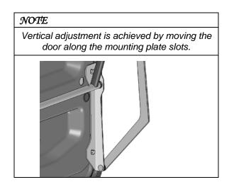
3. Center door in the opening using the retaining rings.
