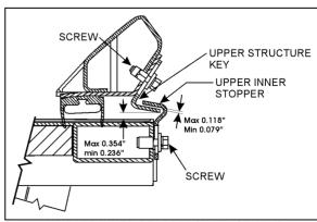
FIGURE 4: UPPER INNER STOPPERS ADJUSTMENT
