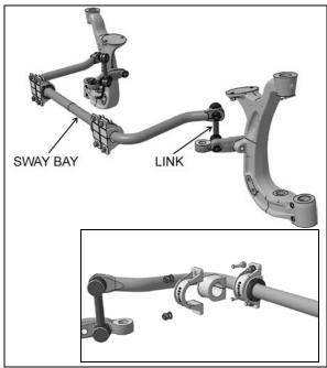
FIGURE 34: SWAY BAR (INDEPENDENT FRONT SUSPENSION)16138\_C
