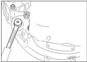
FIGURE 11: VOLVO ENGINE CRANKING POSITION
