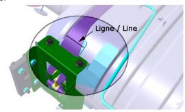
Mark, with a vertical line the central position of the lower and upper clamps with regard to the embossing located at the bottom and at the top of the catalytic converter.
