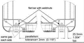
FIGURE 24: RAIL POSITIONING
