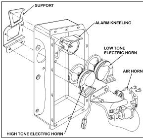
FIGURE 29: ELECTRIC & AIR HORN INSTALLATION 23420
