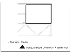
FIGURE 56: FACE FIXED WINDOW INSTALLATION – SIKA TACK+BOOSTER
