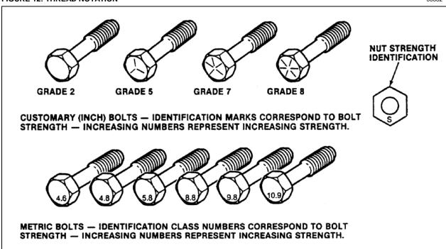
FIGURE 13: BOLT STRENGTH MARKINGS
