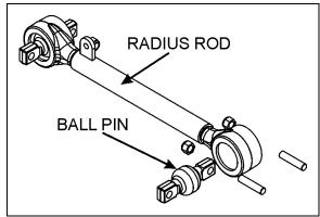
FIGURE 4: TYPICAL RADIUS ROD SETUP
