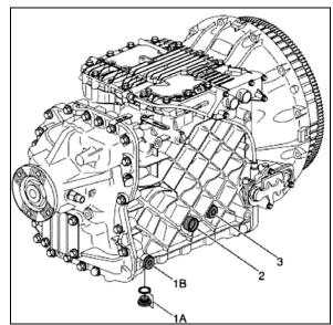
FIGURE 12: I-SHIFT TRANSMISSION OIL CHANGE
