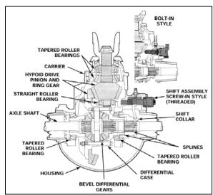
FIGURE 3: DRIVER-CONTROLLED DIFFERENTIAL LOCK
