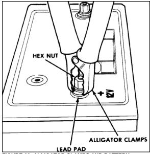
FIGURE 20: ALLIGATOR CLAMPS AND BATTERY 06065
