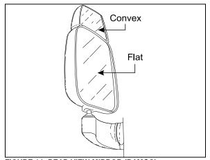
FIGURE 14: REAR VIEW MIRROR (RAMCO)
