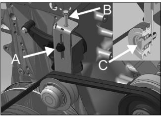
Figure 21: Tensioner on standard belt ARRANGEMENT
