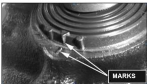
FIGURE 12: STEERING GEARBOX INPUT SHAFT MARKS
