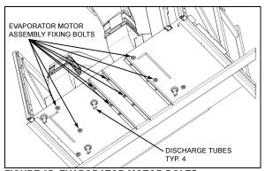
FIGURE 25: EVAPORATOR MOTOR BOLTS
