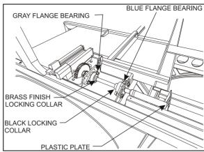
FIGURE 13: MECHANICAL COMPONENTS (TYPICAL)
