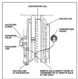
FIGURE 33: SUPERHEAT ADJUSTMENT INSTALLATION22046
