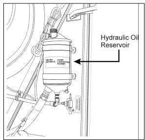
FIGURE 24: HYDRAULIC FLUID RESERVOIR LOCATION
