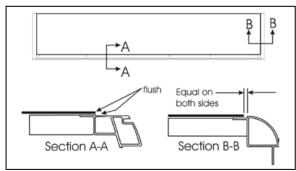
FIGURE 48: TOP PANEL INSTALLATION
