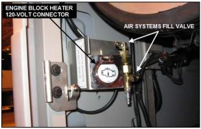
FIGURE 53: REAR VALVE LOCATION
