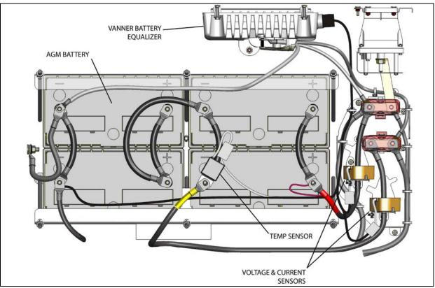
FIGURE 22: PRIME ELECTRICAL COMPONENTS
