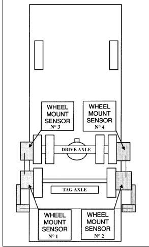
FIGURE 8: TAG AXLE ALIGNMENT
