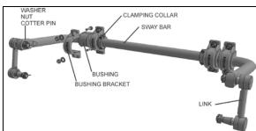
FIGURE 7: I-BEAM FRONT AXLE SWAY BAR
