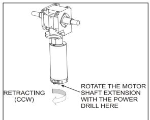
FIGURE 92: SLIDE-OUT MOTOR ROTATION
