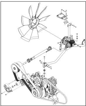
FIGURE 21: COOLING FAN DRIVE MECHANISM
