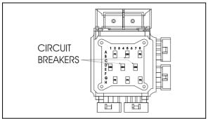
FIGURE 36: VEC CIRCUIT BREAKERS & FUSES
