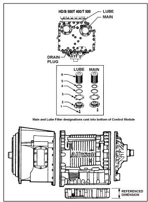
FIGURE 7: DRAIN PLUG AND FILTERS
