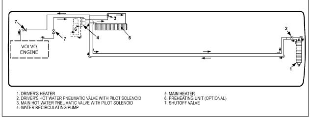
FIGURE 39: CENTRAL HEATING SYSTEM COMPONENTS
