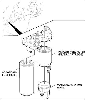
FIGURE 5: FUEL FILTERS WITH VOLVO D13 ENGINE
