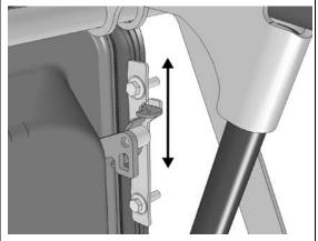
16. Open baggage compartment door and adjust using the cylinder mounting block.
