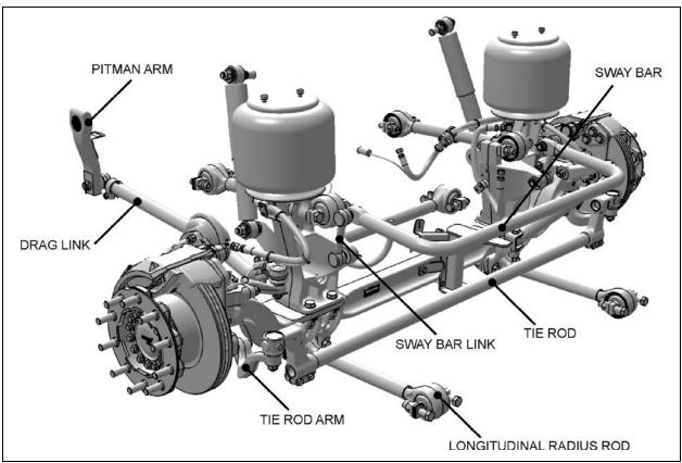
FIGURE 1: FRONT AXLE ASSEMBLY
