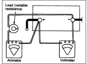
FIGURE 19: LOAD TEST
