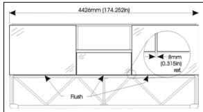
FIGURE 59: FACE FIXED WINDOW INSTALLATION
