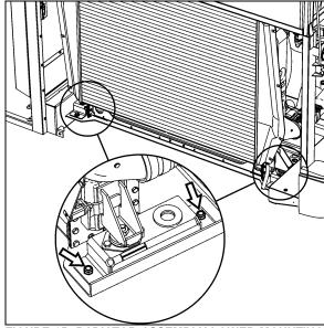
FIGURE 15: RADIATOR ASSEMBLY LOWER MOUNTING FASTENERS
