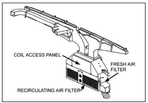
FIGURE 11: DRIVER'S HVAC UNIT COIL ACCESS PANEL
