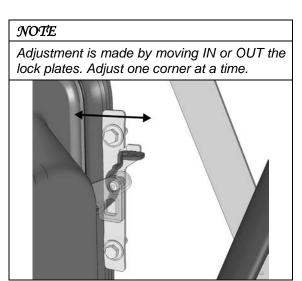
15. Check handle adjustment. Handle must remain tight against its plastic housing.
