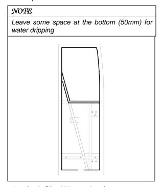
Apply Sika 255 onto door frame structure.
