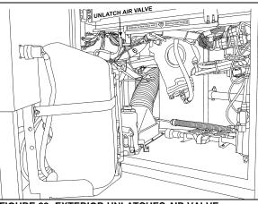
FIGURE 22: EXTERIOR UNLATCHES AIR VALVE 1
