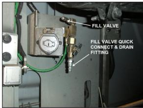
FIGURE 3: REAR VALVE LOCATION (TYPICAL)
