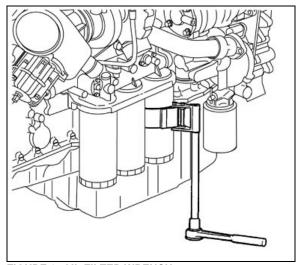
FIGURE 6: OIL FILTER WRENCH
