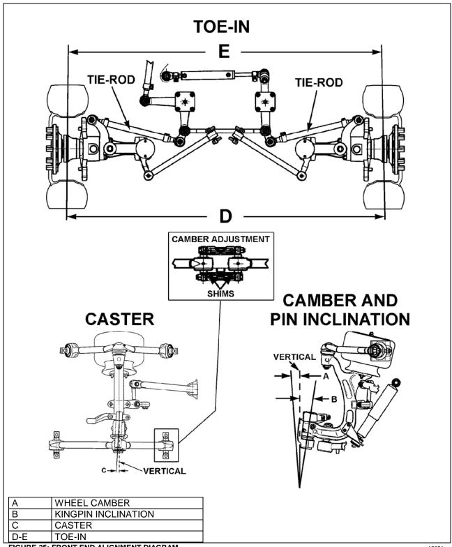
FIGURE 25: FRONT END ALIGNMENT DIAGRAM
