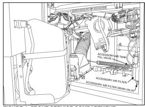
**FIGURE 4: FRONT SERVICE COMPARTMENT**
