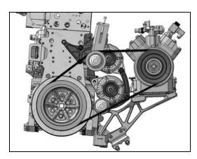
FIGURE 22: STANDARD BELT ARRANGEMENT
