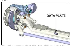
FIGURE 6: I-BEAM AXLE TYPICAL SERIAL & MODEL NUMBERS 00008
