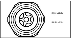
FIGURE 13: SIGHT GLASS FOR CHECKING OIL LEVEL
