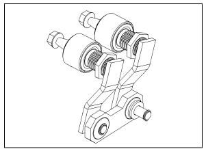
FIGURE 38: DRIVING MECHANISM (DRIVER SIDE) 23284
