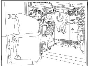
FIGURE 11: FRONT BUMPER RELEASE HANDLE
