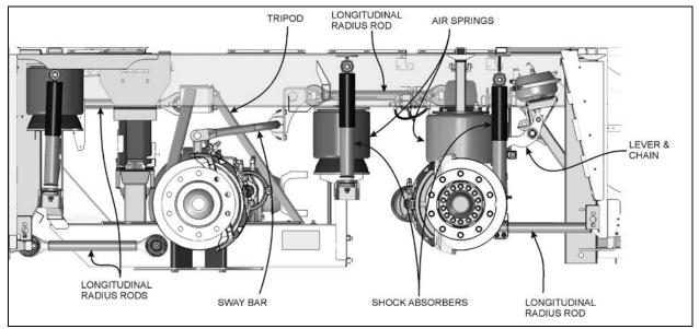
FIGURE 38: REAR SUSPENSION COMPONENTS
