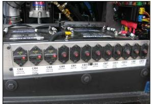
FIGURE 10: REAR ELECTRICAL JUNCTION PANEL
