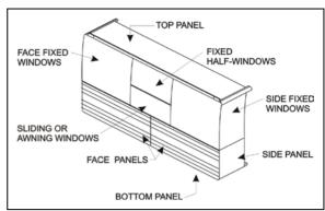
FIGURE 40: SLIDE-OUT PANELS AND WINDOWS
