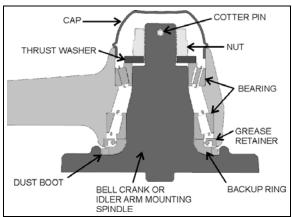
FIGURE 15: BELL CRANK OR IDLER ARM HUB
