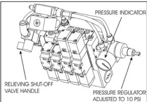
FIGURE 91: INFLATABLE SEAL RELIEVING SHUT-OFF VALVE
