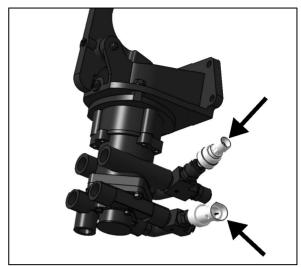
FIGURE 15: PRESSURE SWITCHES
