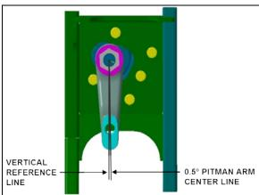
FIGURE 22: IFS PITMAN ARM ALIGNMENT
