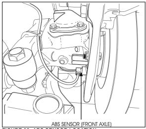
FIGURE 32: ABS SENSOR LOCATION
