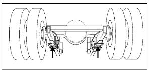
FIGURE 6: JACKING POINTS ON DRIVE AXLE
