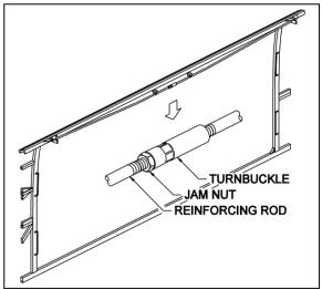
FIGURE 9: FRONT SLIDE-OUT ROOF REINFORCING ROD
