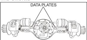
FIGURE 4: DATA PLATE LOCATION WITH MODEL NO., SERIAL NO. AND RATIO 00007
