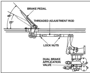
FIGURE 14: BRAKE PEDAL ADJUSTMENT
