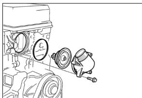
FIGURE 5: VOLVO D13 THERMOSTAT HOUSING
