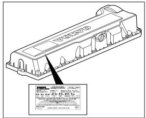
FIGURE 1: VOLVO D13 ENGINE DATA PLATE
