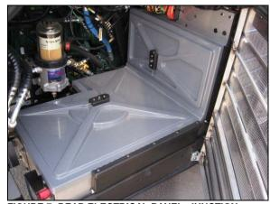
FIGURE 7: REAR ELECTRICAL PANEL, JUNCTION PANEL & BATTERY COMPARTMENT
