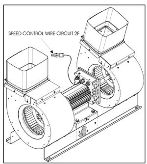
FIGURE 26: EVAPORATOR MOTOR ASSEMBLY
