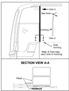
Position and fix horizontal molding (gutter). Lean gutter against vertical molding. Position gutter just above Sika finishing joint.
