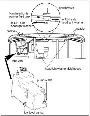
FIGURE 30: HEADLIGHTS CLEANING SYSTEM
