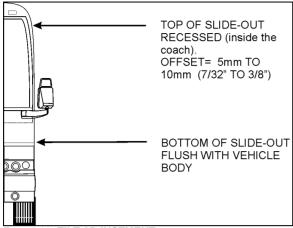
FIGURE 23: TILT ADJUSTMENT
