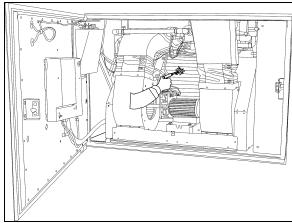
FIGURE 13: EVAPORATOR COIL CLEANING
