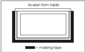
FIGURE 63: MASKING TAPE APPLICATION
