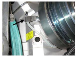
During the 250 hour run-in period of the shaft seal, an increased oil leak rate may occur.
