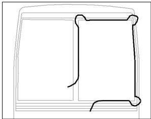
FIGURE 15: WINDSHIELD INSTALLATION USING ROPE
