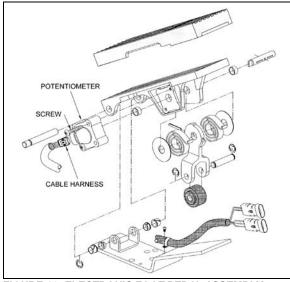
FIGURE 16: ELECTRONIC FOOT PEDAL ASSEMBLY 03035
