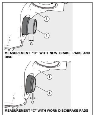
FIGURE 23: BRAKE PAD WEAR CHECK ON DRIVE AXLE
