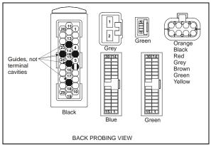
FIGURE 3: MULTIPLEX MODULE CONNECTORS PIN-OUT 06624
