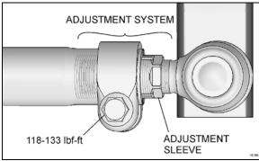
FIGURE 22: DRAG LINK ADJUSTMENT SYSTEM
