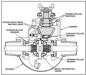
FIGURE 2: DIFFERENTIAL ASSEMBLY
