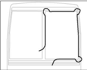
FIGURE 57: WINDSHIELD INSTALLATION USING ROPE
