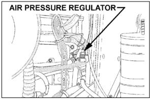
FIGURE 9: AIR PRESSURE REGULATOR (TYPICAL) 07037
