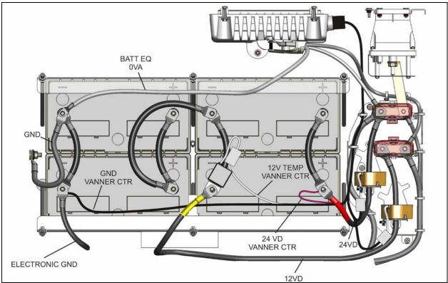
FIGURE 18: AGM BATTERY CONNECTIONS
