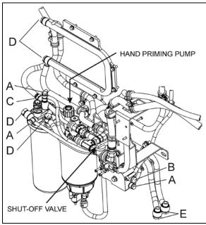
FIGURE 2: MANUAL SHUT-OFF VALVE (VOLVO D13 ENGINE) 03088
