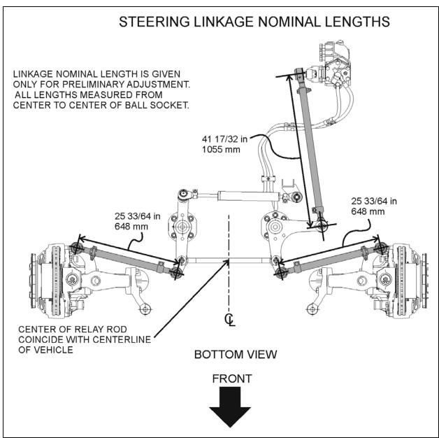
FIGURE 18: STEERING LINKAGE NOMINAL LENGTHS
