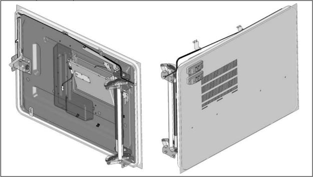
FIGURE 40: EVAPORATOR DOOR (ALUMINUM)
