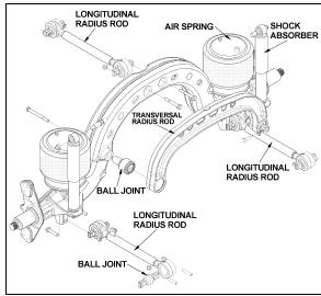
FIGURE 40: TAG AXLE SUSPENSION
