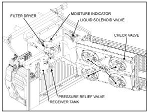
FIGURE 29: A/C CONDENSER COMPARTMENT
