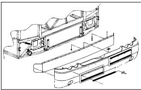
FIGURE 13: FRONT BUMPER REMOVAL
