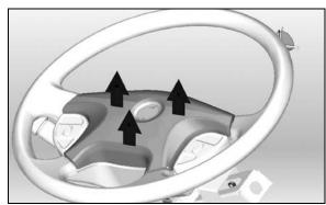
FIGURE 10: REMOVING THE HORN PAD
