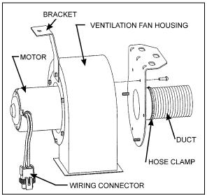
FIGURE 24: VENTILATION FAN INSTALLATION
