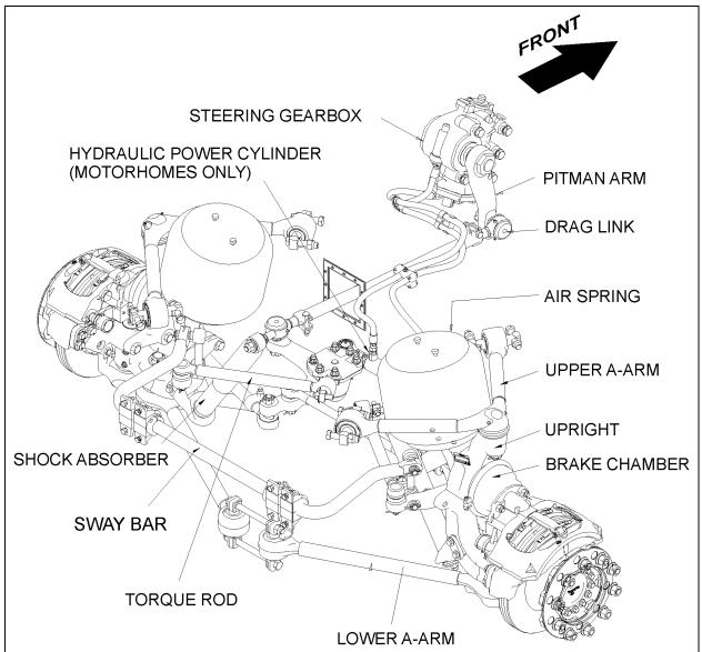
FIGURE 8: INDEPENDENT FRONT SUSPENSION
