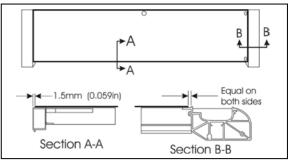
FIGURE 49: BOTTOM PANEL INSTALLATION
