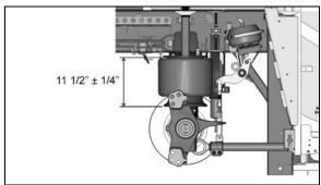
FIGURE 47: TAG AXLE AIR SPRING CLEARANCE
