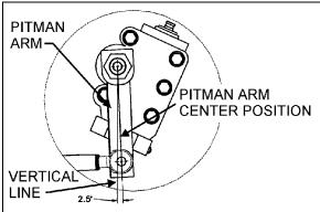
FIGURE 17: I-BEAM FRONT AXLE PITMAN ARM ADJUSTMENT 14037
