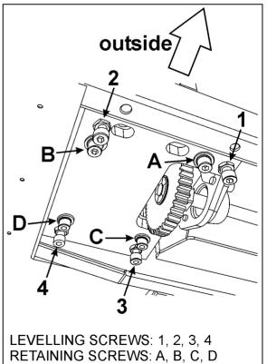
FIGURE 22: SLIDE-OUT LEVELING
