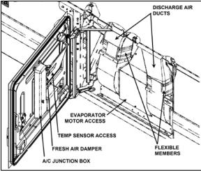
FIGURE 24: EVAPORATOR COMPARTMENT
