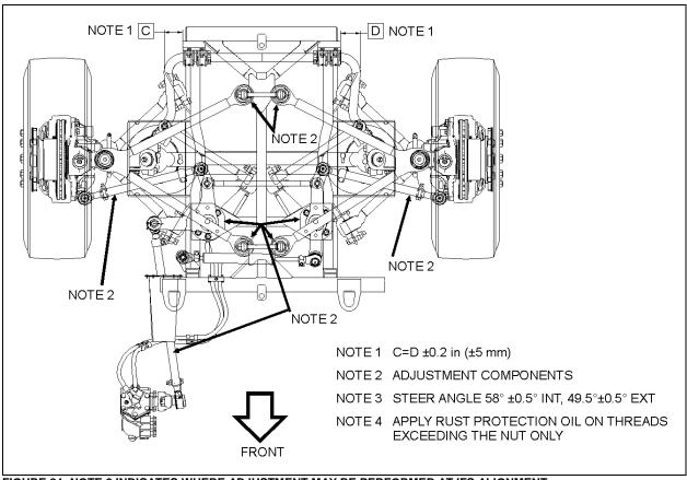
FIGURE 24: NOTE 2 INDICATES WHERE ADJUSTMENT MAY BE PERFORMED AT IFS ALIGNMENT
