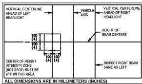
FIGURE 36: AIM INSPECTION LIMITS FOR UPPER-BEAM HEADLIGHTS
