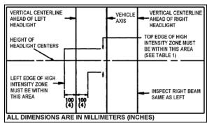
FIGURE 37: AIM INSPECTION LIMITS FOR LOWER-BEAM HEADLIGHTS 06506
