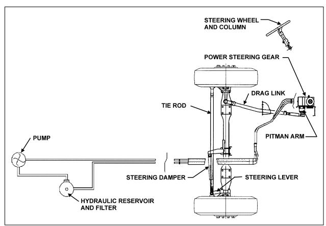
FIGURE 1: I-BEAM AXLE STEERING SYSTEM SETUP
