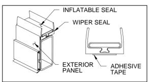
FIGURE 30: SEAL ASSEMBLY
