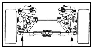
FIGURE 91: JACKING POINTS ON IND. SUSPENSION 16095
