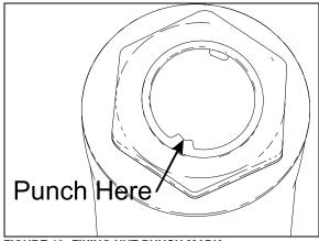
FIGURE 19: FIXING NUT PUNCH MARK
