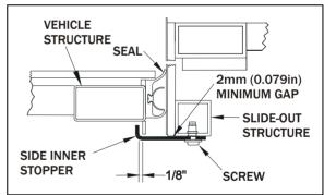
FIGURE 3: SIDE INNER STOPPER ADJUSTMENT
