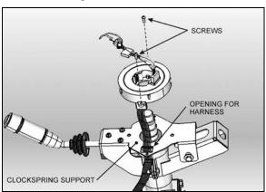
FIGURE 13: CLOCKSPRING INSTALLATION
