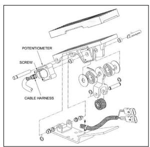
FIGURE 13: ELECTRONIC FOOT PEDAL ASSEMBLY 3035
