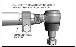
FIGURE 31: ADEQUATE CLAMPING CONDITION
