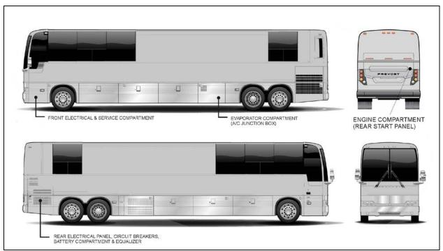
FIGURE 5: ELECTRICAL COMPARTMENTS (X3-45 VIP)
