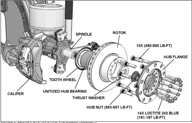
FIGURE 8: FRONT & TAG AXLE HUB AND ROTOR ASSEMBLY
