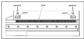
FIGURE 39: MAGNETS ON SLIDE-OUT UNDERBODY
