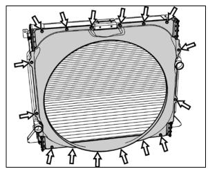
FIGURE 20: REMOVING FAN SHROUD FROM RADIATOR
