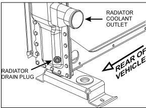
FIGURE 9: RADIATOR DRAIN PLUG
