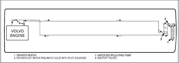
FIGURE 54: SMALL HEATING SYSTEM COMPONENTS
