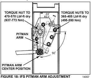
7. You must use a puller to remove pitman arm.
