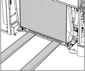
FIGURE 17: POSITIONING FORKLIFT
