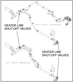
FIGURE 42: HEATER LINE SHUT-OFF VALVES
