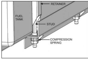
FIGURE 13: FUEL TANK RETENTION
