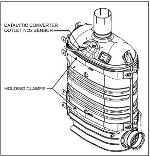
FIGURE 5: CATALYTIC CONVERTER
