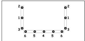
FIGURE 67: CORRECT TIGHTENING SEQUENCE
