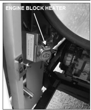
FIGURE 30: ELECTRIC HEATER CONNECTION
