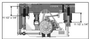
FIGURE 46: DRIVE AXLE AIR SPRING CLEARANCE 16195
