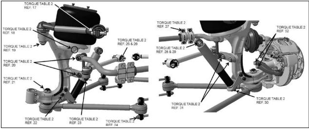
FIGURE 10: IFS - SUSPENSION COMPONENTS
