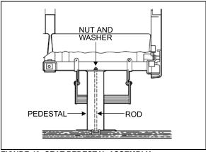
FIGURE 48: SEAT PEDESTAL ASSEMBLY
