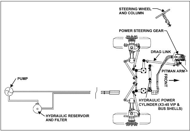
FIGURE 2: IFS STEERING SYSTEM SETUP
