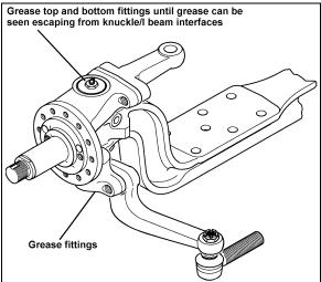
FIGURE 2: FRONT AXLE GREASING POINTS
