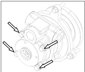
FIGURE 7: POWER STEERING PUMP REMOVAL
