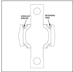
FIGURE 28: LOWER A-ARM BAR PIN BUSHING 16047
