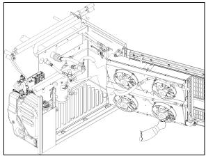
FIGURE 14: CONDENSER COMPARTMENT
