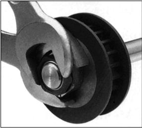
FIGURE 14: KEYLESS BUSHING TIGHTENING
