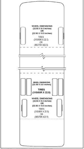
FIGURE 2: WHEEL ARRANGEMENT
