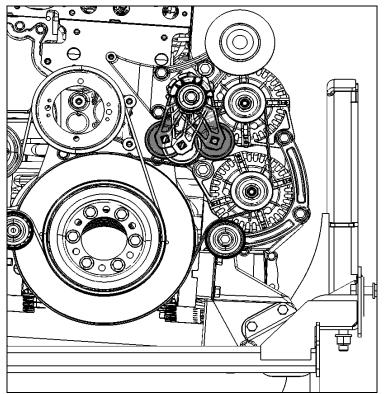
FIGURE 28: ALTERNATOR DRIVE BELT
