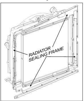
FIGURE 11: RADIATOR SEALING FRAME
