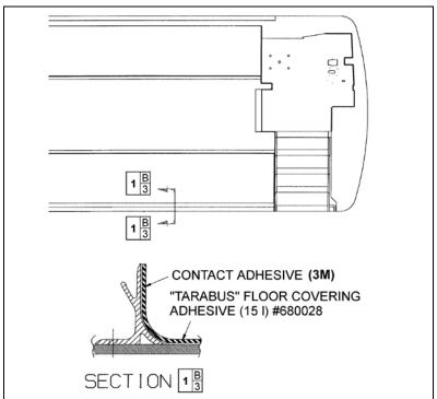
FIGURE 49: TARABUS FLOOR COVERING ADHESIVE APPLICATION
