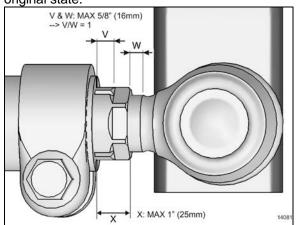
FIGURE 23: DRAG LINK ADJUSTMENT SYSTEM
