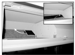
FIGURE 18: OVERHEAD COMPARTMENT FAN AIR FILTER
