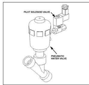
FIGURE 44: DRIVER'S HOT WATER PNEUMATIC VALVE ASSEMBLY
