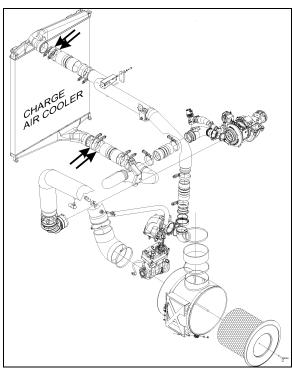
FIGURE 13: CHARGE AIR COOLER HOSE CLAMPS
