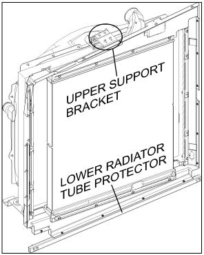
FIGURE 14: UPPER SUPPORT BRACKET & TUBE PROTECTOR
