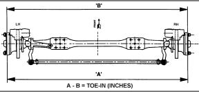
FIGURE 5: TOE-IN MEASUREMENT
