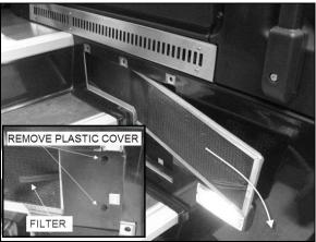
FIGURE 16: REMOVING DRIVER'S SECTION AIR FILTERS
