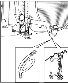
FIGURE 7: EXTRACTING COOLANT
