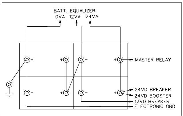
FIGURE 17: STANDARD BATTERY CONNECTIONS
