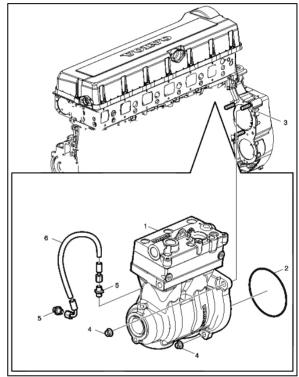
FIGURE 10: AIR COMPRESSOR LOCATION 03
