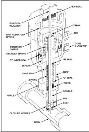
FIGURE 45: DRIVER'S PNEUMATIC WATER VALVE
