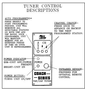
FIGURE 14: TUNER CONTROLS DESCRIPTION
