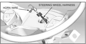
FIGURE 11: STEERING HARNESS & HORN WIRE
