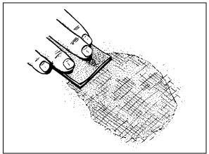
FIGURE 7: FIBERGLASS REPAIR
