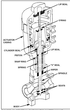
FIGURE 47: CENTRAL PNEUMATIC WATER VALVE 22330
