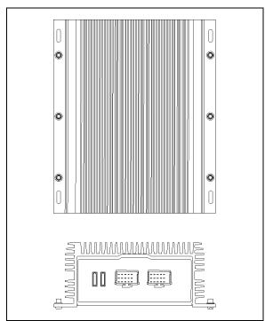
FIGURE 8: MULTICHANNEL POWER AMPLIFIER
