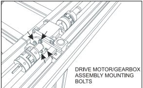
FIGURE 18: DRIVE MOTOR/GEARBOX ASSEMBLY MOUNTING BOLTS
