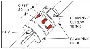
FIGURE 20: JAW COUPLING
