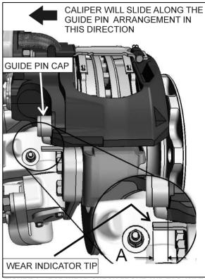
FIGURE 24: PAD WEAR CHECK FRONT AND TAG AXLE
