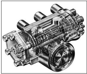
FIGURE 3: POWER STEERING GEAR
