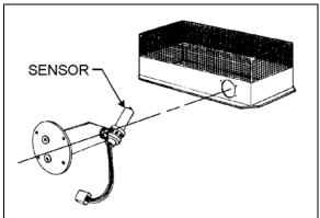
FIGURE 7: THERMISTOR SENSOR
