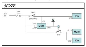
JB6 is a wake-up pin. JA15 output remains active for 5 minutes after JB6 is inactive.
