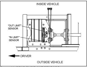
FIGURE 38: REAR SLIDE-OUT SENSORS
