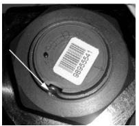
FIGURE 14: FIXING NUT PUNCH MARK
