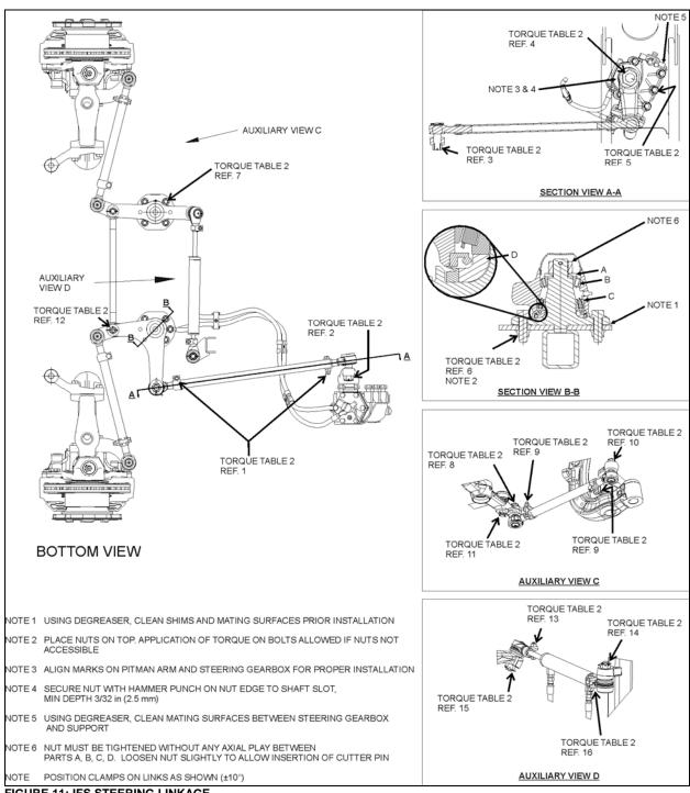
FIGURE 11: IFS STEERING LINKAGE
