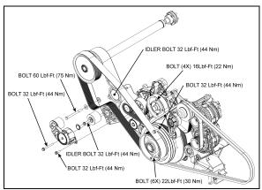
FIGURE 23: TIGHTENING SPECIFICATION (VOLVO D13 ENGINE)
