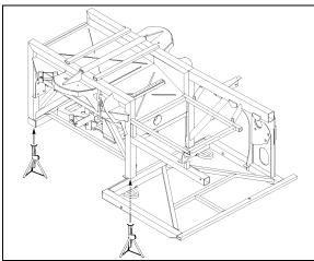
FIGURE 89: FRONT END JACKING POINTS
