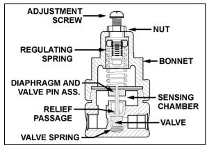
FIGURE 9: AIR PRESSURE REGULATING VALVE 12141A
