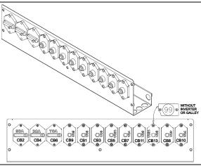
FIGURE 2: REAR ELECTRICAL JUNCTION PANEL 06621
