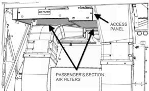
FIGURE 17: PASSENGERS' SECTION AIR FILTER 22375
