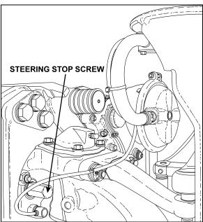
FIGURE 16: STEERING STOP SCREW ON I-BEAM AXLE
