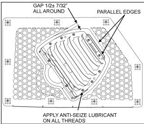
FIGURE 7: DIFFUSER POSITION ADJUSTMENT 04015\_1
