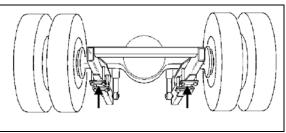
FIGURE 93: JACKING POINTS ON DRIVE AXLE OEH3B762
