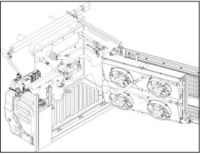
FIGURE 9: CONDENSER COMPARTMENT
