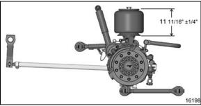
FIGURE 48: FRONT I-BEAM AXLE AIR SPRING CLEARANCE
