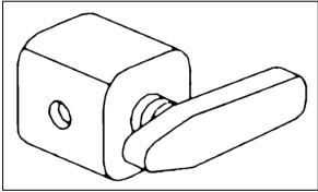
FIGURE 21: THREE-WAY VALVE
