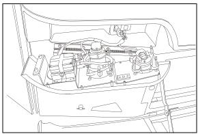
FIGURE 32: OPENING HEADLIGHT ASSEMBLY 0654
