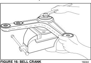
11. Unscrew nut until bell crank or idler arm starts to turn with the application of 1 to 3 lbf
