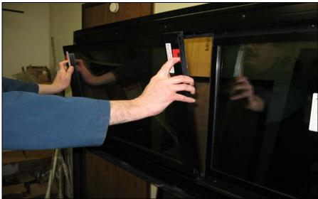
FIGURE 64: REMOVING THE SASH
