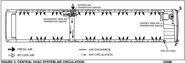
FIGURE 3: CENTRAL HVAC SYSTEM AIR CIRCULATION
