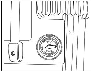
FIGURE 21: INTERIOR UNLATCH AIR VALVE
