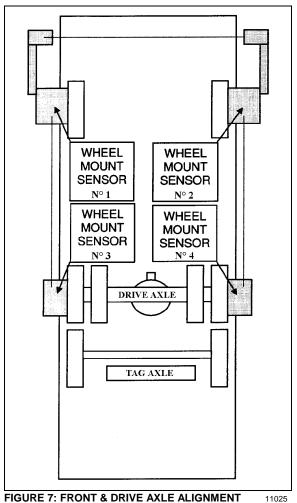
FIGURE 7: FRONT & DRIVE AXLE ALIGNMENT
