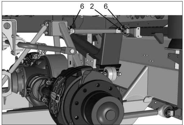
FIGURE 60: TORQUE SPECIFICATIONS - DRIVE AXLE, TOP
