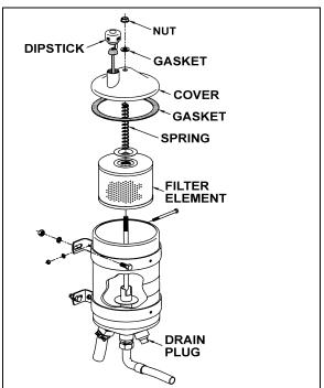
FIGURE 25: POWER STEERING FLUID RESERVOIR14018A
