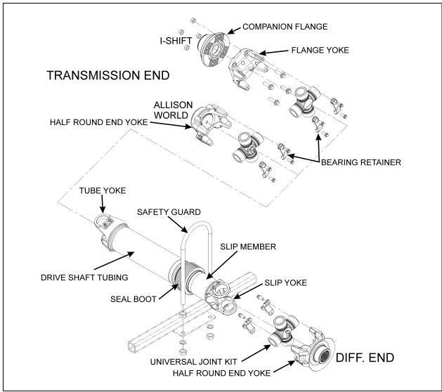
FIGURE 1: PROPELLER SHAFT ASSEMBLY (TYPICAL)
