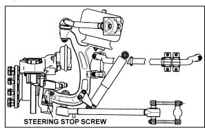
FIGURE 15: STEERING STOP SCREW ON IFS
