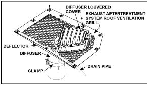
FIGURE 6: DIFFUSER ASSEMBLY
