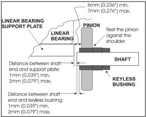
FIGURE 11: PINION AND KEYLESS BUSHING POSITIONING
