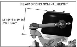
FIGURE 36: TYPICAL AIR SPRING CLEARANCE
