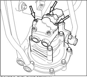
FIGURE 7: FUEL PUMP REMOVAL
