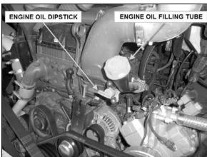
FIGURE 8: ENGINE OIL FILLING TUBE
