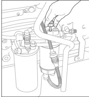
FIGURE 6: HAND PRIMING PUMP
