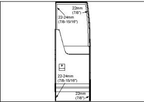
FIGURE 25: SEAL COMPRESSION ADJUSTMENT
