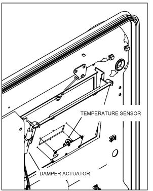
FIGURE 2: PASSENGERS' AREA FRESH AIR DAMPER 22302\_A
