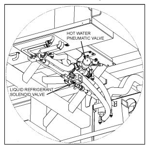
FIGURE 40: CEILING OF THE SPARE WHEEL COMPARTMENT
