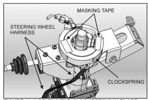
FIGURE 12: LOCKING THE CLOCKSPRING IN PLACE
