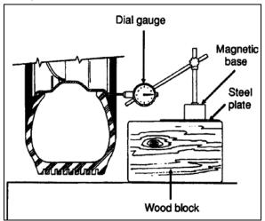
FIGURE 4: DIAL GAUGE INSTALLATION
