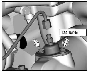
FIGURE 9: AFTERTREATMENT FUEL INJECTOR
