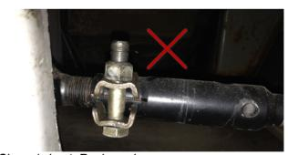
Clamp is bent. Replace clamp.
