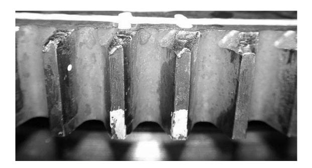
Please refer to the above photos and please replace the ring gear which has similar level of damage as these. See the next page for the method to measure the depth of the damage.
