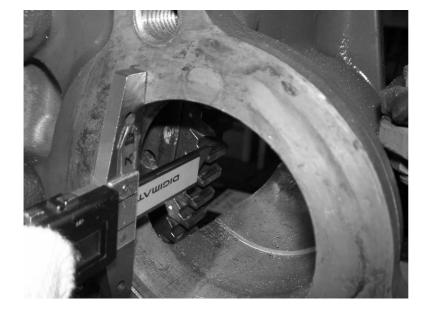
Dimension between the mounting surface and the damage depth portion of ring gear
