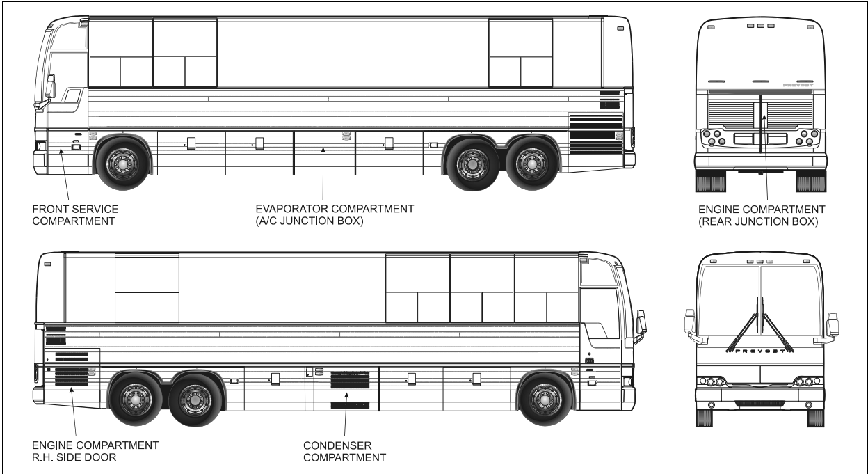
FIGURE 12: ELECTRICAL COMPARTMENTS (XL2-40 BUS SHELLS)
