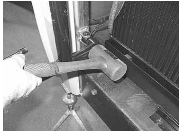
FIGURE 64: PANTOGRAPH ARM ADJUSTMENT
