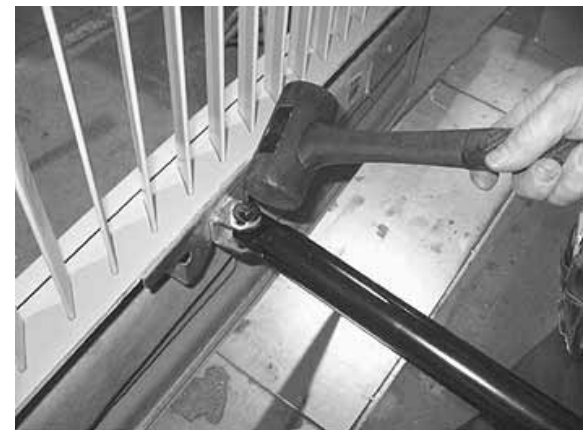
FIGURE 65: DOOR LATERAL ADJUSTMENT
