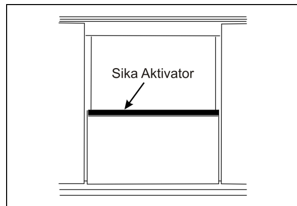
FIGURE 72 : SLIDING WINDOW - SIKa AKTIVATOR
