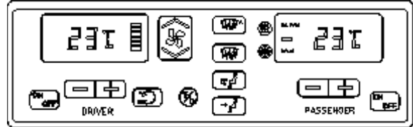
FIGURE 5: CENTRAL HVAC SYSTEM CONTROL UNIT 22296
