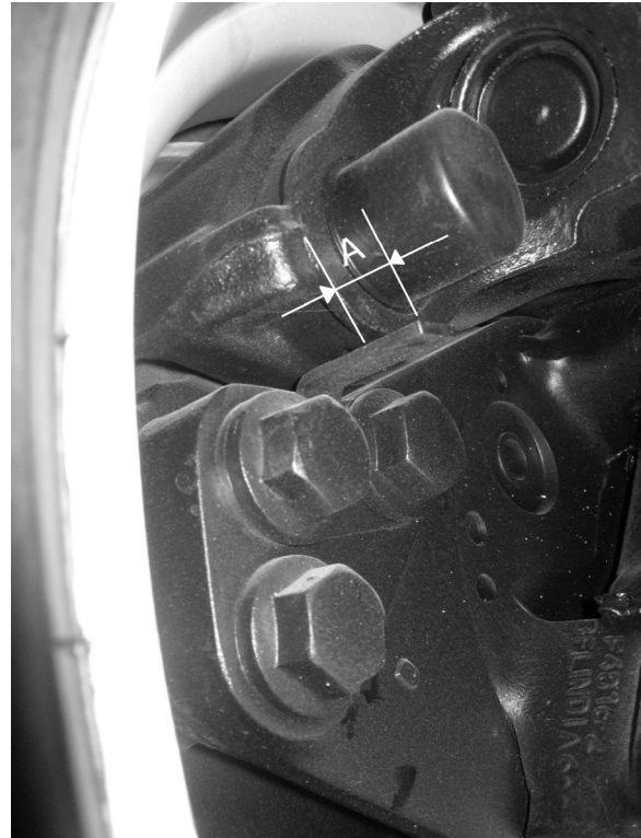
FIGURE 25: BRAKE PAD WEAR INSPECTION 12119
