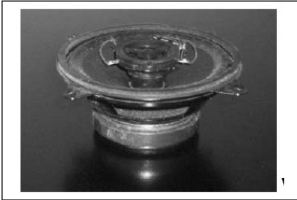
FIGURE 10: 10CM COAXIAL SPEAKER
