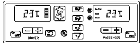
FIGURE 5: CENTRAL HVAC SYSTEM CONTROL UNIT 22296
