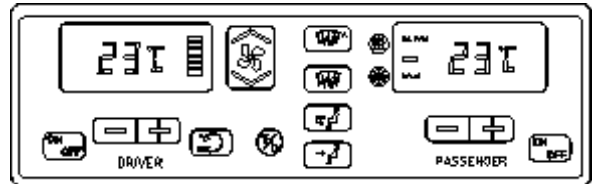
FIGURE 5: CENTRAL HVAC SYSTEM CONTROL UNIT 22296
