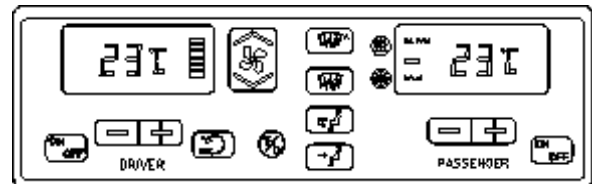
FIGURE 5: CENTRAL HVAC SYSTEM CONTROL UNIT 22296
