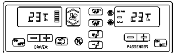
FIGURE 5: CENTRAL HVAC SYSTEM CONTROL MODULE
