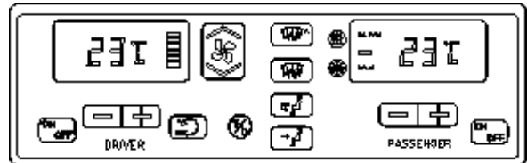
FIGURE 5: CENTRAL HVAC SYSTEM CONTROL MODULE
