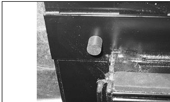
FIGURE 77 : SLIDING WINDOW - RUBBER BUSHING
