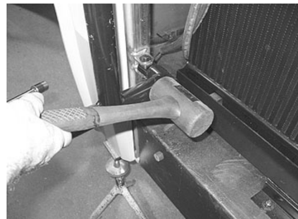
FIGURE 63: PANTOGRAPH ARM ADJUSTMENT
