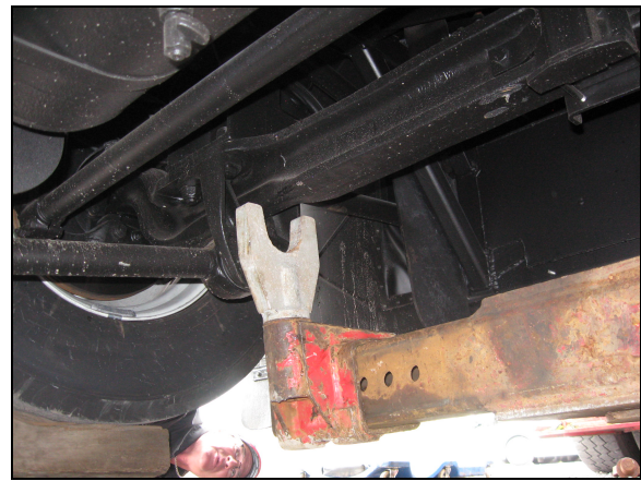
LIFTING FROM UNDER THE FRONT AXLE
