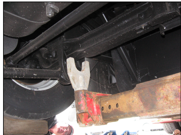
LIFTING FROM UNDER THE FRONT AXLE
