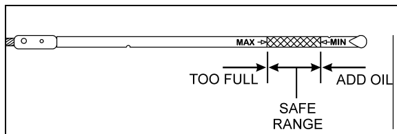
VOLVO D13 ENGINE OIL LEVEL DIPSTICK
