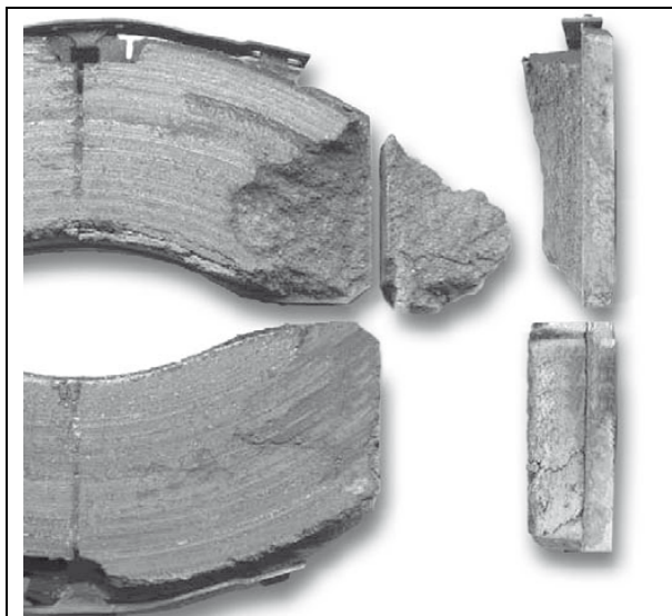
MAJOR BREAKOUTS ON THE SURFACE OF THE BRAKE PAD ARE NOT PERMITTED
