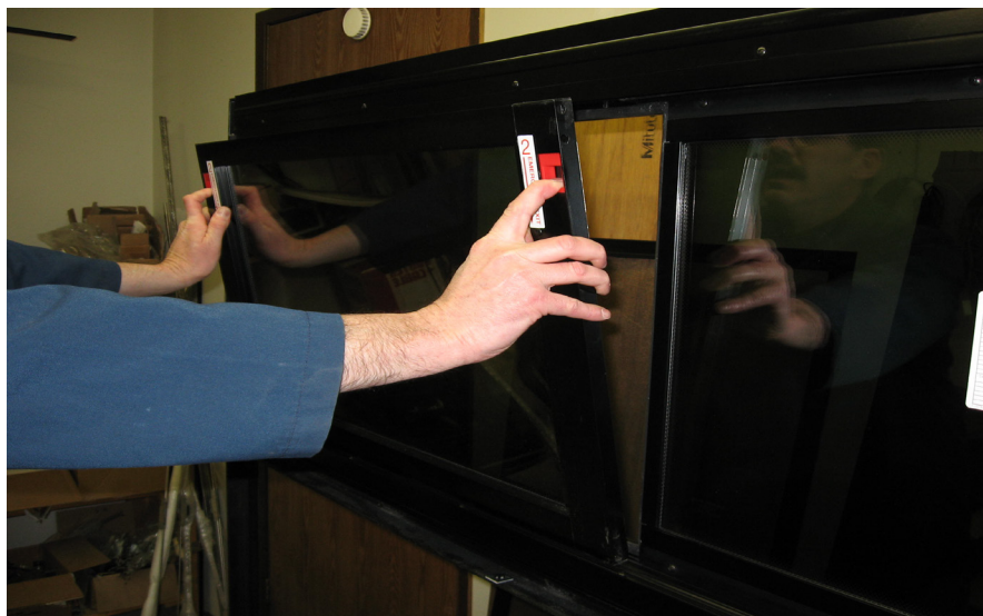
FIGURE 62: REMOVING THE SASH
