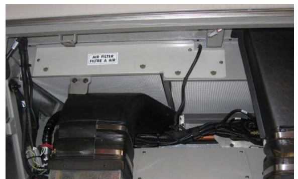
FIGURE 17: PASSENGERS' SECTION AIR FILTER
