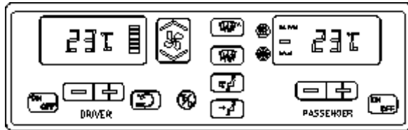
FIGURE 6: CENTRAL HVAC SYSTEM CONTROL UNIT
