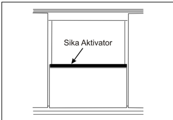
FIGURE 72 : SLIDING WINDOW - SIKA AKTIVATOR
