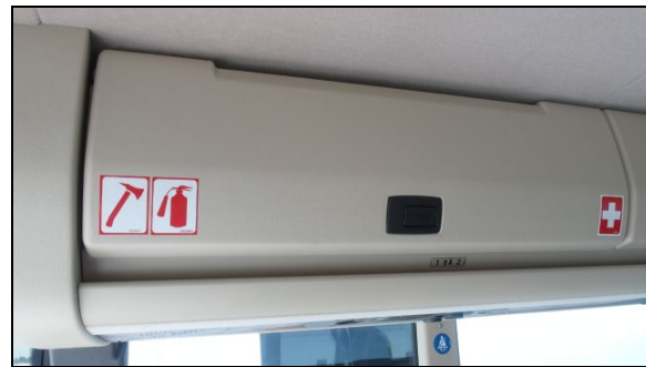
A DECAL INDICATES THAT A FIRE EXTINGUISHER (OPTION) IS LOCATED IN THIS OVERHEAD COMPARTMENT
