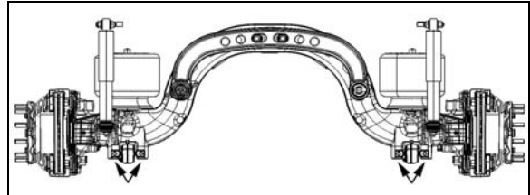
FIGURE 85: JACKING POINTS ON TAG AXLE
