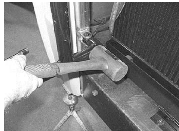
FIGURE 63: PANTOGRAPH ARM ADJUSTMENT
