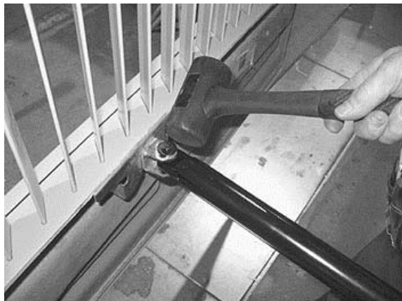
FIGURE 64: DOOR LATERAL ADJUSTMENT
