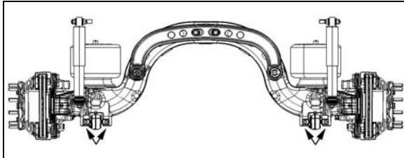
FIGURE 11: JACKING POINTS ON TAG AXLE 11023
