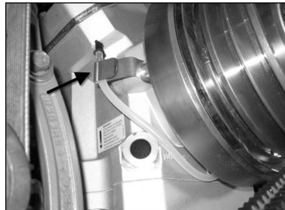
FIGURE 25: SHAFT SEAL OIL COLLECTING TUBE
