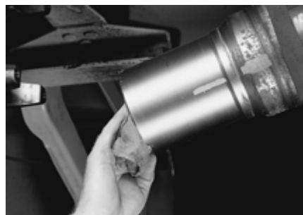
FIGURE 22: CLEAN GREASE FROM SPLINE SLEEVE
