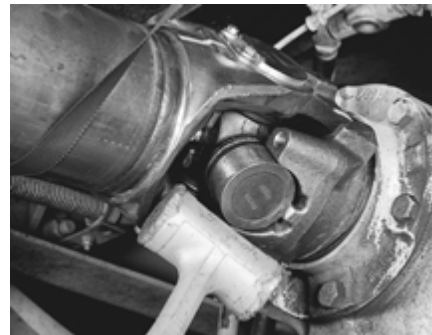
FIGURE 13: UNSEATING BEARING CUP ASSEMBLIES
