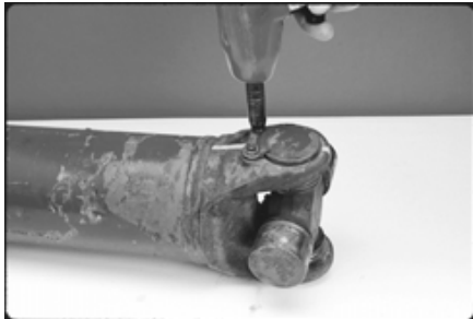
FIGURE 15: SPRING TAB BOLTS REMOVAL
