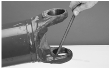
FIGURE 20: RAISED METAL OR FRETTING CAN BE REMOVED FROM YOKE CROSS HOLES WITH A FINE-TOOTHED FILE
