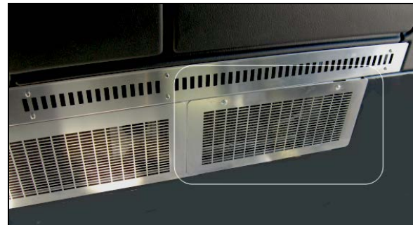
ACCESS TO DRIVER'S HVAC UNIT AIR FILTERS
