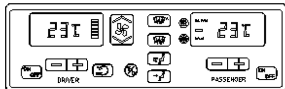
CENTRAL HVAC SYSTEM CONTROL MODULE
