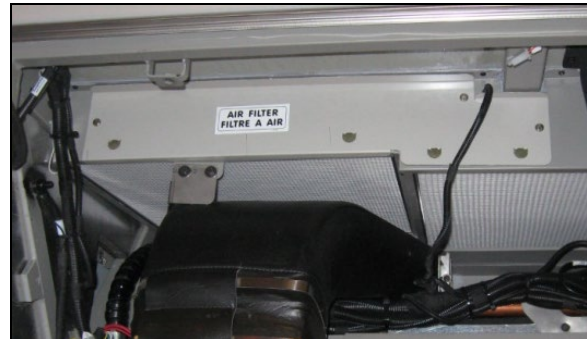
PASSENGERS AREA AIR FILTER REMOVAL
