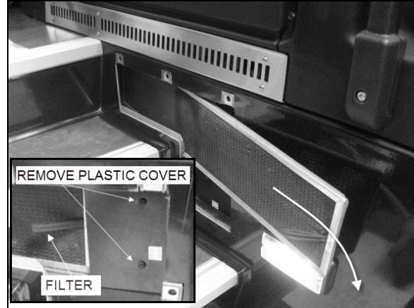
REMOVING DRIVER'S SECTION AIR FILTER
