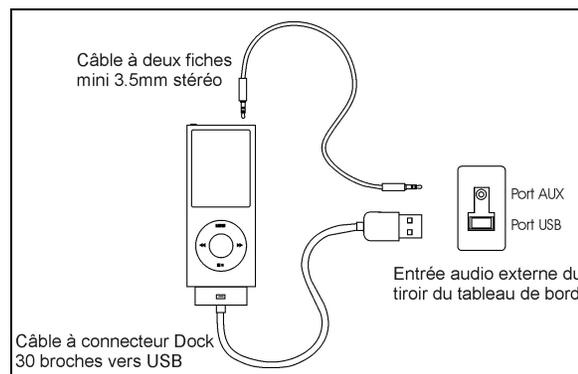
CONNEXION D'UN IPOD AVEC DEUX CÂBLES SÉPARÉS
