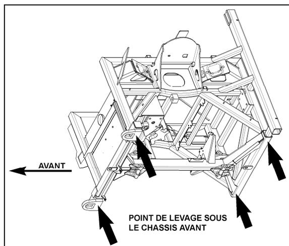
POINTS DE LEVAGE SOUS LE CHÂSSIS AVANT –
