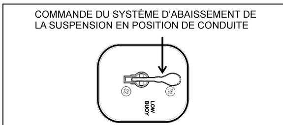
COMMANDE DU SYSTÈME D'ABAISSEMENT DE LA SUSPENSION
