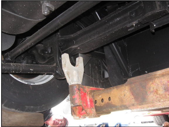
LIFTING FROM UNDER THE FRONT AXLE
