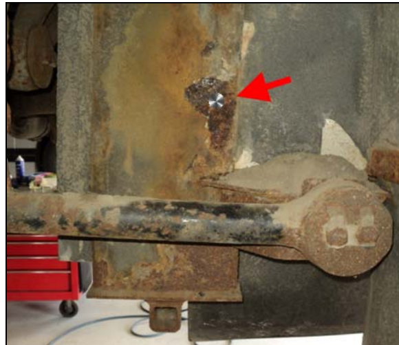
FIGURE 6: CLEANED SPOT ON STRUCTURAL MEMBER
