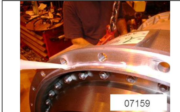
FIGURE 12: SILICONE APPLICATION TRANSMISSION HOUSING
