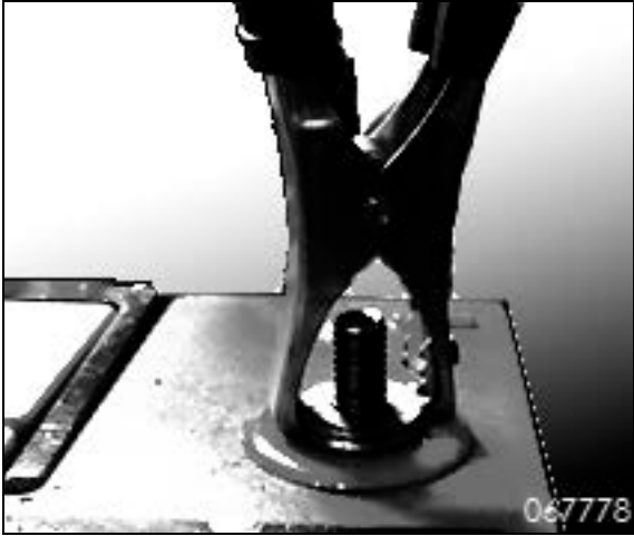
FIGURE 29 ALLIGATOR CLAMP POSITION- TYPICAL AGM BATTERY
