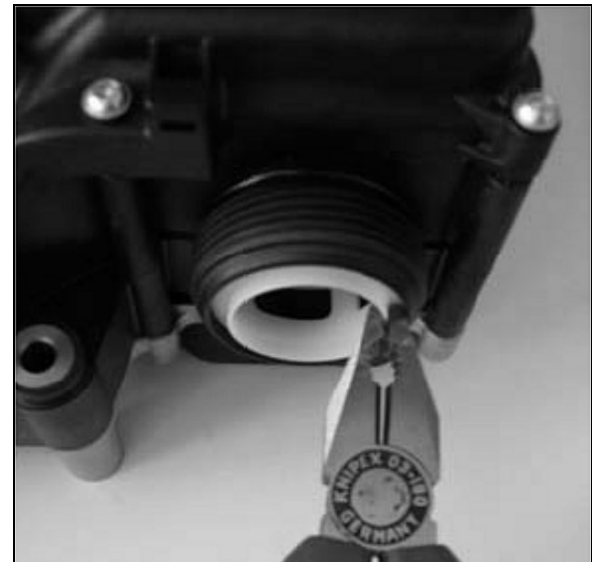
FIGURE 12 : PUMP ASSEMBLY FILTER ELEMENT
