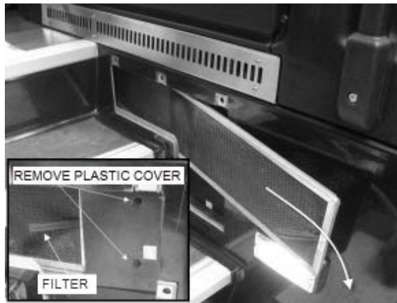
FIGURE 17: REMOVING DRIVER'S SECTION AIR FILTERS
