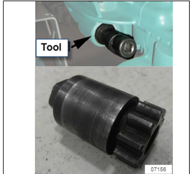
FIGURE 10: VOLVO ENGINE TURNING TOOL #88800014
