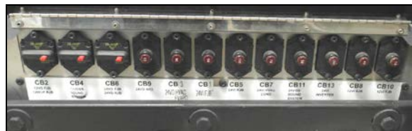
FIGURE 59: X3 SERIES REAR ELECTRICAL JUNCTION PANEL WITH CIRCUIT BREAKERS
