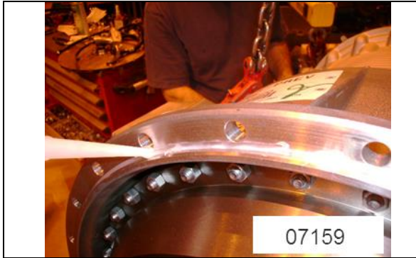
FIGURE 12: SILICONE APPLICATION TRANSMISSION HOUSING
