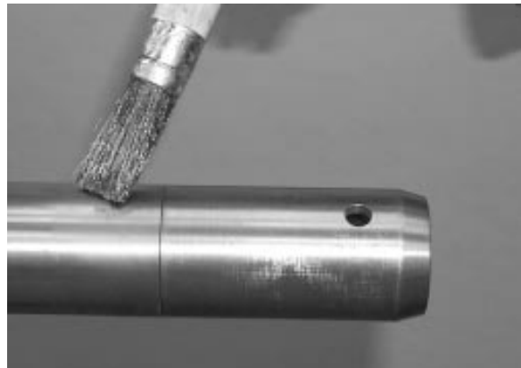
FIGURE 19: APPLY GLEITMO 805 GREASE
