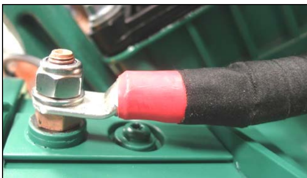
Figure 16: No exposed or broken copper strands.
