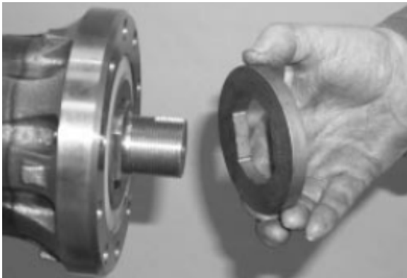
FIGURE 21: INSTALL THRUST WASHER
