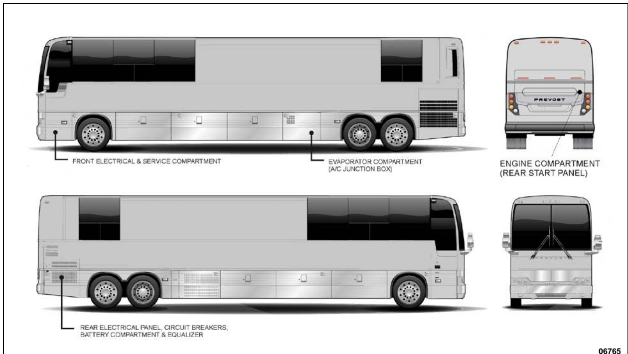
FIGURE 6: ELECTRICAL COMPARTMENTS (X3-45 VIP)
