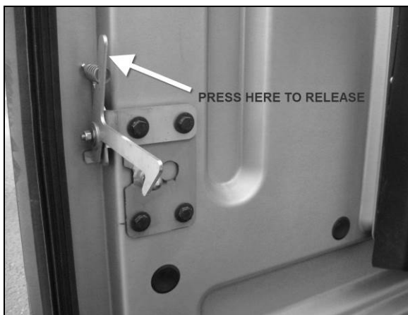
SECONDARY LOCK LEVER
