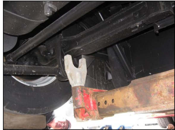
LIFTING FROM UNDER THE FRONT AXLE
