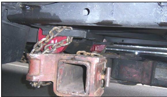
ADEQUATELY SECURE THE TOW EYES TO THE TOW TRUCK LIFTING ATTACHMENT WITH CHAINS
