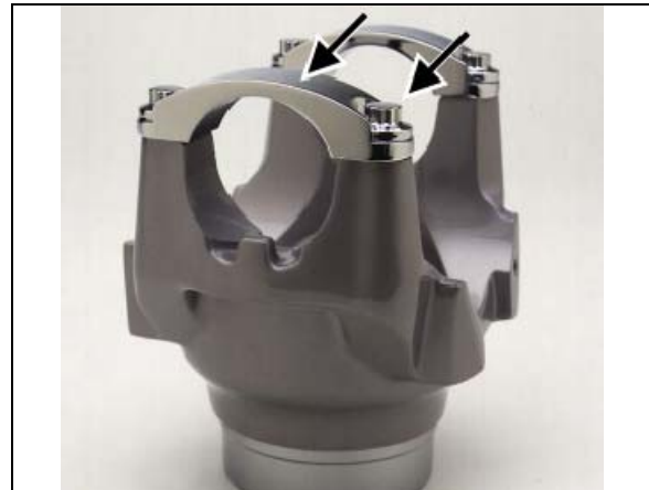
FIGURE 3: COLD FORMED BEARING RETAINER AND BOLTS AS USED ON PREVOST VEHICLES
