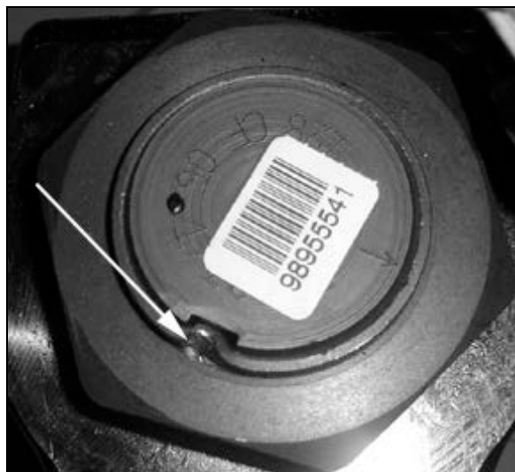
FIGURE 20: FIXING NUT PUNCH MARK 16098
