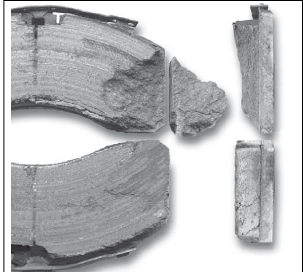
FIGURE 27: MAJOR BREAKOUTS ON THE SURFACE OF THE BRAKE PAD ARE NOT PERMITTED
