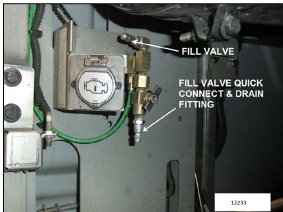
FIGURE 6: REAR VALVE LOCATION (typical)
