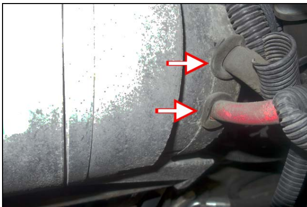
Figure 21: Bosch T1 alternator with the two required rubber grommets. Alternator cables connected to the alternator stud terminals must be protected against metal edges with rubber grommets.
