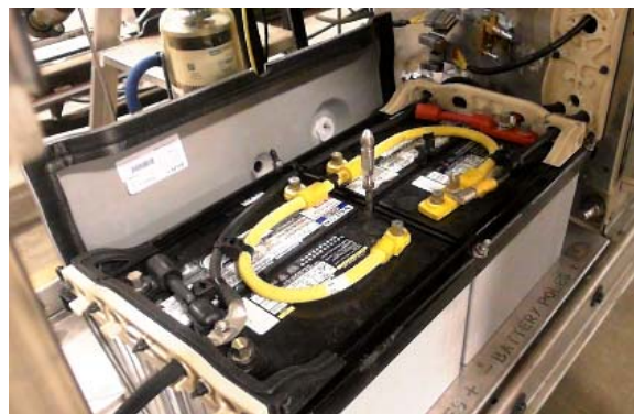
FIGURE 30: BATTERY BANK COVER REMOVED
