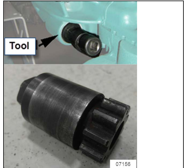
FIGURE 10: VOLVO ENGINE TURNING TOOL #88800014
