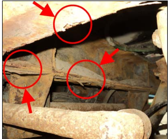
FIGURE 3: METAL FLAKING AND ACCUMULATED SAND
